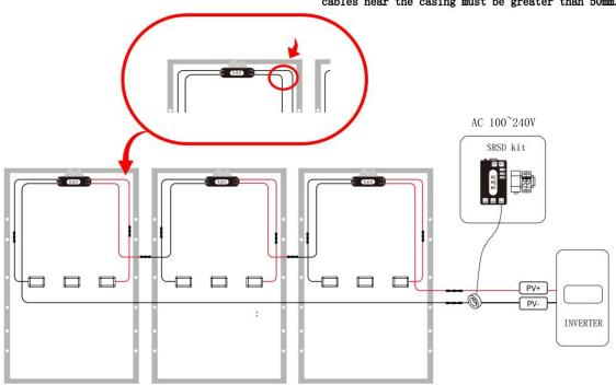
NOTE: When installing cables, the bending radius of the cables near the casing must be greater than 50mm.
