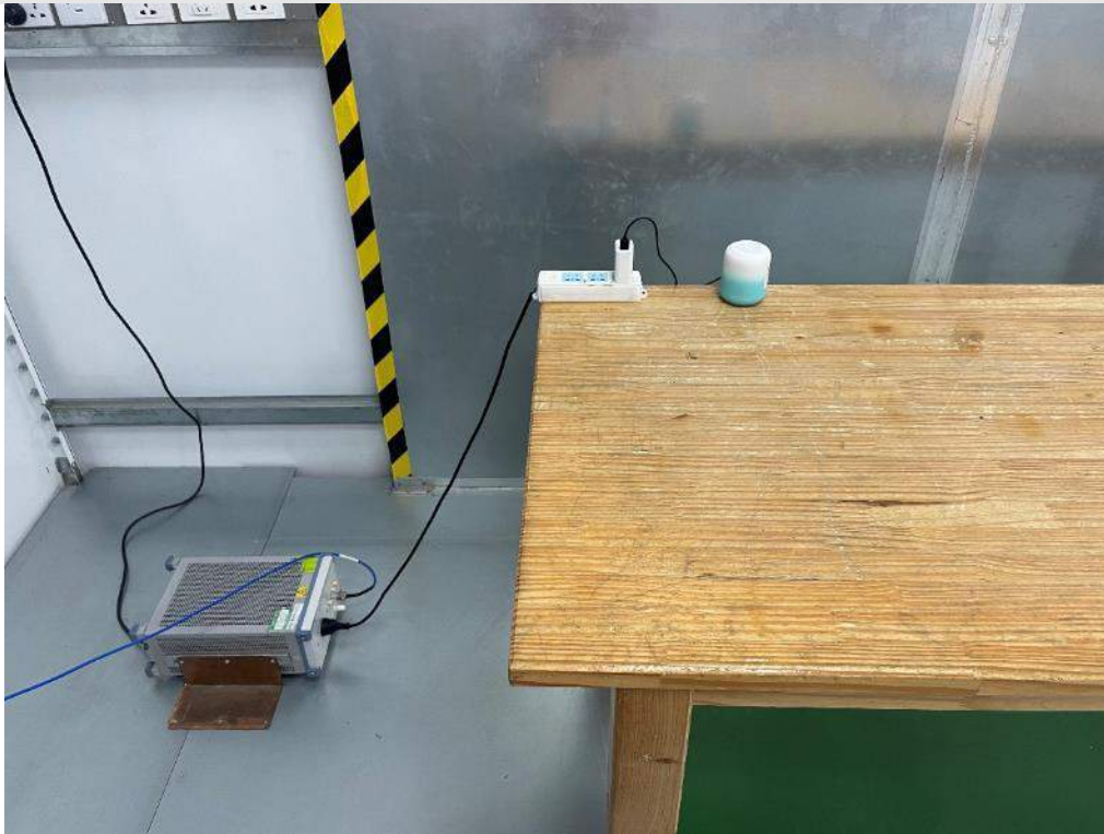
AC Power Line Conducted Emission
