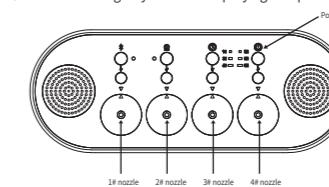
Short press the power button once to cycle through 15S-60S-120S.
