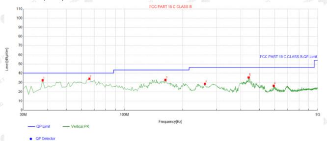
Suspected List Freq. Factor Reading Level Limit Margin Height Angle NO. Polarity [MHz] [dB] [dBµV/m] [dBµV/m] [dBµV/m] [dB] [cm] [°] 37.767768 -15.62 48.20 32.58 40.00 7.42 100 192 Vertical 2 65.925926 -15.15 100 168 49.46 34.31 40.00 5.69 Vertical 3 163.02302 -17.19 50.24 33.05 43.50 10.45 100 350 Vertical 4 261.09109 -12.73 41.56 28.83 46.00 17.17 100 178 Vertical 5 439.74975 -8.46 44.19 35.73 46.00 10.27 100 77 Vertical 592.19219 -5.33 31.89 26.56 46.00 6 19.44 100 170 Vertical
