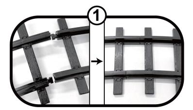
For easiest assembly, connect track pieces together on the ground.
