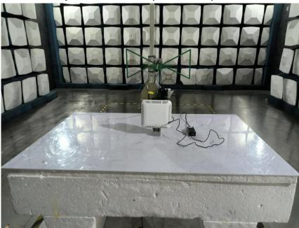
RF Radiated Spurious Emissions (1GHz -18GHz)
