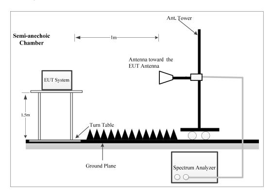
Place the measurement antenna at a measurement distance that is in the far-field of the measurement antenna, in the far-field of the EUT antenna. The EIRP test was performed at 1m distance, which was larger than the minimum test distance, please refer to section 4.3.4 for more detail.
