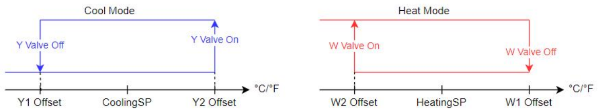
FIGURE 19: TWO PIPE COOLING AND HEATING MODE
