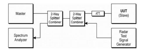
Figure 3-1. Conducted Test Setup for DFS
