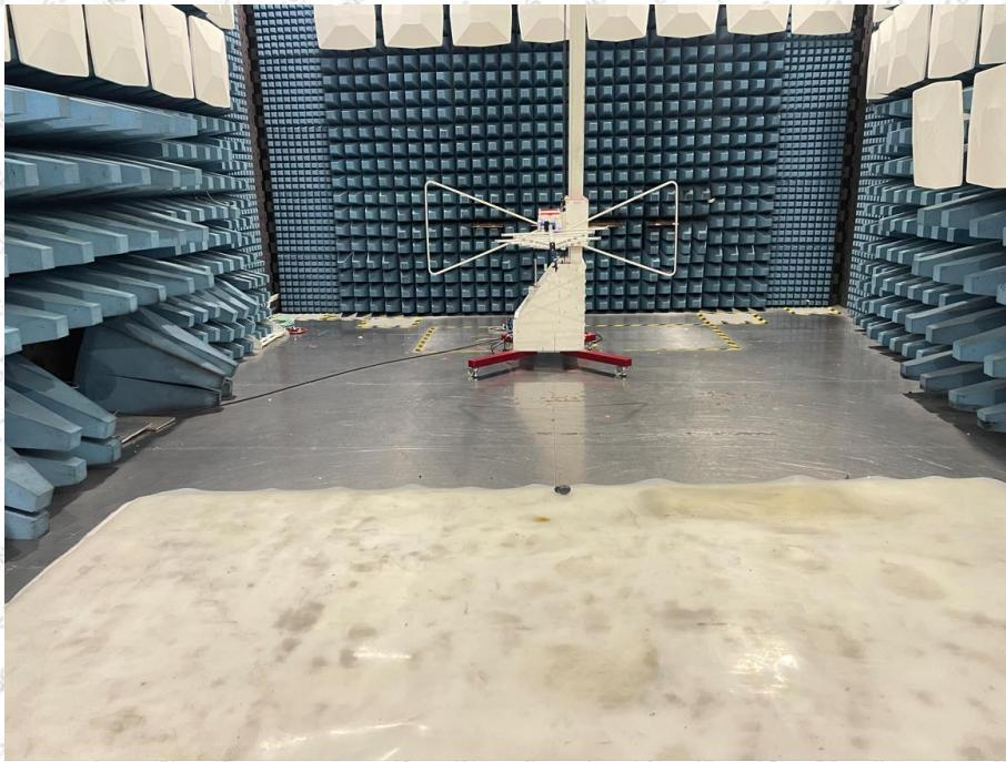
**Radiated Emissions (Above 1 GHz)**
