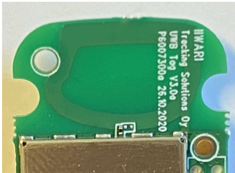
Figure 3. Photo of CloudTag antenna
