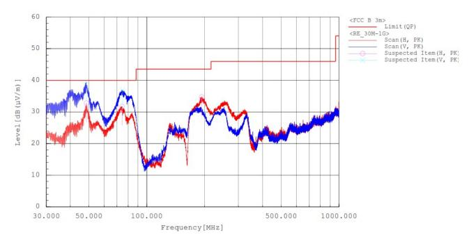
Result Frequency Reading c.f Limit No. Pol. Margin[dB] Remark [MHz] [dBuV] [dB/m] [dBuV/m] [dBuV/m] 1 48.527 Н 49.7 -16.9 32.8 40.0 7.2 2 48.527 ٧ 56.5 -16.9 39.6 40.0 0.4 74.329 50.3 40.0 3 Н -18.6 31.7 8.3 4 74.814 ٧ 55.5 -18.6 36.9 40.0 3.1 5 192.669 Н 50.0 -15.2 34.8 43.5 8.7
