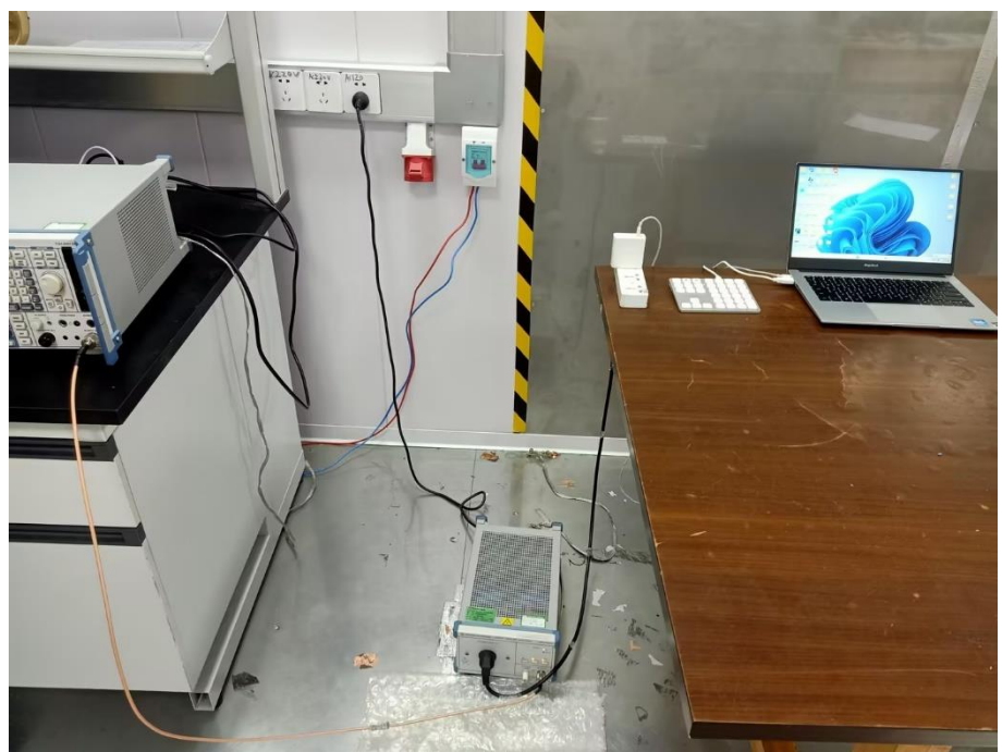
Conducted Emission Test Setup
