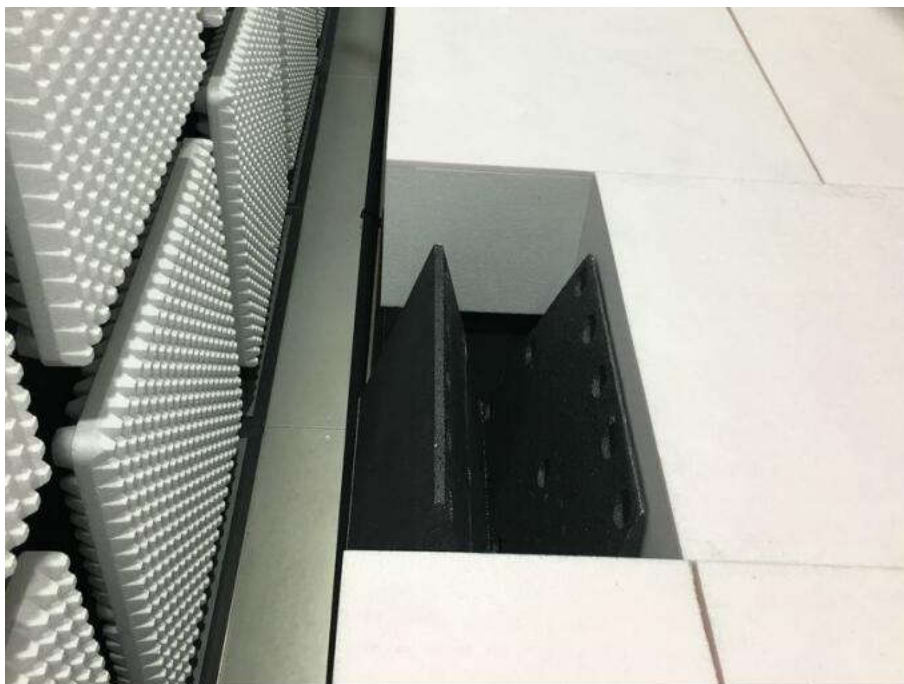
Radiated spurious emission Test Setup-7 There are absorbing materials under the ground.
