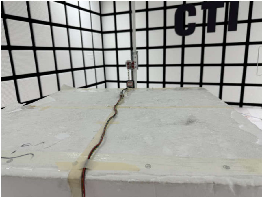
Radiated spurious emission Test Setup-3(Above 1GHz)
