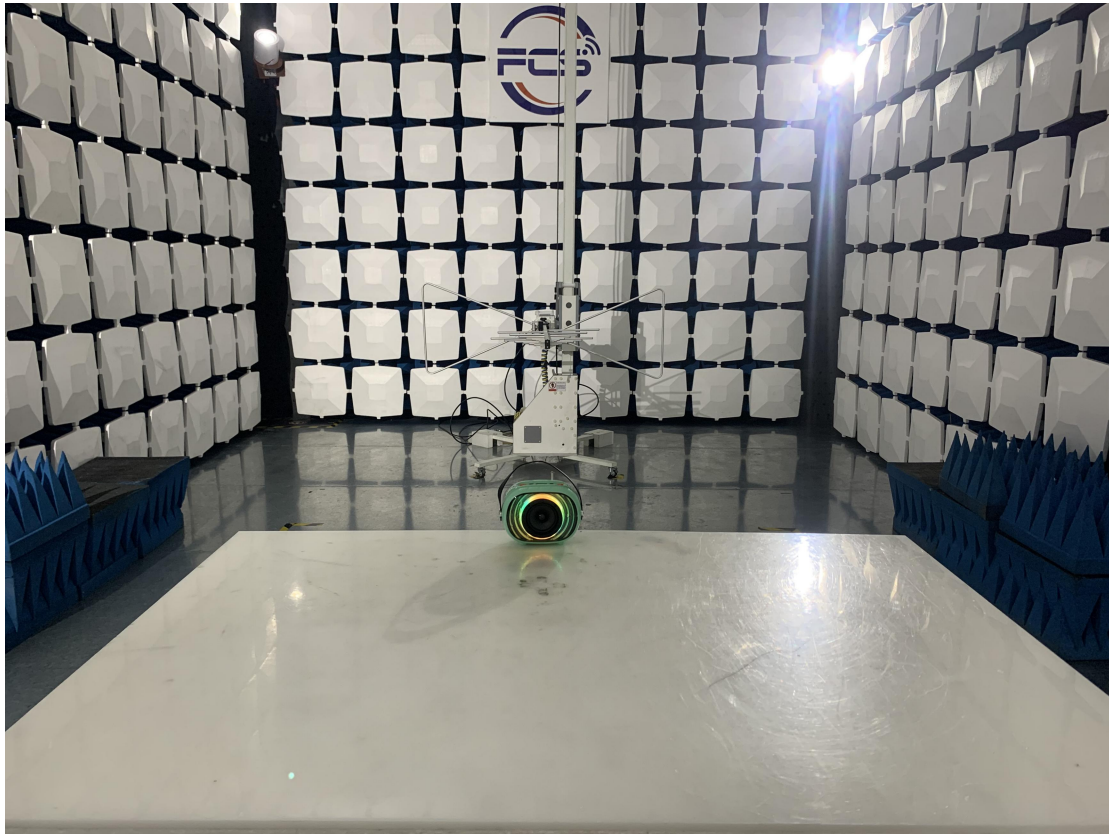
Above 1GHz for radiated emission test setup
