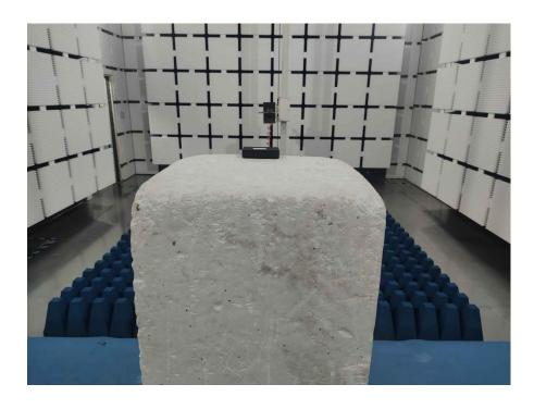
Conducted Emissions at AC Power Line (150kHz-30MHz)
