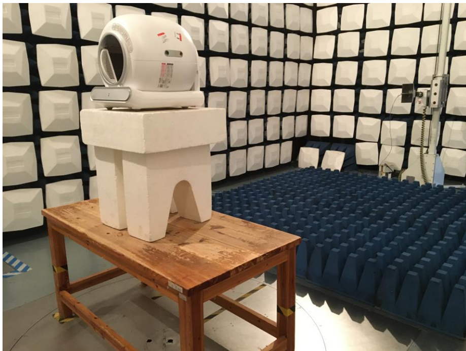
Test Setup For Radiated Emission (Above 1GHz)
