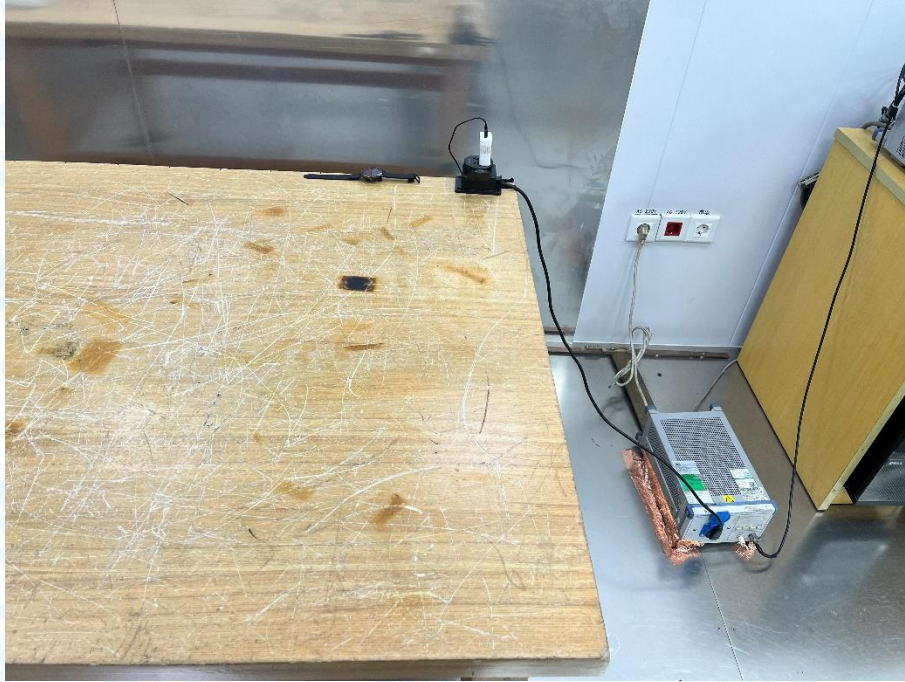
Photo of Setup for Radiated Emission (30MHz~1GHz)
