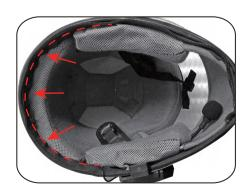
Tuck the speaker connection cables into the helmet's interior lining.
