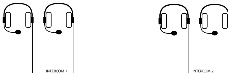
Figure 7.1.: The intercom function is active. All participants on INTERCOM 1 can talk to each other and to the INTERCOM 2 participants, who can also talk to each other and the INTERCOM 1 participants.
