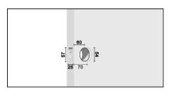
01. According to the template, hole in the door and door frame.
