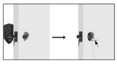
06. Insert the Exterior Assembly into the door hole. Route the cable below the latch.
