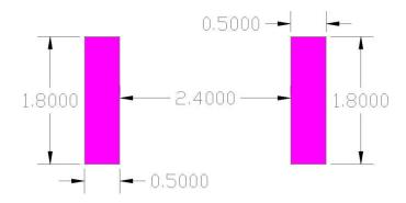
◆ 2<sup>nd</sup> Layout Dimensions in Clearance area(Size=8.0\*3.0mm)
