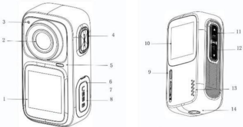
1. Front screen; 2. lens; 3. MIC ; 4. On/off switch key; 5. Front indicator light; 6. Reset hole; 7.TF card holder; 8.Typec interface
