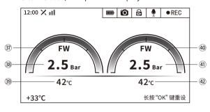
36经纬度/Longitude and latitude ③前轮胎压报警/Front tire pressure alarm (正常蓝色,报警变红/Normal blue, alarm turns red) 38前轮胎压数值/Front tire pressure value 39前轮胎温/Front tire temperature ⑩后轮胎压报警/Rear tire pressure alarm (正常蓝色,报警变红/Normal blue, alarm turns red) ④后轮胎压数值/Rear tire pressure value ④后轮胎温/Rear tire temperature
