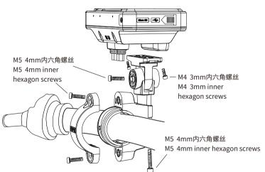
main host can be rotated in different angles. Please choose right place and adjust the angle before installation, tighten the screws
