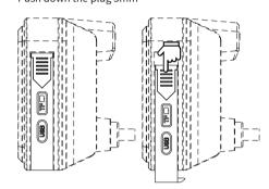
注意:TF卡金属条朝向主机屏幕,最大支持512G TF卡 Note:TF card metal side up to the main screen side (max support for 512GB TF card)
