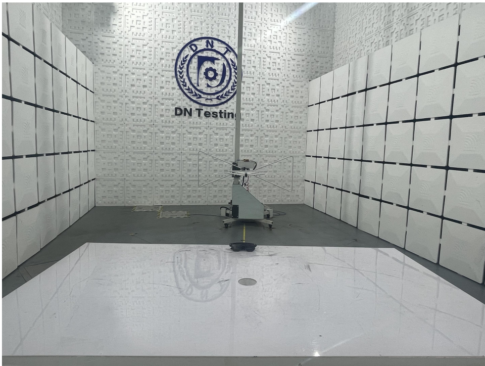
Radiated Emission Test View((Below 1G)
