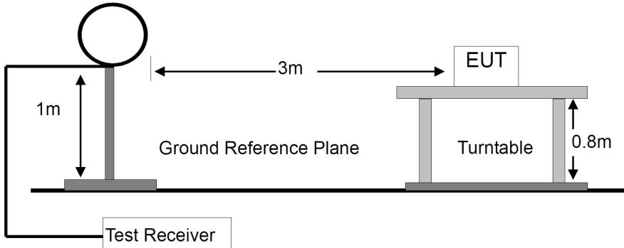
For Radiated Emission 30-1000MHz
