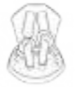
The headset is charging: the ice blue light of the headset stays on for 3 seconds and then turns off. Fully charged earphones: The earphones do not light up, and the ice blue light in the charging compartment goes out.
