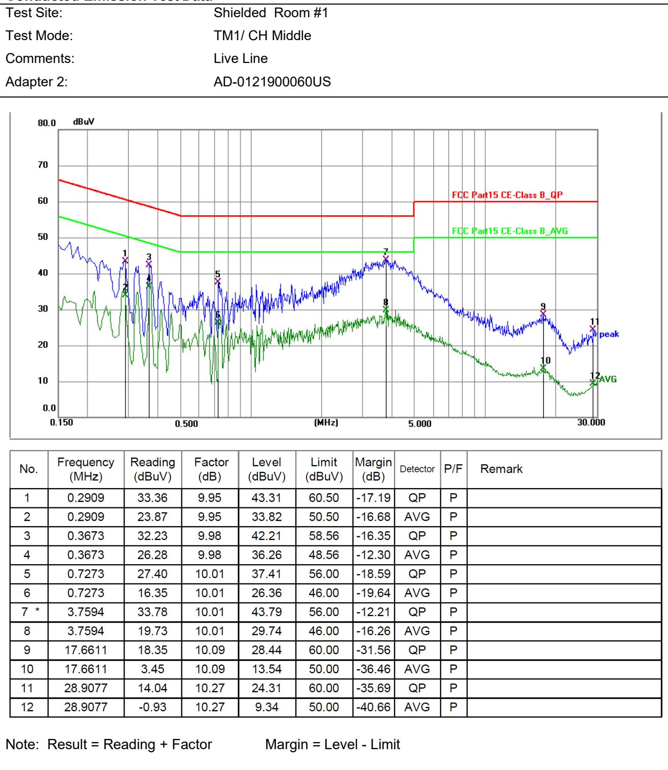
**Conducted Emission Test Data**
