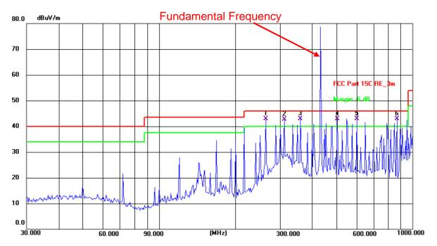
Site: 3m Anechoic Chamber Polarization: Horizontal Temperature: 24.6(C) Humidity: 53 %
