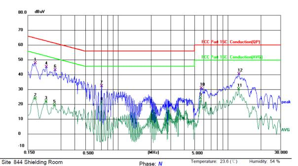
Limit: FCC Part 15C Conduction(QP)
