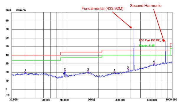
Site 3m Anechoic Chamber Polarization: Vertical Temperature: 20.3(C) Humidity: 55 %
