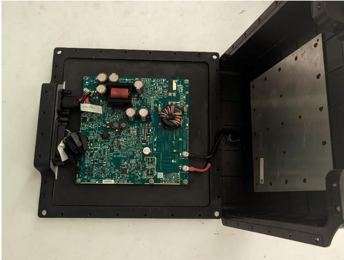
Photograph 4 – View of the PCB Mounting in the Enclosure
