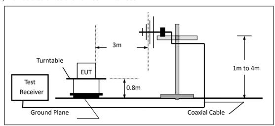
(c) For radiated emissions above 1000MHz
