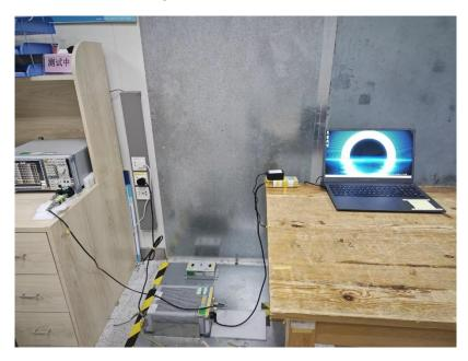
Radiated Emissions From 30MHz-1000MHz
