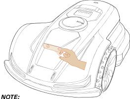
Please make sure to remove the protective film outside the front camera before use. If the lens becomes dirty during subsequent use, you can clean it with a soft cloth.
