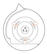
3. Use a cross-tip screwdriver to loosen the screws.
