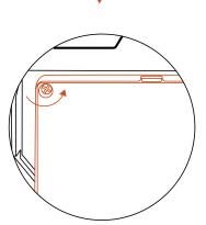
**3.** Loosen the 4 screws holding the battery. compartment in place with a cross-tip screwdriver.
