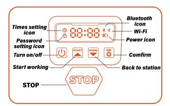
Power icon: The battery power icon shows the remain power of the machine. This icon displaying 1 bar indicates that the power is 30% or under, displaying 2 bars indicates that the remain power is between 31-66%, and displaying 3 bars indicates power of 67% and higher.
