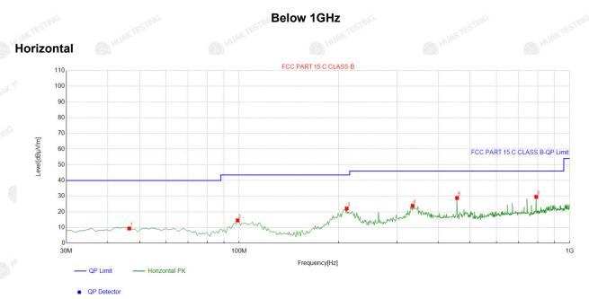
Suspected List Freq. Factor Level Limit Reading Margin Height Angle NO. Polarity [MHz] [dB] [dBµV/m] [dBµV/m] [dBµV/m] [dB] [cm] [°] 226.13613 -13.91 35.58 21.67 46.00 24.33 100 255 Horizontal 1 2 328.08808 -10.93 42.01 31.08 46.00 14.92 100 110 Horizontal 384.40440 46.59 8.47 3 -9.06 37.53 46.00 100 103 Horizontal 421.30130 -9.09 43.79 46.00 11.30 100 4 34.70 41 Horizontal 5 513.54354 -8.01 36.11 28.10 46.00 17.90 100 14 Horizontal -4.50 37.03 46.00 100 6 671.81181 32.53 13.47 96 Horizontal
