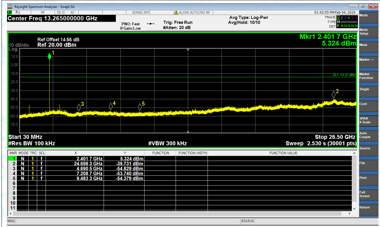
Tx. Spurious NVNT 1-DH1 2402MHz Ant1 Emission
