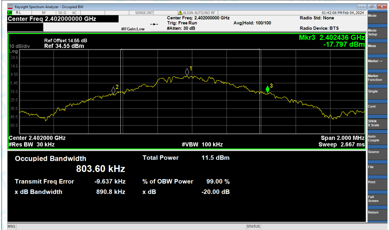
-20dB Bandwidth NVNT 1-DH1 2441MHz Ant1
