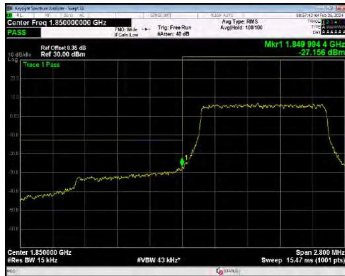
Band2 QPSK BW=1.4MHz Channel=19193 RB Size=1 Position=#0
