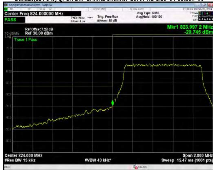
Band26(824-849) QPSK BW=1.4MHz Channel=27033 RB Size=6 Position=#0
