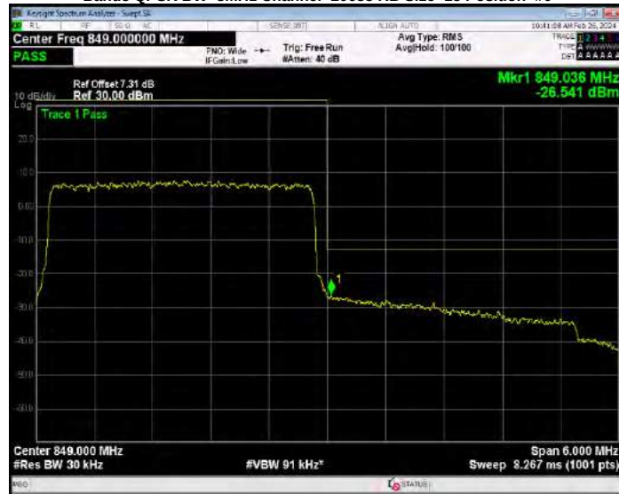
Band5 QPSK BW=5MHz Channel=20425 RB Size=1 Position=#0
