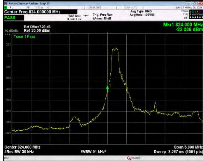
Band5 16QAM BW=3MHz Channel=20415 RB Size=15 Position=#0
