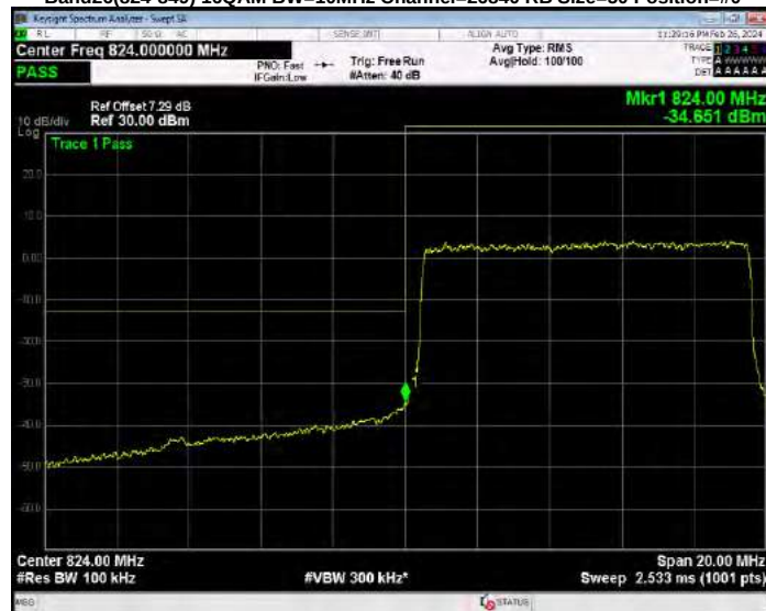
Band26(824-849) 16QAM BW=10MHz Channel=26990 RB Size=50 Position=#0
