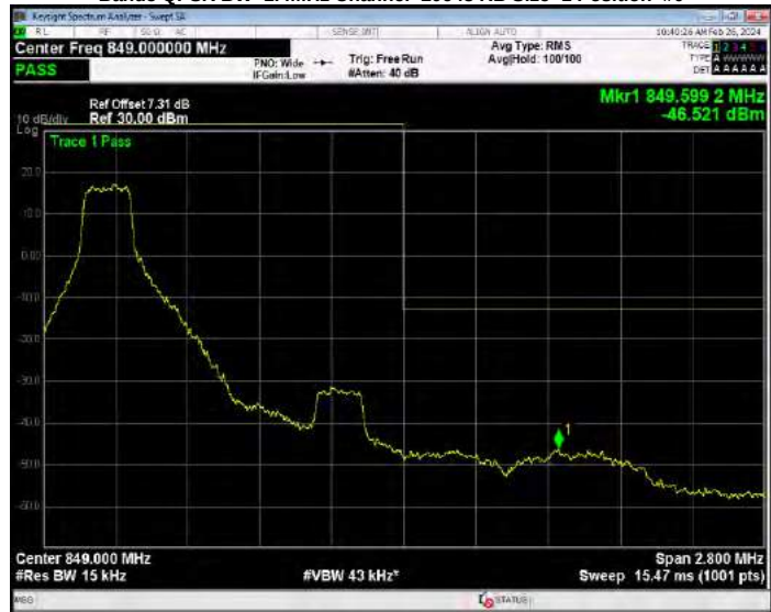
Band5 QPSK BW=1.4MHz Channel=20643 RB Size=6 Position=#0
