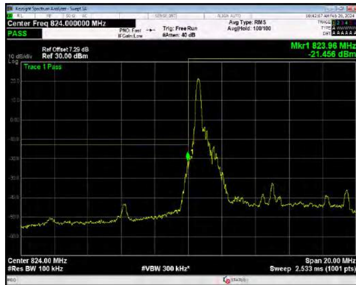
Band5 16QAM BW=10MHz Channel=20450 RB Size=50 Position=#0
