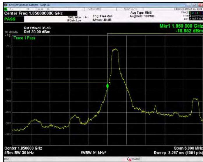
Band2 QPSK BW=3MHz Channel=18615 RB Size=15 Position=#0
