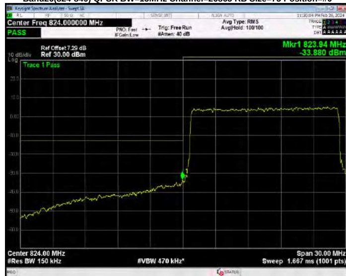
Band26(824-849) QPSK BW=15MHz Channel=26965 RB Size=75 Position=#0
