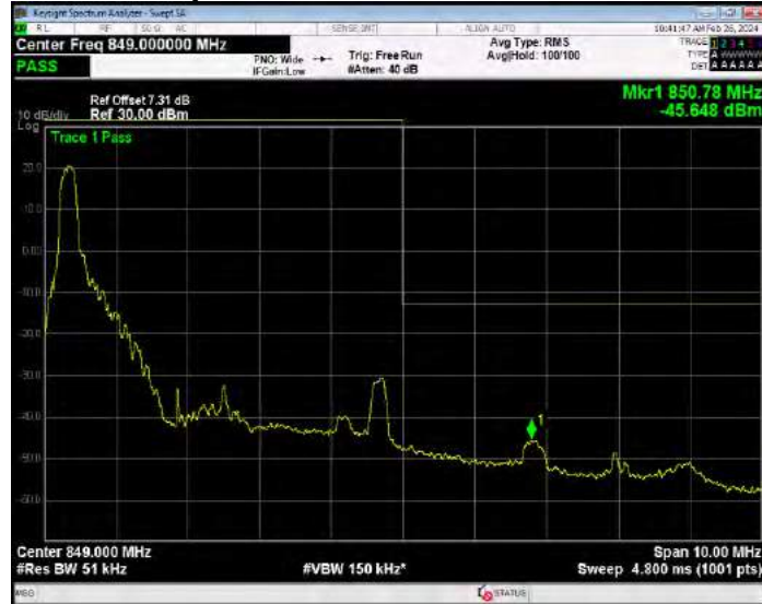
Band5 16QAM BW=5MHz Channel=20625 RB Size=25 Position=#0
