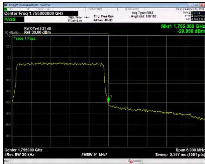
Band4 QPSK BW=5MHz Channel=19975 RB Size=1 Position=#0
