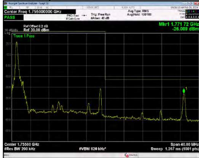
Band4 16QAM BW=20MHz Channel=20300 RB Size=100 Position=#0
