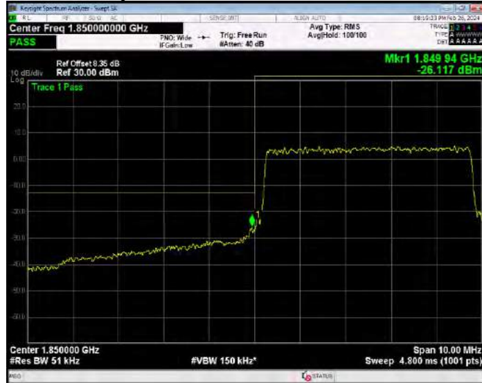
Band25 16QAM BW=5MHz Channel=26665 RB Size=25 Position=#0
