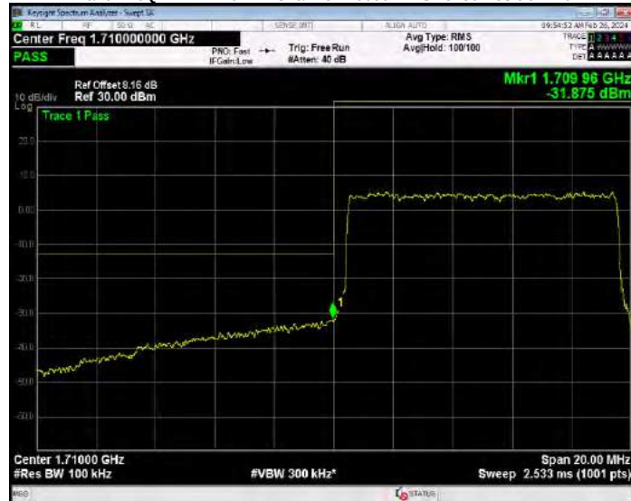
Band4 16QAM BW=10MHz Channel=20350 RB Size=1 Position=#0
