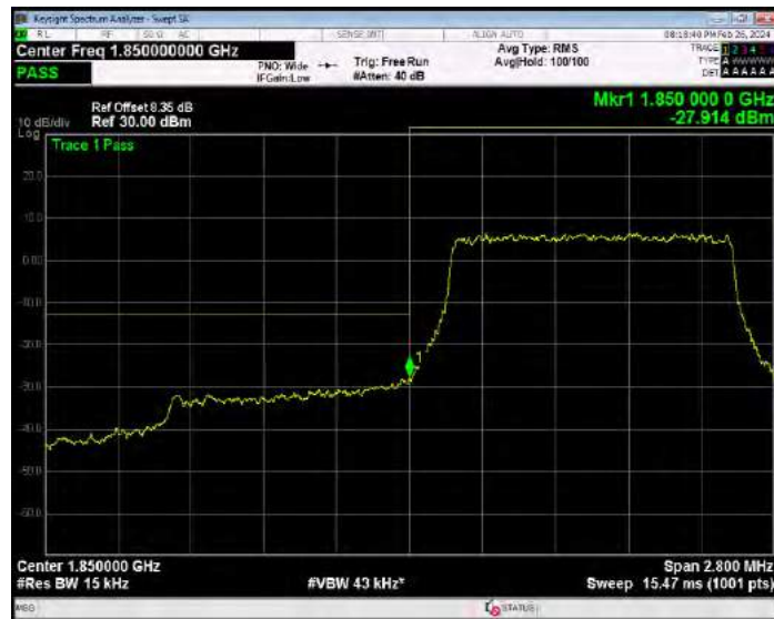
Band25 QPSK BW=1.4MHz Channel=26683 RB Size=6 Position=#0
