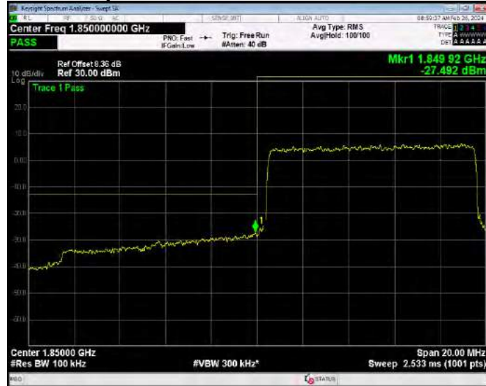
Band2 QPSK BW=10MHz Channel=19150 RB Size=1 Position=#0
