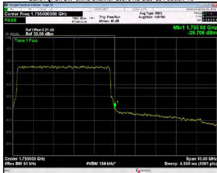
Band5 16QAM BW=1.4MHz Channel=20407 RB Size=1 Position=#0
