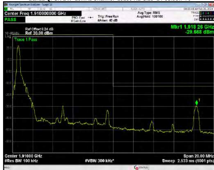
Band2 QPSK BW=10MHz Channel=19150 RB Size=50 Position=#0
