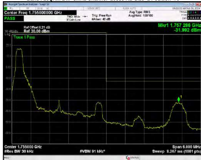
Band4 16QAM BW=3MHz Channel=20385 RB Size=15 Position=#0
