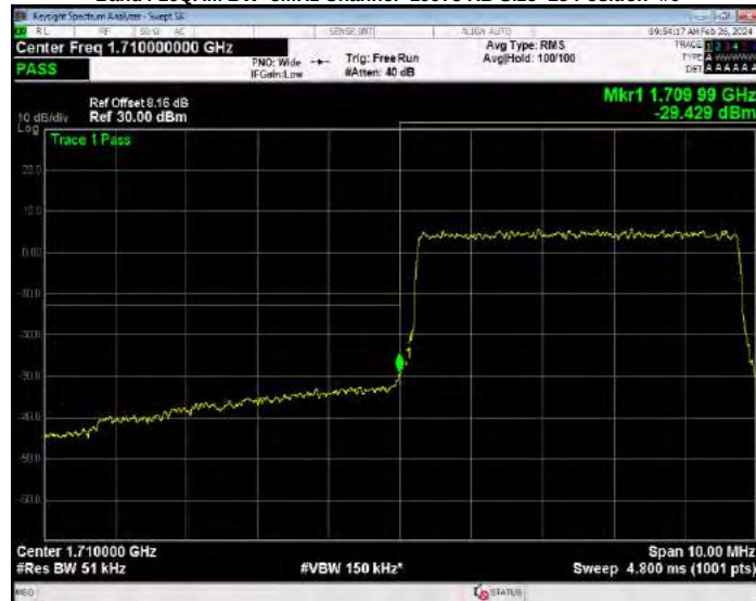
Band4 16QAM BW=5MHz Channel=20375 RB Size=1 Position=#0
