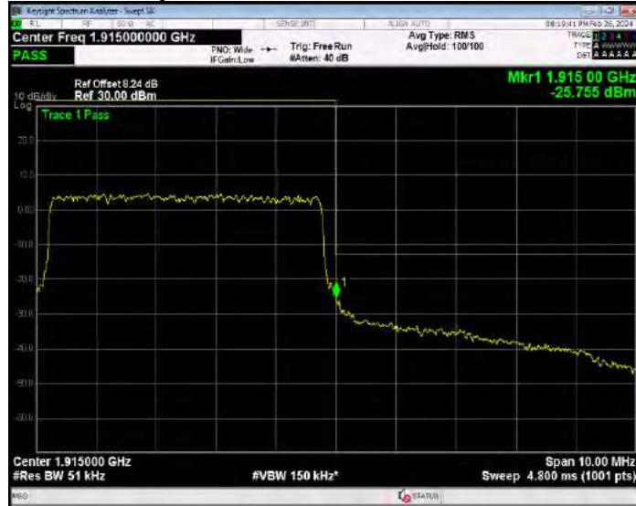
Band25 QPSK BW=1.4MHz Channel=26047 RB Size=6 Position=#0
