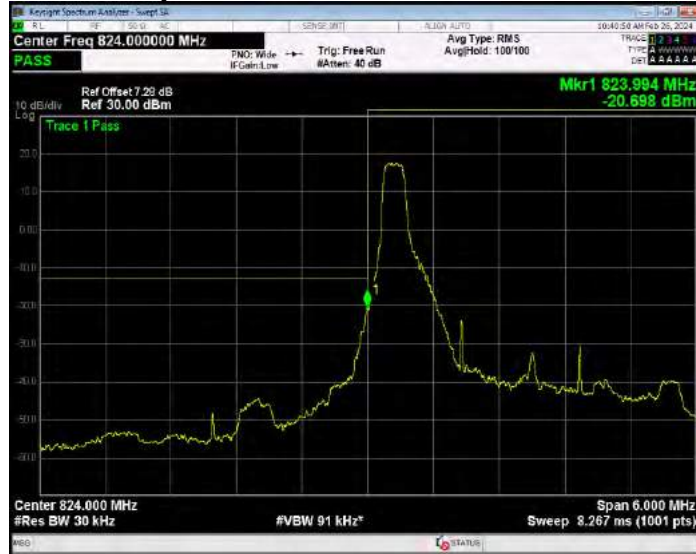
Band5 QPSK BW=3MHz Channel=20415 RB Size=15 Position=#0
