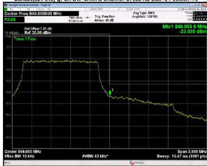
Band26(824-849) QPSK BW=10MHz Channel=26840 RB Size=50 Position=#0
