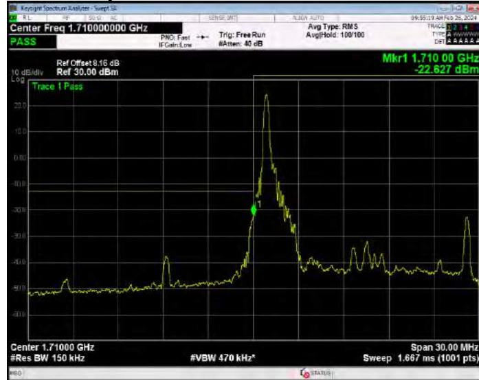
Band4 QPSK BW=15MHz Channel=20025 RB Size=75 Position=#0
