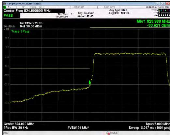
Band5 16QAM BW=3MHz Channel=20635 RB Size=1 Position=#0
