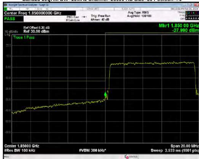
Band25 16QAM BW=10MHz Channel=26640 RB Size=50 Position=#0
