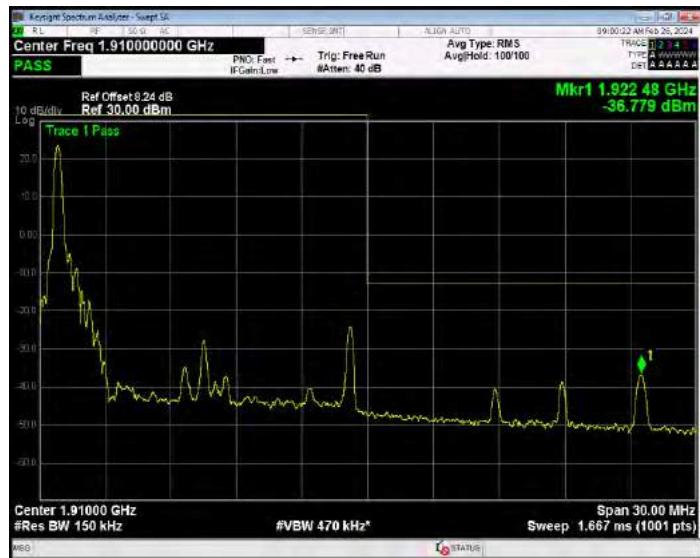
Band2 QPSK BW=15MHz Channel=19125 RB Size=75 Position=#0
