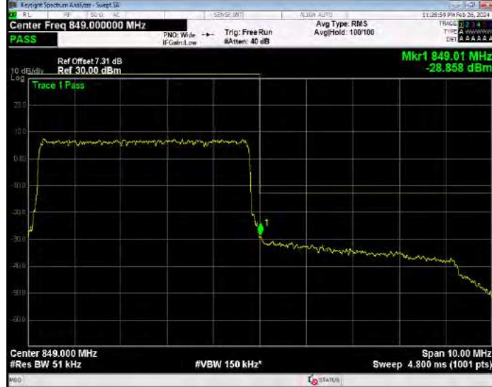
Band26(814-824) 16QAM BW=1.4MHz Channel=26697 RB Size=6 Position=#0
