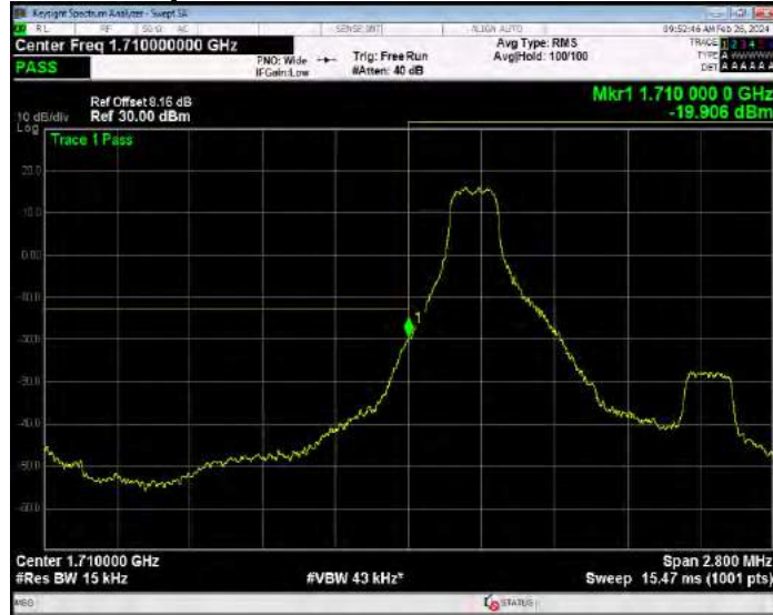
Band4 QPSK BW=1.4MHz Channel=19957 RB Size=6 Position=#0
