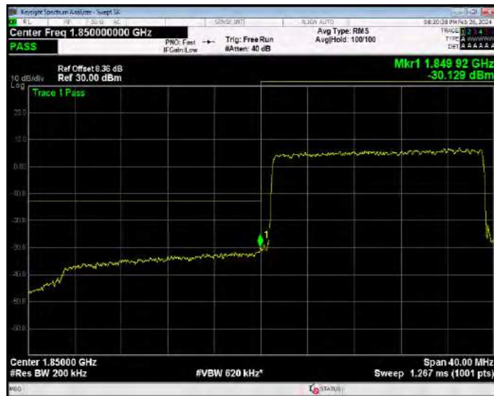
Band25 QPSK BW=20MHz Channel=26590 RB Size=100 Position=#0
