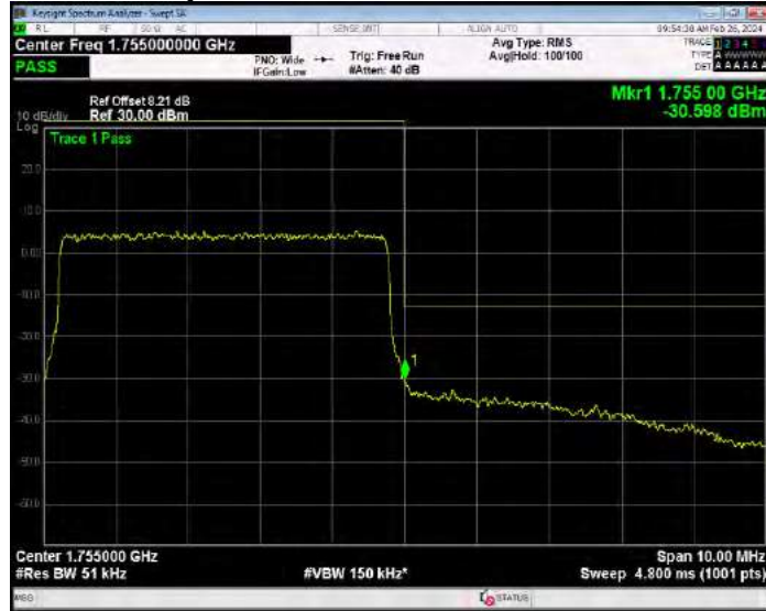
Band4 QPSK BW=1.4MHz Channel=19957 RB Size=1 Position=#0
