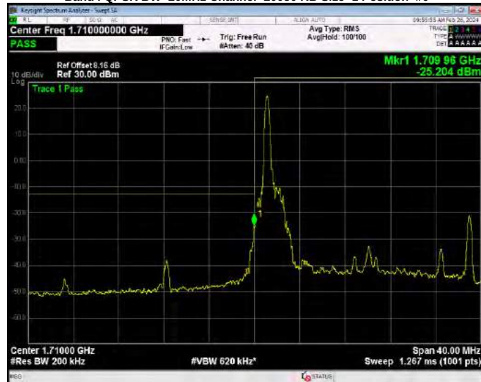
Band4 QPSK BW=20MHz Channel=20050 RB Size=100 Position=#0
