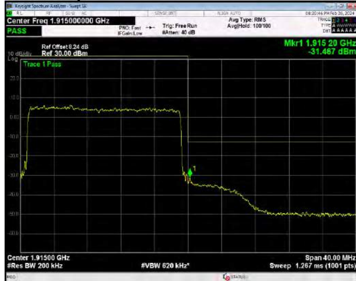
Band25 QPSK BW=3MHz Channel=26055 RB Size=15 Position=#0
