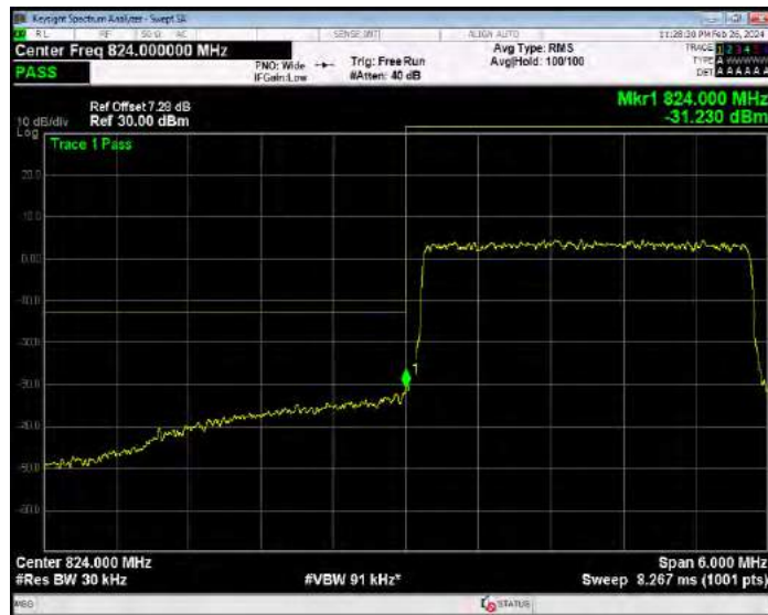
Band26(824-849) 16QAM BW=3MHz Channel=27025 RB Size=15 Position=#0
