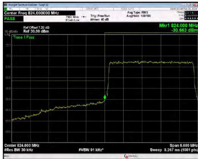
Band5 QPSK BW=3MHz Channel=20635 RB Size=1 Position=#0
