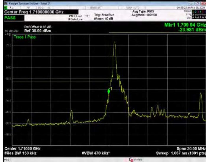
Band4 16QAM BW=15MHz Channel=20025 RB Size=75 Position=#0
