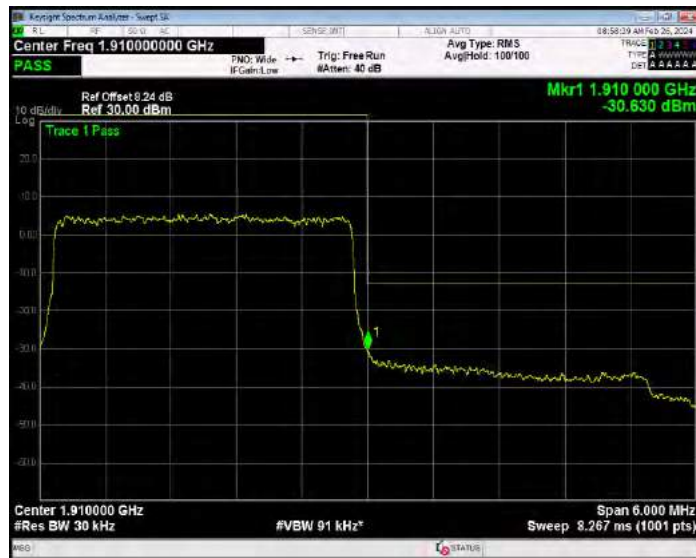
Band2 QPSK BW=5MHz Channel=18625 RB Size=1 Position=#0
