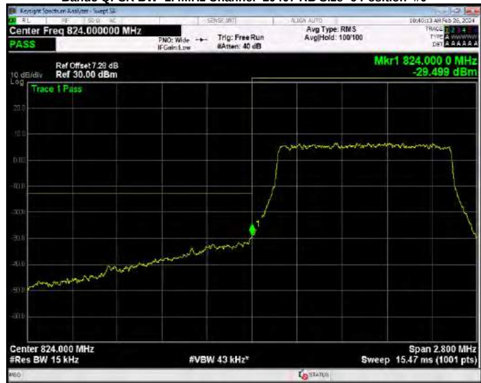
Band5 QPSK BW=1.4MHz Channel=20643 RB Size=1 Position=#0
