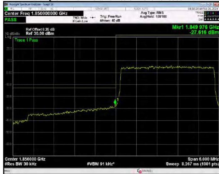
Band2 QPSK BW=3MHz Channel=19185 RB Size=1 Position=#0
