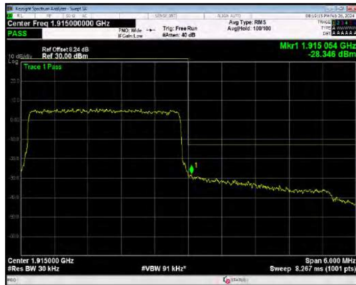
Band25 QPSK BW=5MHz Channel=26065 RB Size=25 Position=#0
