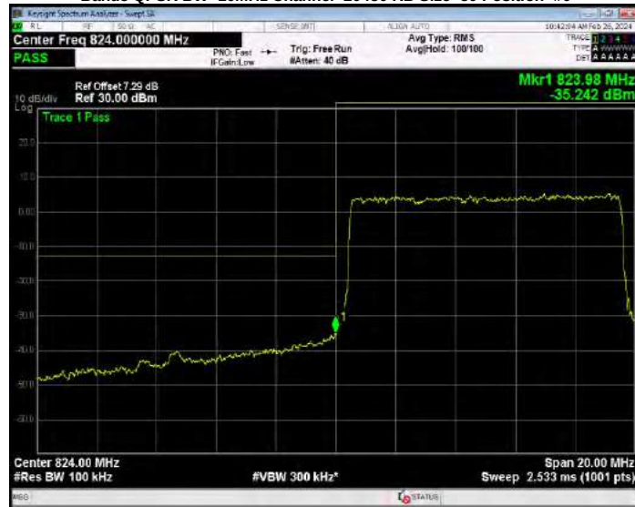
Band5 QPSK BW=10MHz Channel=20600 RB Size=1 Position=#0
