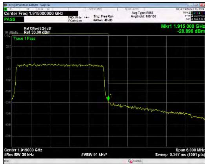
Band25 16QAM BW=5MHz Channel=26065 RB Size=25 Position=#0
