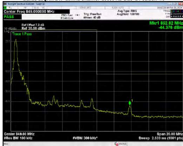
Band5 16QAM BW=10MHz Channel=20600 RB Size=50 Position=#0
