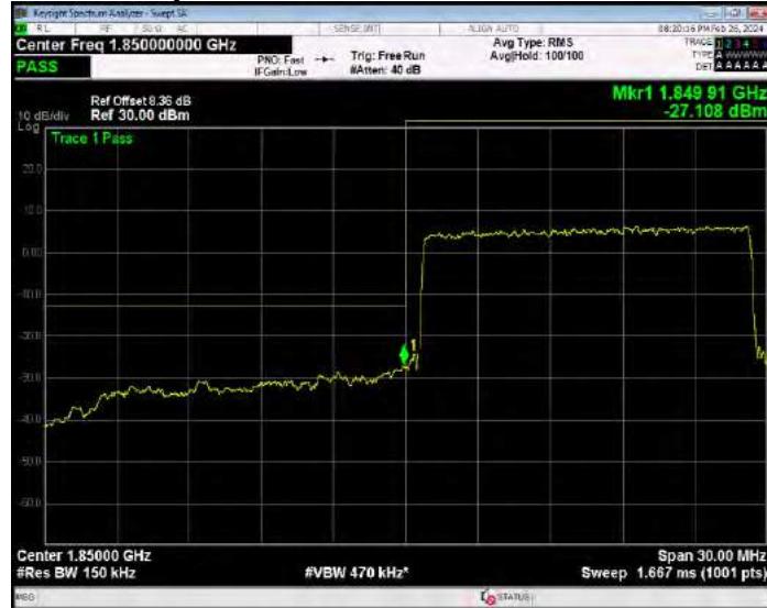
Band25 QPSK BW=15MHz Channel=26615 RB Size=75 Position=#0
