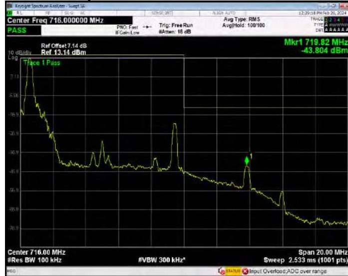
Band17 16QAM BW=10MHz Channel=23800 RB Size=50 Position=#0
