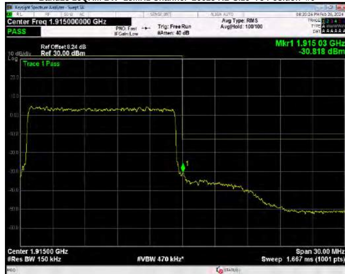
Band25 16QAM BW=20MHz Channel=26140 RB Size=100 Position=#0
