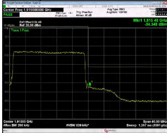
Band25 16QAM BW=3MHz Channel=26055 RB Size=15 Position=#0
