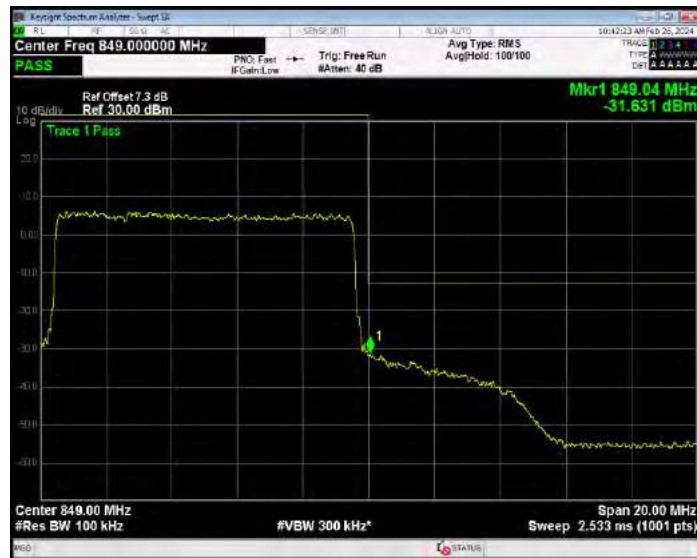
Band5 16QAM BW=3MHz Channel=20415 RB Size=1 Position=#0
