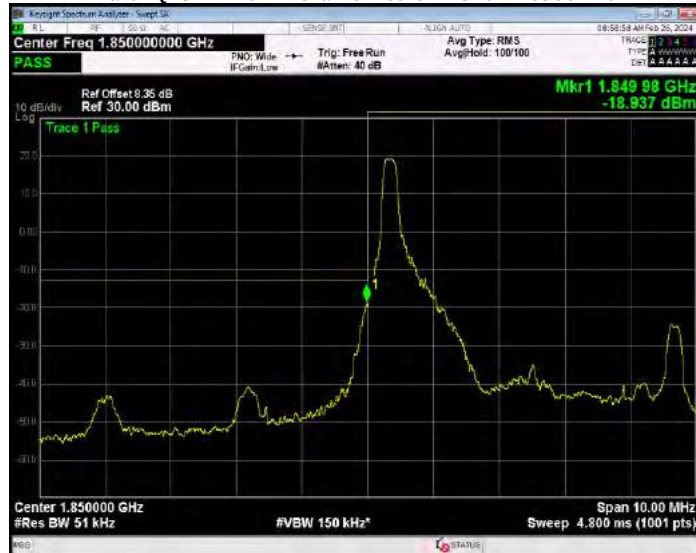
Band2 QPSK BW=5MHz Channel=18625 RB Size=25 Position=#0
