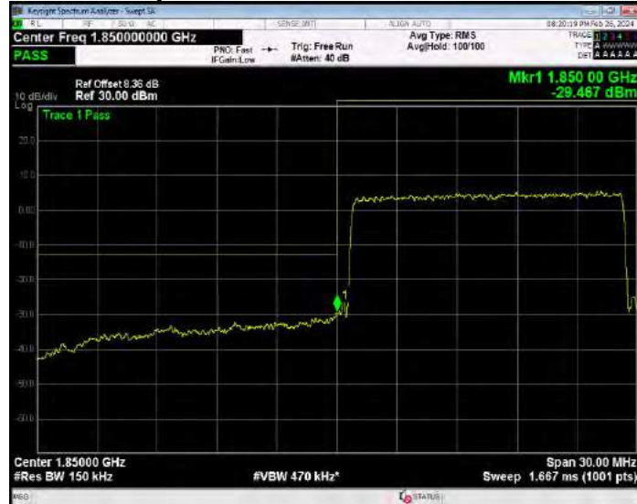
Band25 16QAM BW=15MHz Channel=26115 RB Size=75 Position=#0
