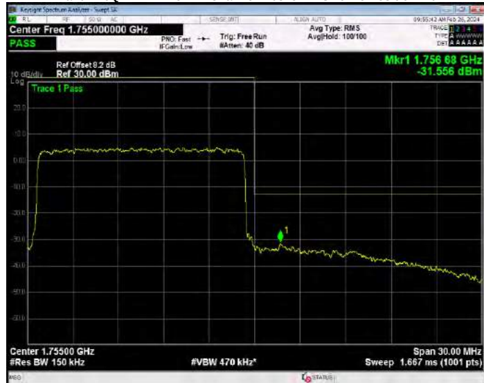
Band4 16QAM BW=20MHz Channel=20050 RB Size=1 Position=#0
