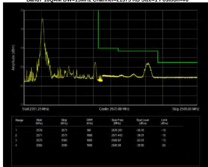
Band7 16QAM BW=15MHz Channel=21375 RB Size=75 Position=#0
