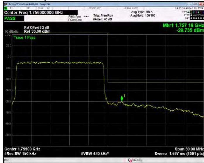
Band4 QPSK BW=20MHz Channel=20050 RB Size=1 Position=#0
