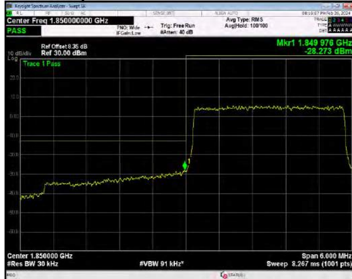
Band25 QPSK BW=3MHz Channel=26675 RB Size=15 Position=#0
