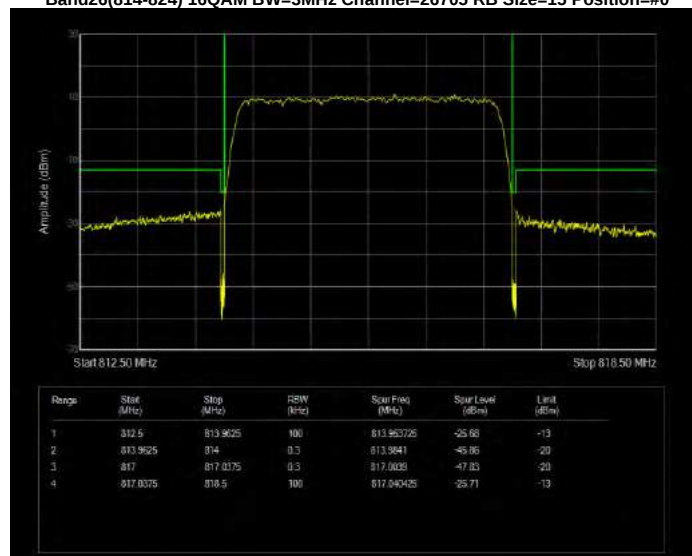
Band26(814-824) 16QAM BW=3MHz Channel=26775 RB Size=15 Position=#0
