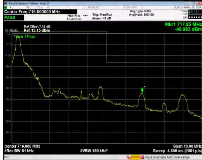
Band17 QPSK BW=5MHz Channel=23825 RB Size=25 Position=#0
