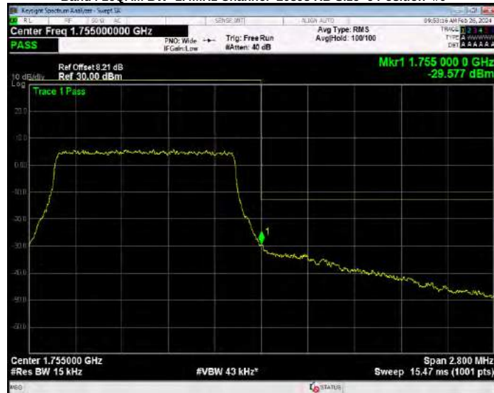
Band4 16QAM BW=10MHz Channel=20000 RB Size=1 Position=#0
