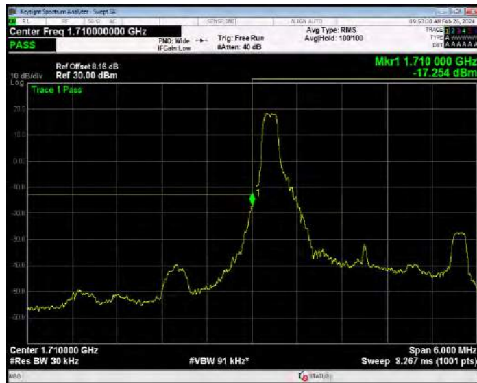
Band4 QPSK BW=3MHz Channel=19965 RB Size=15 Position=#0
