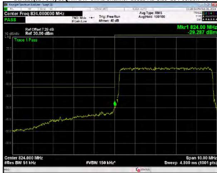
Band26(824-849) 16QAM BW=5MHz Channel=27015 RB Size=25 Position=#0
