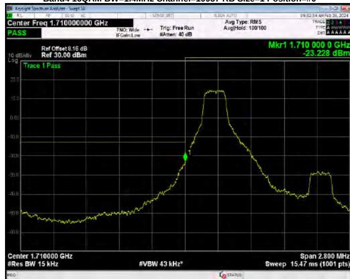
Band4 16QAM BW=1.4MHz Channel=19957 RB Size=6 Position=#0
