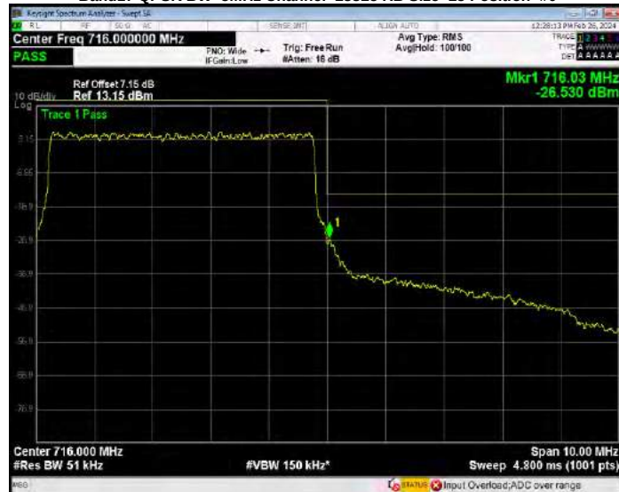
Band25 16QAM BW=1.4MHz Channel=26047 RB Size=6 Position=#0
