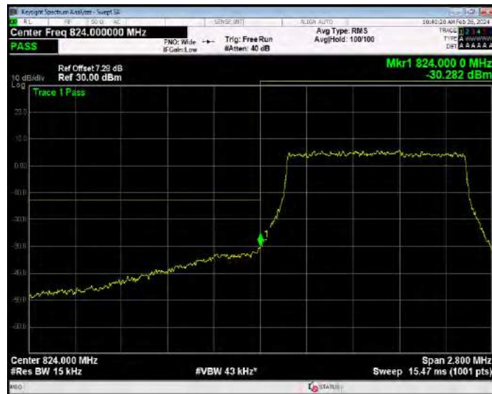
Band5 16QAM BW=1.4MHz Channel=20643 RB Size=1 Position=#0
