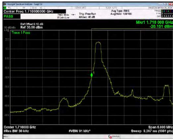
Band4 16QAM BW=3MHz Channel=19965 RB Size=15 Position=#0
