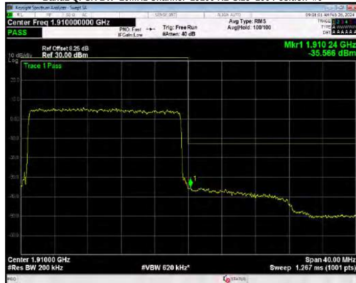
Band2 QPSK BW=3MHz Channel=18615 RB Size=1 Position=#0
