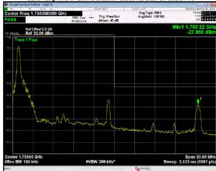
Band4 16QAM BW=10MHz Channel=20350 RB Size=50 Position=#0
