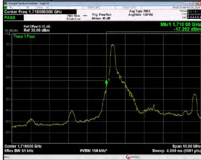
Band4 16QAM BW=5MHz Channel=19975 RB Size=25 Position=#0
