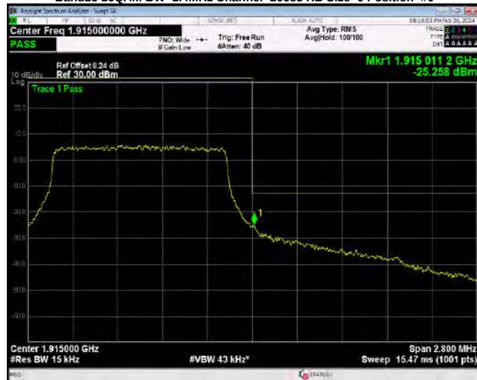
Band25 16QAM BW=10MHz Channel=26090 RB Size=50 Position=#0
