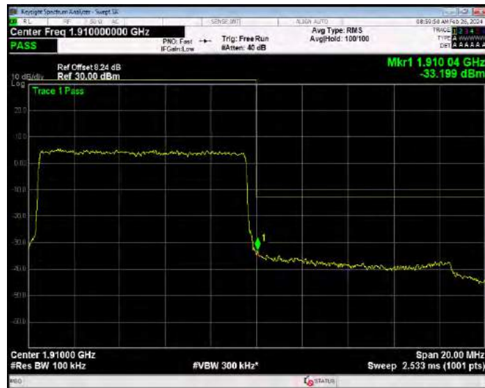
Band2 QPSK BW=15MHz Channel=18675 RB Size=1 Position=#0
