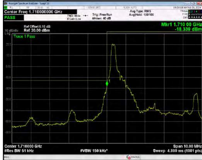
Band4 QPSK BW=5MHz Channel=19975 RB Size=25 Position=#0
