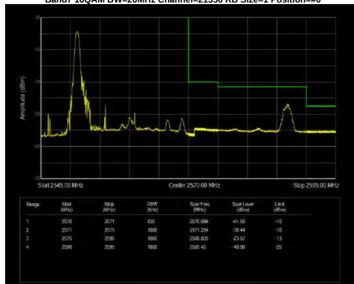
Band7 16QAM BW=20MHz Channel=21350 RB Size=100 Position=#0
