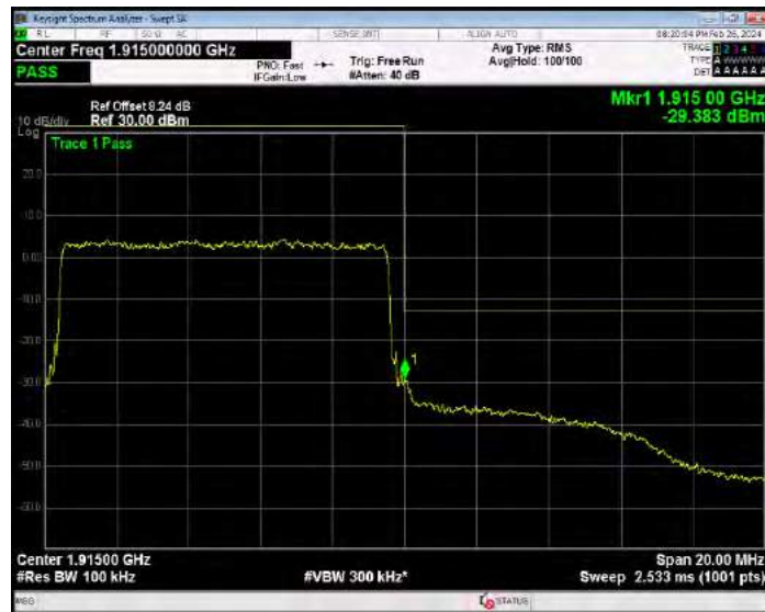
Band25 16QAM BW=15MHz Channel=26115 RB Size=75 Position=#0
