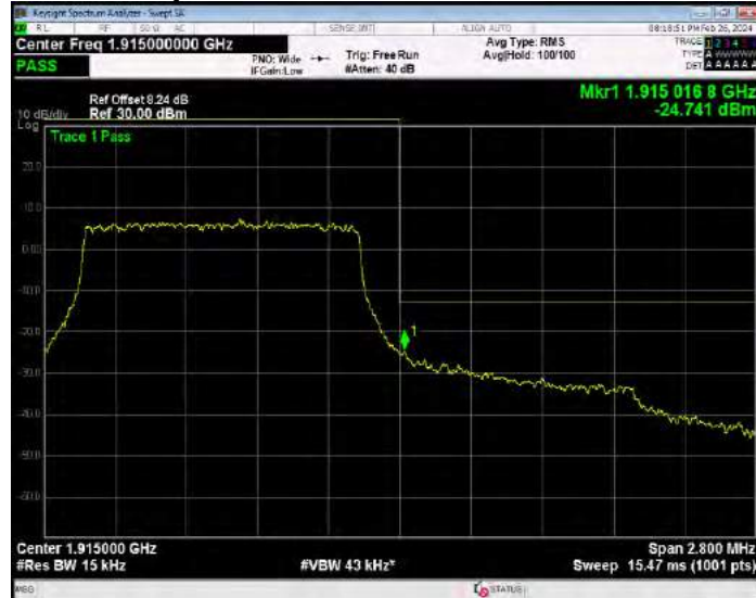
Band25 QPSK BW=10MHz Channel=26090 RB Size=50 Position=#0
