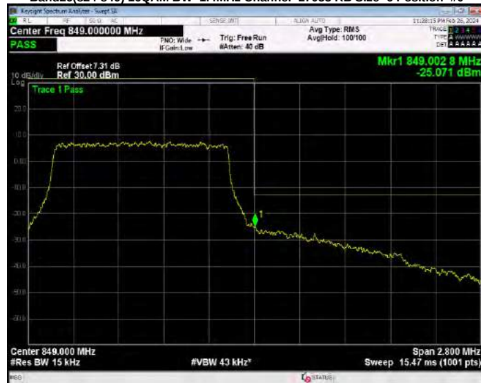
Band26(824-849) 16QAM BW=10MHz Channel=26840 RB Size=50 Position=#0
