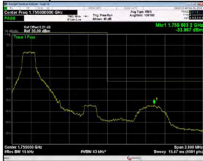
Band4 16QAM BW=1.4MHz Channel=20393 RB Size=6 Position=#0
