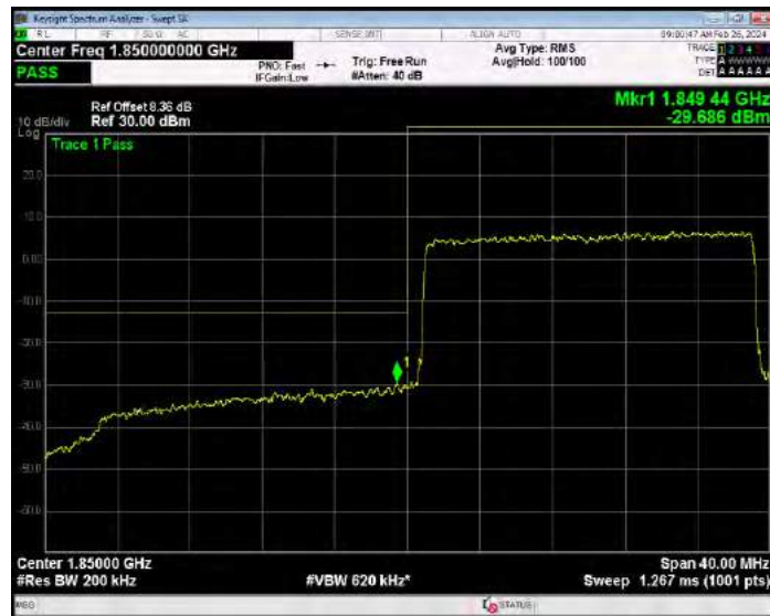
Band2 QPSK BW=20MHz Channel=19100 RB Size=1 Position=#0
