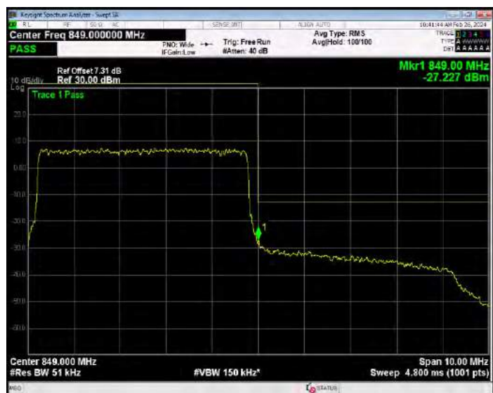
Band7 16QAM BW=10MHz Channel=20800 RB Size=1 Position=#0
