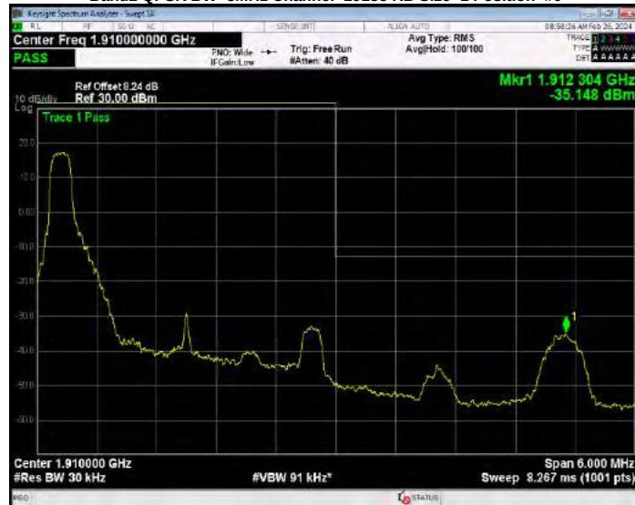
Band2 QPSK BW=3MHz Channel=19185 RB Size=15 Position=#0
