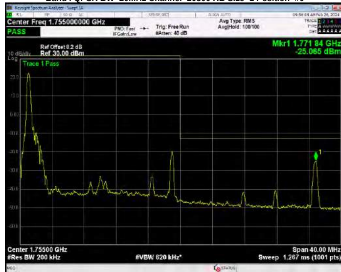
Band4 QPSK BW=20MHz Channel=20300 RB Size=100 Position=#0
