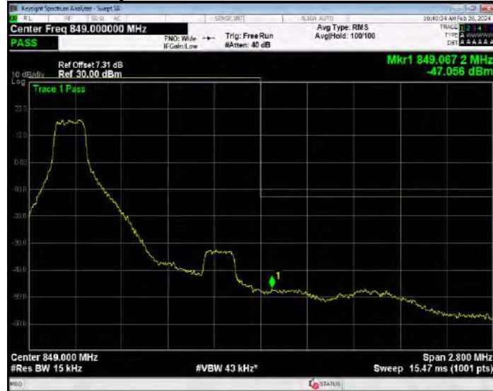
Band5 16QAM BW=1.4MHz Channel=20643 RB Size=6 Position=#0
