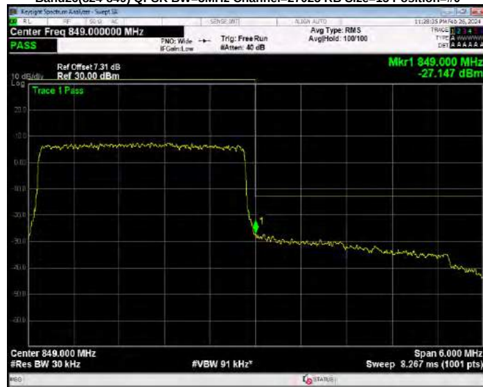
Band26(824-849) QPSK BW=5MHz Channel=26815 RB Size=25 Position=#0
