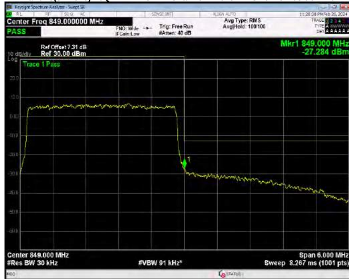
Band26(824-849) 16QAM BW=5MHz Channel=26815 RB Size=25 Position=#0
