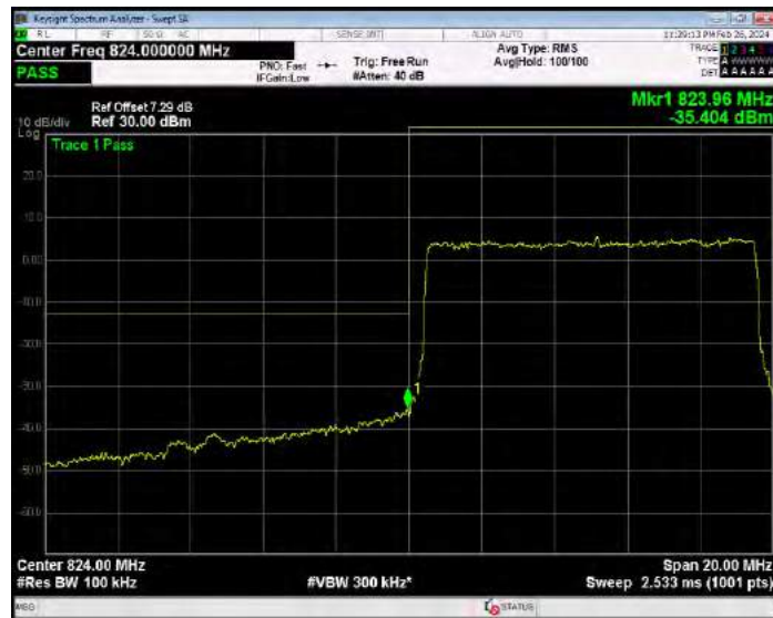
Band26(824-849) QPSK BW=10MHz Channel=26990 RB Size=50 Position=#0
