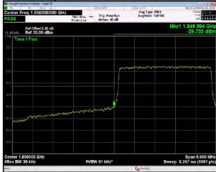
Band25 16QAM BW=3MHz Channel=26675 RB Size=15 Position=#0
