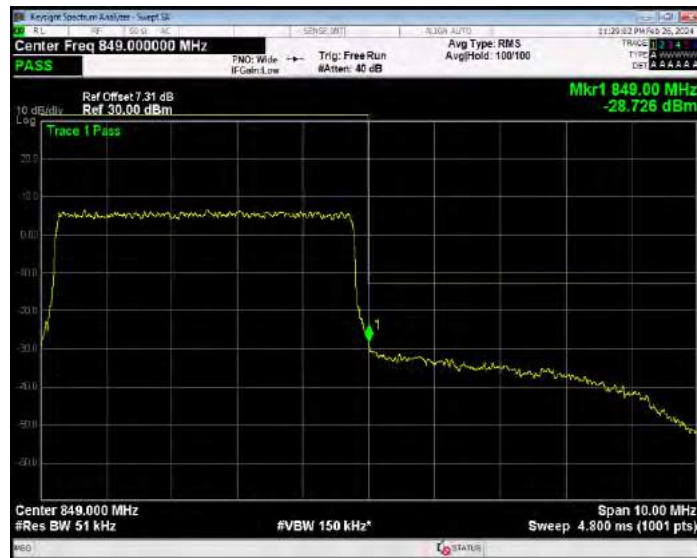
Band26(824-849) QPSK BW=1.4MHz Channel=26797 RB Size=6 Position=#0
