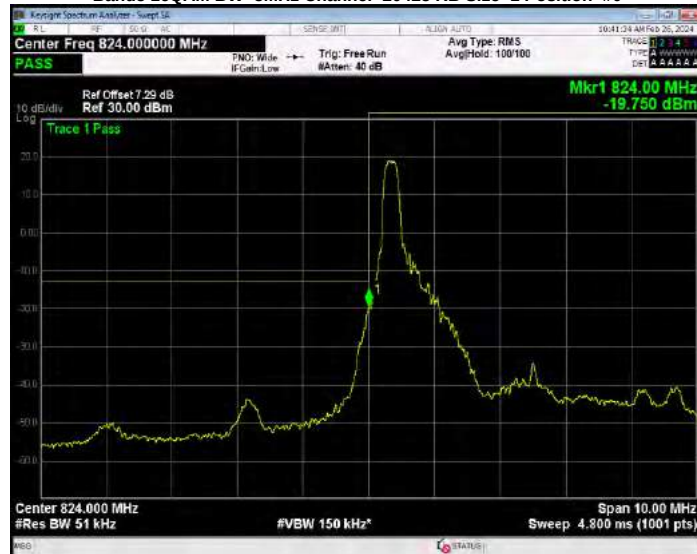
Band5 16QAM BW=5MHz Channel=20425 RB Size=25 Position=#0
