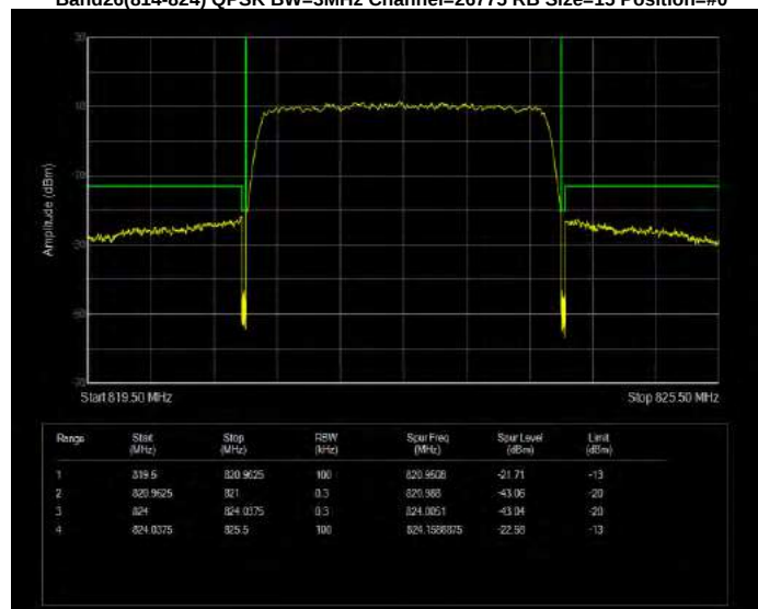
Band26(814-824) QPSK BW=5MHz Channel=26715 RB Size=25 Position=#0
