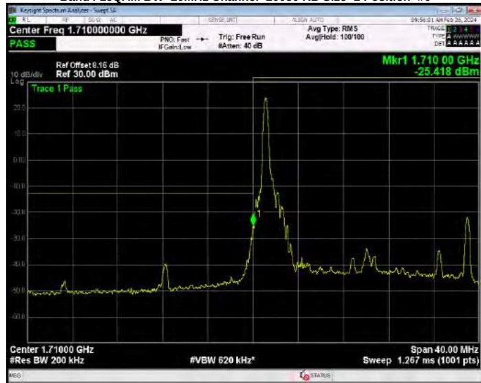
Band4 16QAM BW=20MHz Channel=20050 RB Size=100 Position=#0
