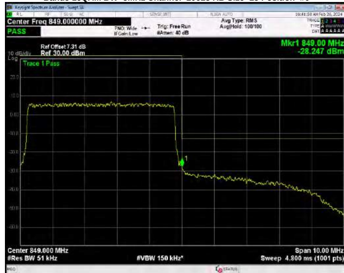
Band5 QPSK BW=1.4MHz Channel=20407 RB Size=1 Position=#0
