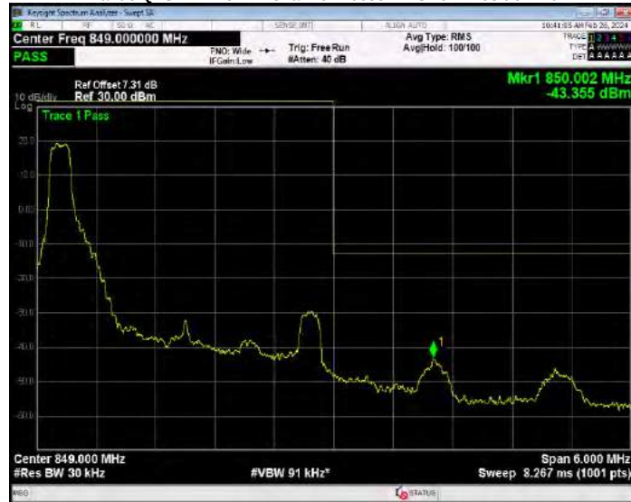
Band5 QPSK BW=3MHz Channel=20635 RB Size=15 Position=#0
