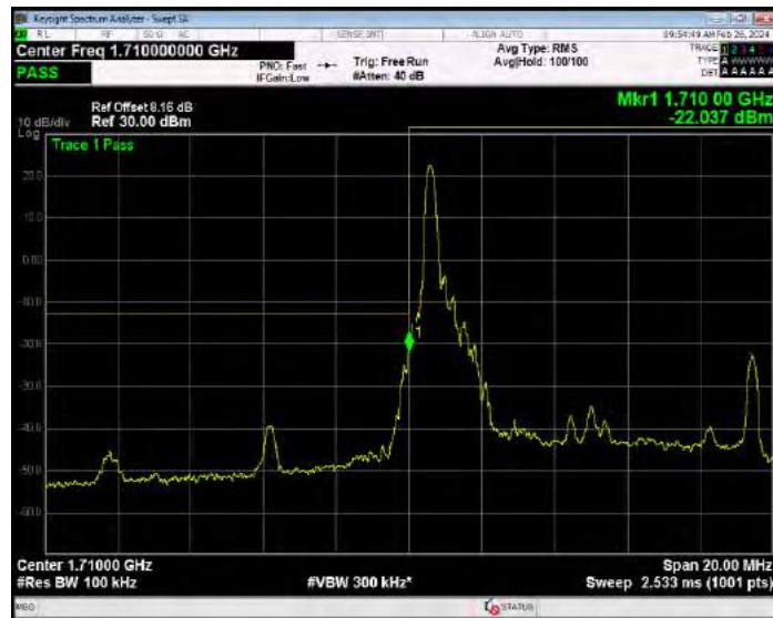
Band4 16QAM BW=10MHz Channel=20000 RB Size=50 Position=#0
