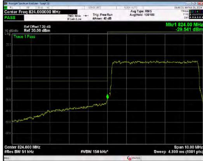
Band5 QPSK BW=5MHz Channel=20625 RB Size=1 Position=#0
