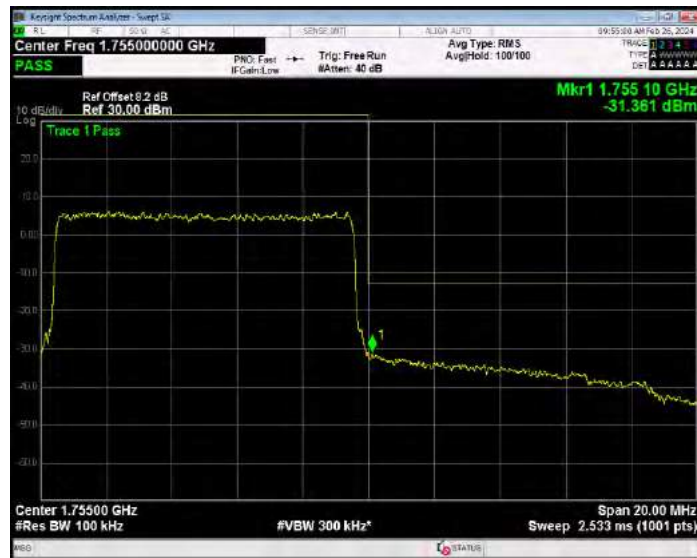
Band4 QPSK BW=15MHz Channel=20025 RB Size=1 Position=#0
