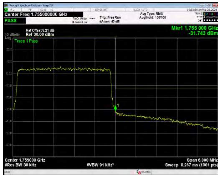
Band4 16QAM BW=5MHz Channel=19975 RB Size=1 Position=#0
