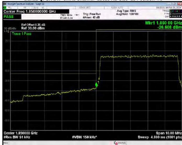
Band2 QPSK BW=5MHz Channel=19175 RB Size=1 Position=#0
