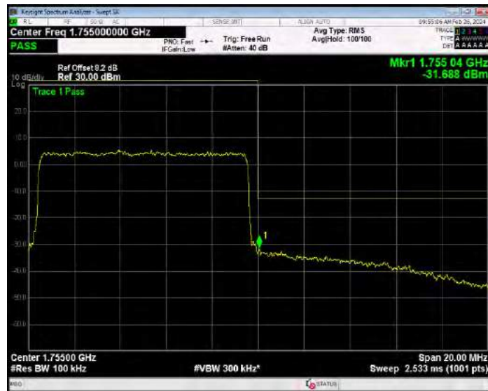
Band4 16QAM BW=15MHz Channel=20025 RB Size=1 Position=#0
