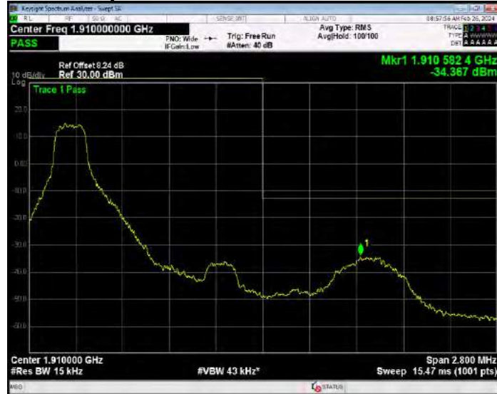
Band2 QPSK BW=1.4MHz Channel=19193 RB Size=6 Position=#0
