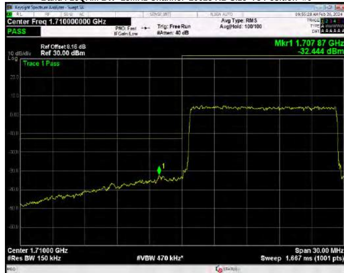
Band4 16QAM BW=15MHz Channel=20325 RB Size=1 Position=#0
