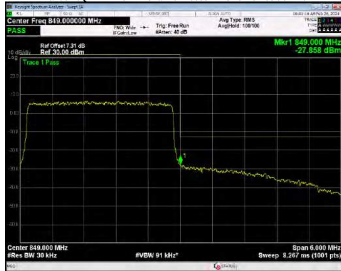
Band5 16QAM BW=5MHz Channel=20425 RB Size=1 Position=#0
