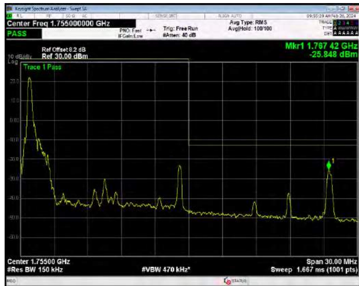
Band4 16QAM BW=15MHz Channel=20325 RB Size=75 Position=#0
