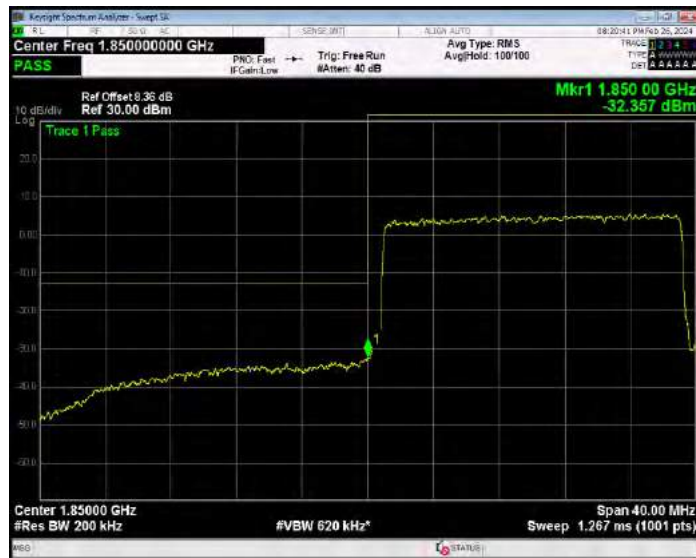
Band25 16QAM BW=20MHz Channel=26590 RB Size=100 Position=#0
