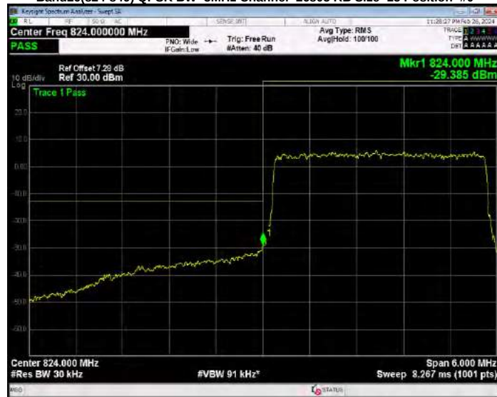
Band26(824-849) QPSK BW=3MHz Channel=27025 RB Size=15 Position=#0
