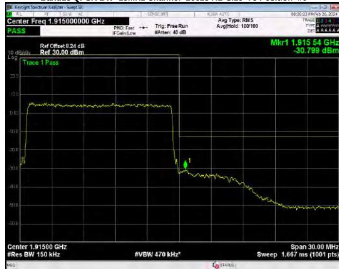
Band25 QPSK BW=20MHz Channel=26140 RB Size=100 Position=#0
