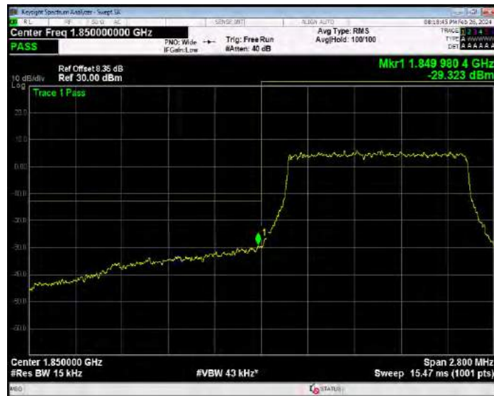
Band25 16QAM BW=1.4MHz Channel=26683 RB Size=6 Position=#0
