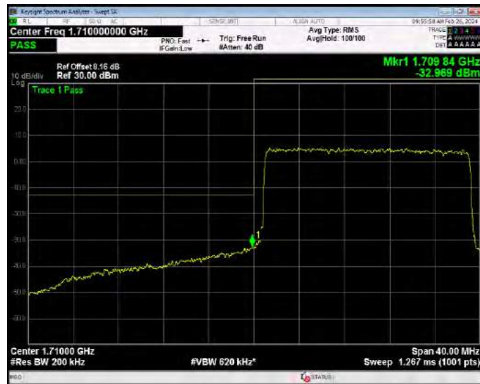
Band4 QPSK BW=20MHz Channel=20300 RB Size=1 Position=#0
