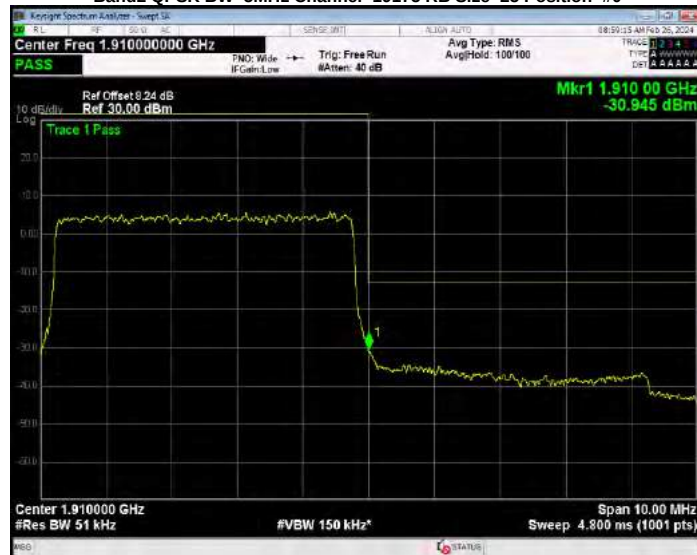
Band4 16QAM BW=1.4MHz Channel=19957 RB Size=1 Position=#0
