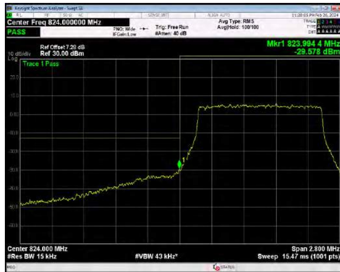
Band26(824-849) 16QAM BW=1.4MHz Channel=27033 RB Size=6 Position=#0
