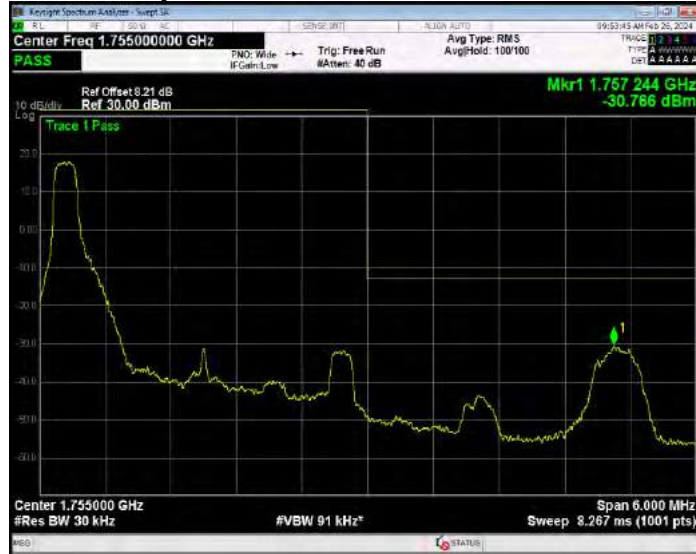
Band4 QPSK BW=3MHz Channel=20385 RB Size=15 Position=#0
