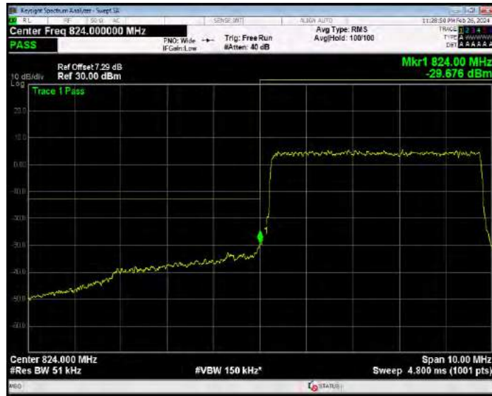
Band26(824-849) QPSK BW=5MHz Channel=27015 RB Size=25 Position=#0
