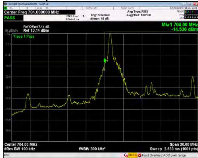
Band17 QPSK BW=10MHz Channel=23780 RB Size=50 Position=#0
