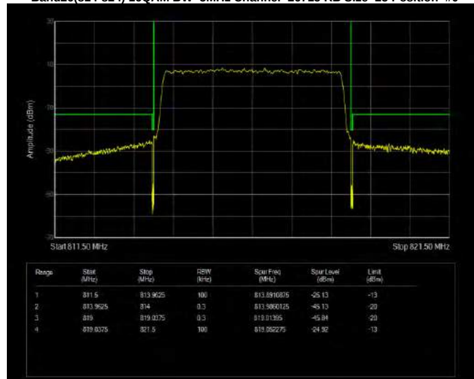
Band26(814-824) 16QAM BW=5MHz Channel=26765 RB Size=25 Position=#0
