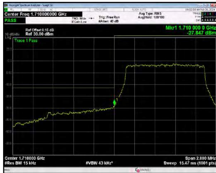
Band4 QPSK BW=1.4MHz Channel=20393 RB Size=1 Position=#0
