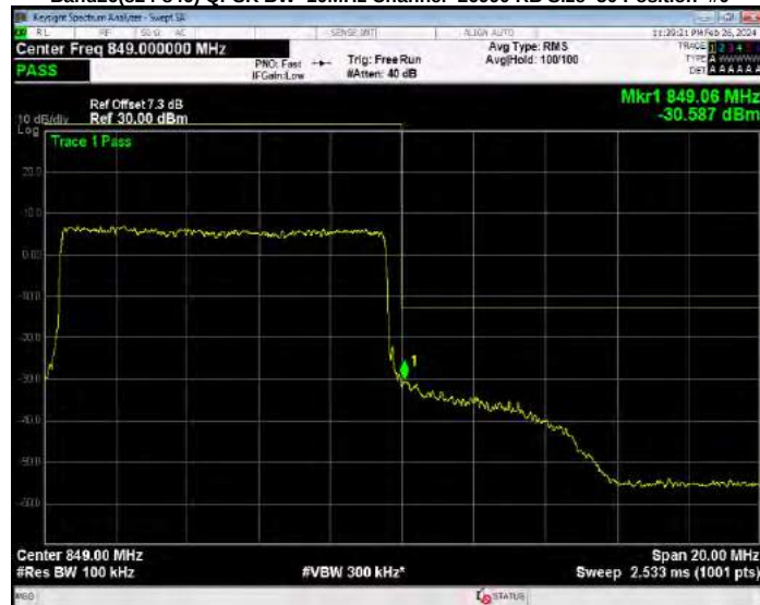
Band26(824-849) QPSK BW=15MHz Channel=26865 RB Size=75 Position=#0
