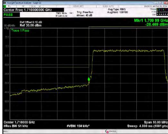
Band4 QPSK BW=5MHz Channel=20375 RB Size=1 Position=#0
