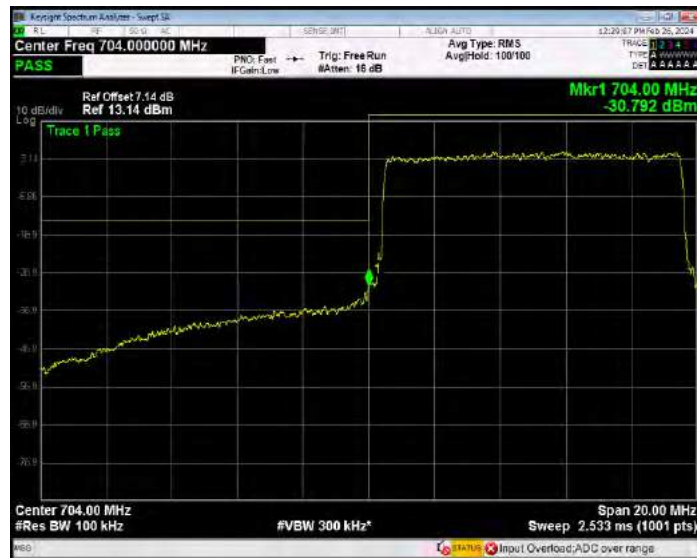
Band17 16QAM BW=10MHz Channel=23800 RB Size=1 Position=#0
