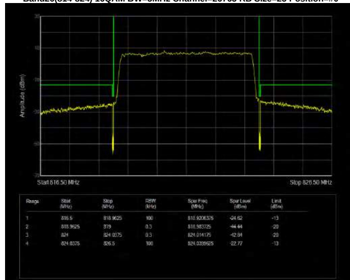
Band26(814-824) QPSK BW=1.4MHz Channel=26697 RB Size=6 Position=#0
