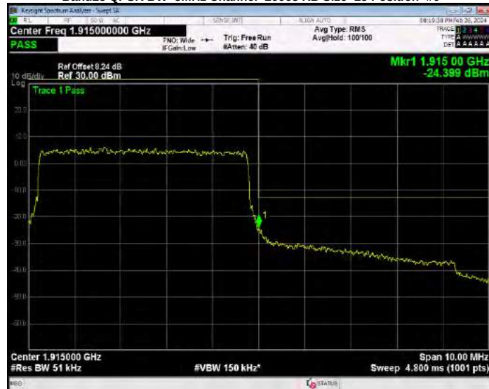
Band26(824-849) 16QAM BW=1.4MHz Channel=26797 RB Size=6 Position=#0
