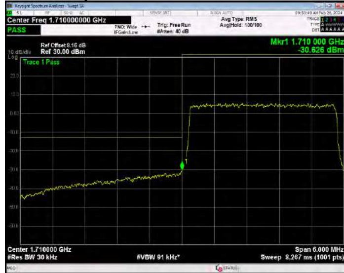
Band4 16QAM BW=3MHz Channel=20385 RB Size=1 Position=#0
