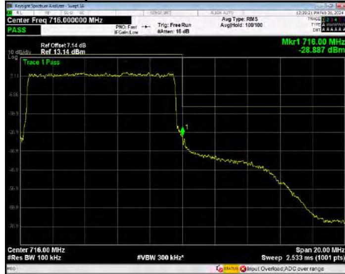
Band17 16QAM BW=5MHz Channel=23755 RB Size=1 Position=#0
