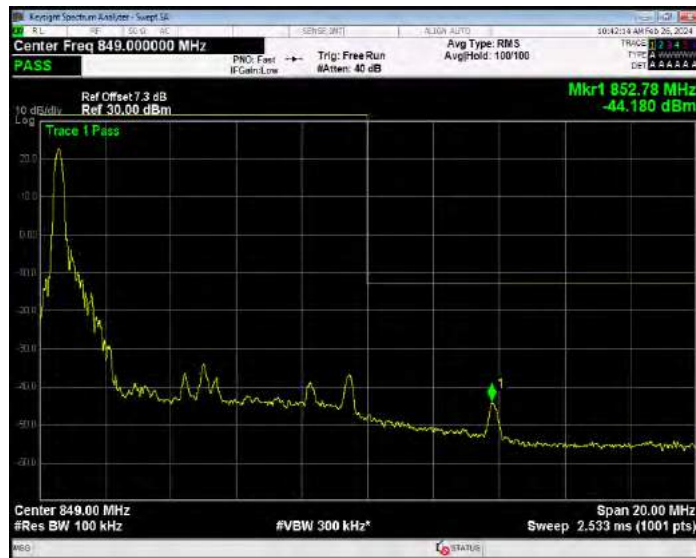
Band5 QPSK BW=10MHz Channel=20600 RB Size=50 Position=#0
