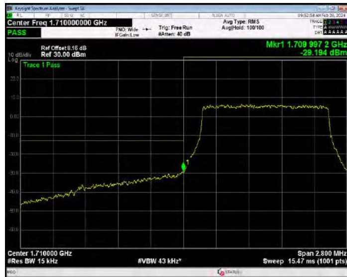
Band4 16QAM BW=1.4MHz Channel=20393 RB Size=1 Position=#0
