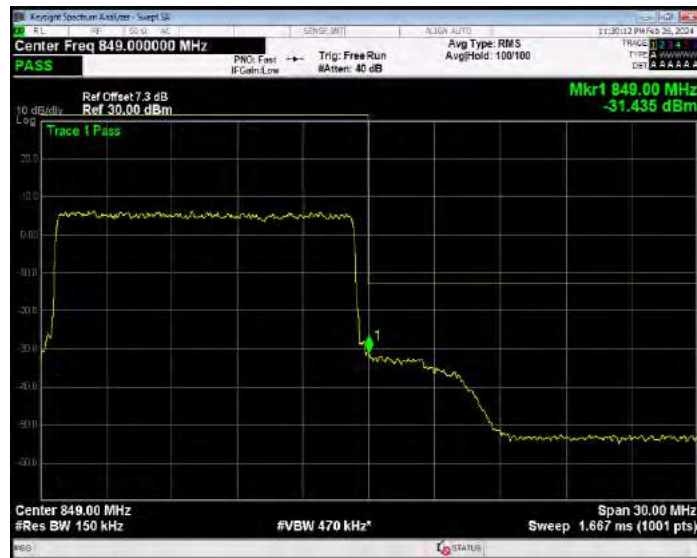
Band26(824-849) QPSK BW=3MHz Channel=26805 RB Size=15 Position=#0
