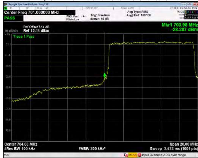
Band17 QPSK BW=10MHz Channel=23800 RB Size=1 Position=#0
