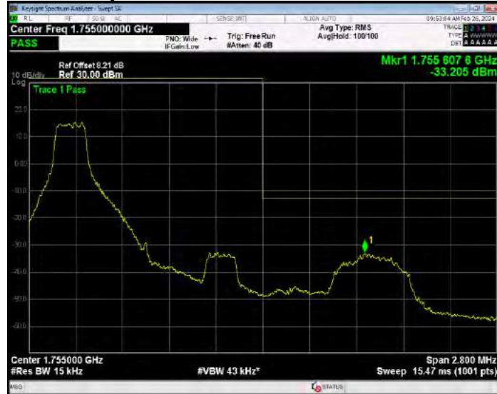
Band4 QPSK BW=1.4MHz Channel=20393 RB Size=6 Position=#0
