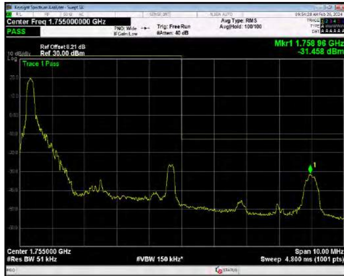
Band4 16QAM BW=5MHz Channel=20375 RB Size=25 Position=#0
