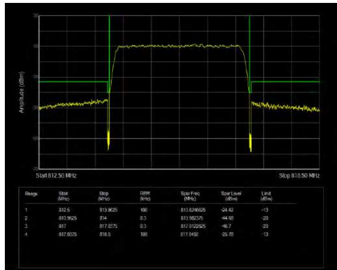
Band26(814-824) QPSK BW=3MHz Channel=26775 RB Size=15 Position=#0
