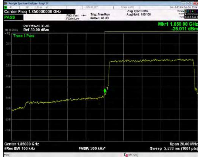
Band25 QPSK BW=10MHz Channel=26640 RB Size=50 Position=#0
