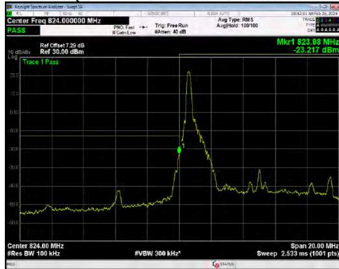
Band5 QPSK BW=10MHz Channel=20450 RB Size=50 Position=#0
