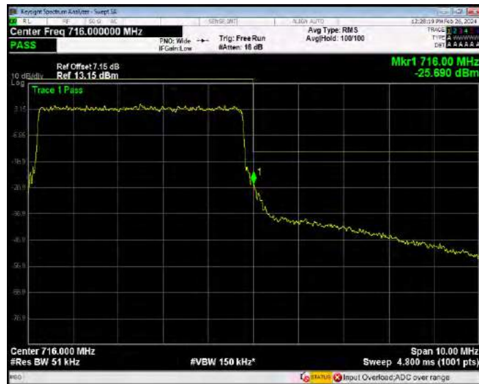
Band17 QPSK BW=10MHz Channel=23780 RB Size=1 Position=#0
