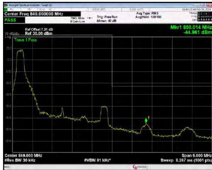
Band5 16QAM BW=3MHz Channel=20635 RB Size=15 Position=#0
