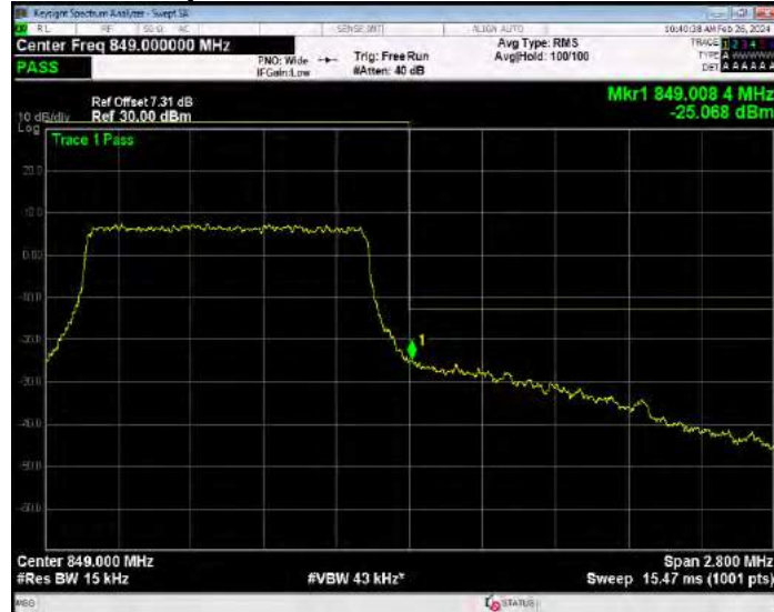
Band5 16QAM BW=10MHz Channel=20450 RB Size=1 Position=#0
