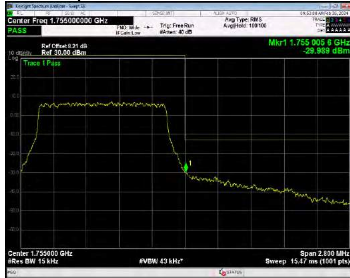
Band4 QPSK BW=10MHz Channel=20000 RB Size=1 Position=#0
