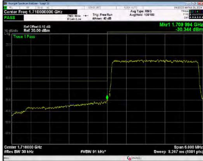
Band4 QPSK BW=3MHz Channel=20385 RB Size=1 Position=#0
