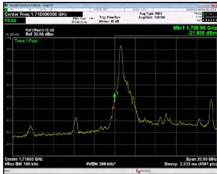
Band4 QPSK BW=10MHz Channel=20000 RB Size=50 Position=#0
