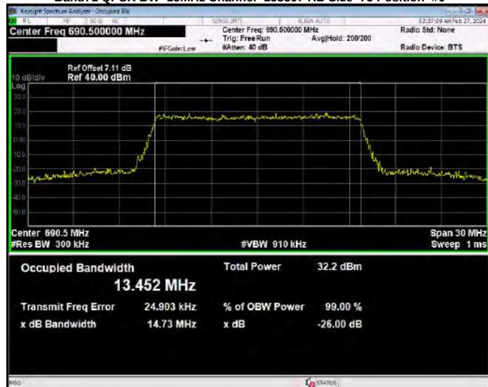
Band71 QPSK BW=20MHz Channel=133222 RB Size=100 Position=#0
