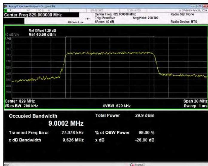
Band26(824-849) 16QAM BW=10MHz Channel=26915 RB Size=50 Position=#0
