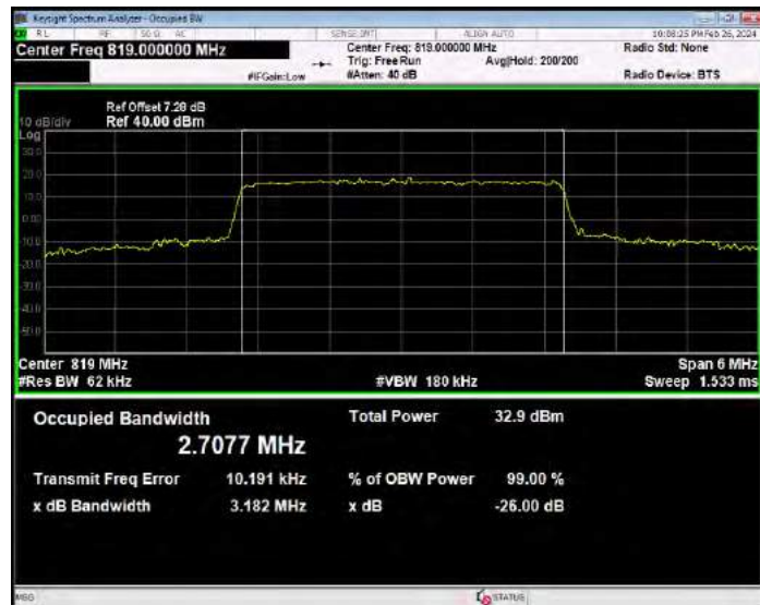
Band26(814-824) QPSK BW=3MHz Channel=26775 RB Size=15 Position=#0
