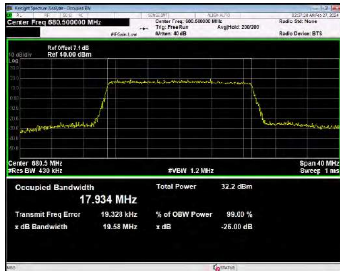
Band71 QPSK BW=20MHz Channel=133372 RB Size=100 Position=#0
