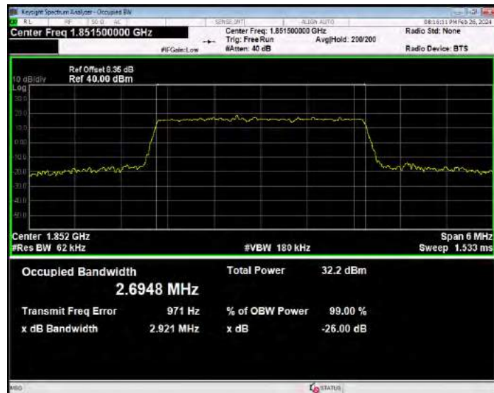
Band25 QPSK BW=3MHz Channel=26365 RB Size=15 Position=#0
