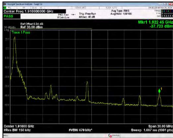
Band2 16QAM BW=15MHz Channel=19125 RB Size=75 Position=#0
