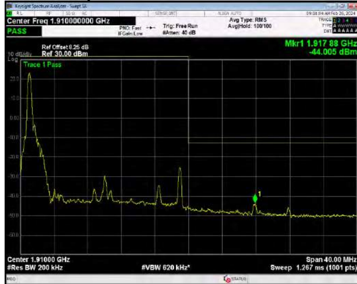
Band2 16QAM BW=20MHz Channel=19100 RB Size=100 Position=#0
