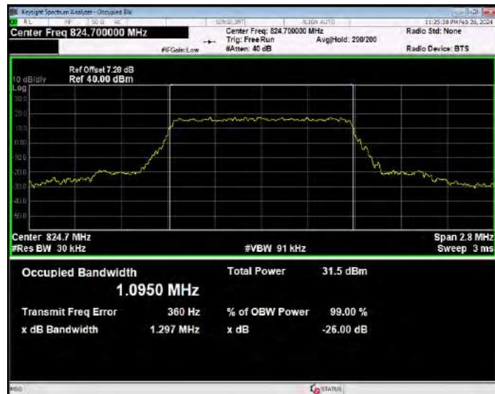
Band26(824-849) QPSK BW=1.4MHz Channel=26915 RB Size=6 Position=#0
