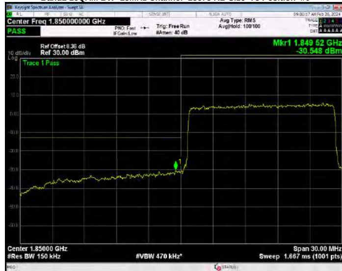
Band2 16QAM BW=15MHz Channel=19125 RB Size=1 Position=#0
