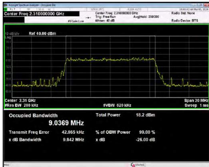
Band40(2305-2315) QPSK BW=5MHz Channel=38725 RB Size=25 Position=#0
