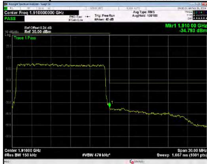
Band2 16QAM BW=20MHz Channel=18700 RB Size=1 Position=#0
