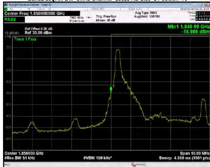
Band2 16QAM BW=5MHz Channel=18625 RB Size=25 Position=#0
