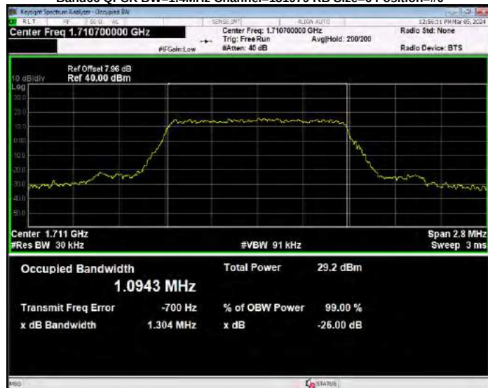
Band66 QPSK BW=1.4MHz Channel=132322 RB Size=6 Position=#0
