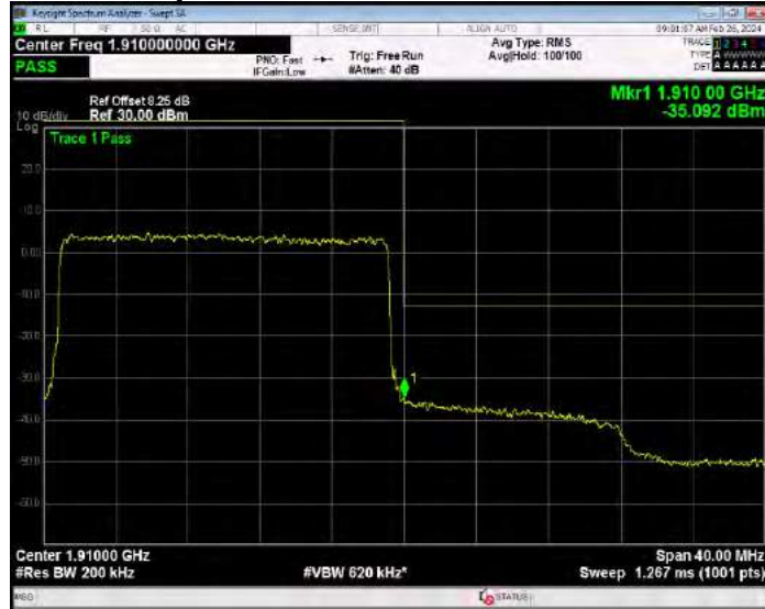
Band2 16QAM BW=3MHz Channel=18615 RB Size=1 Position=#0
