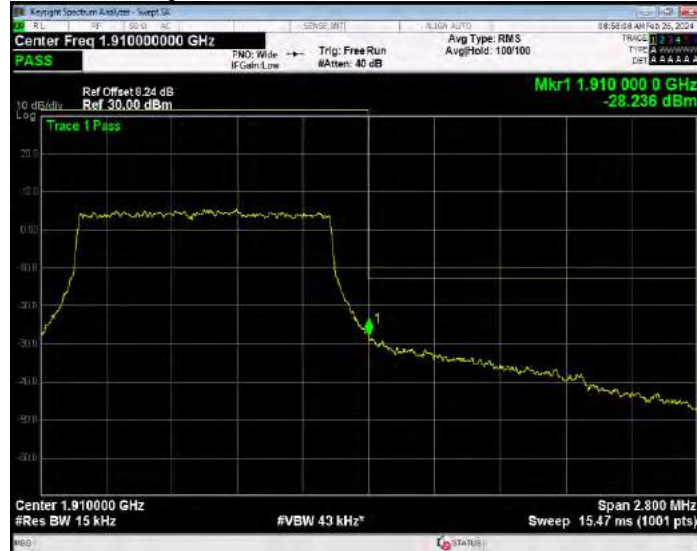
Band2 16QAM BW=10MHz Channel=18650 RB Size=1 Position=#0
