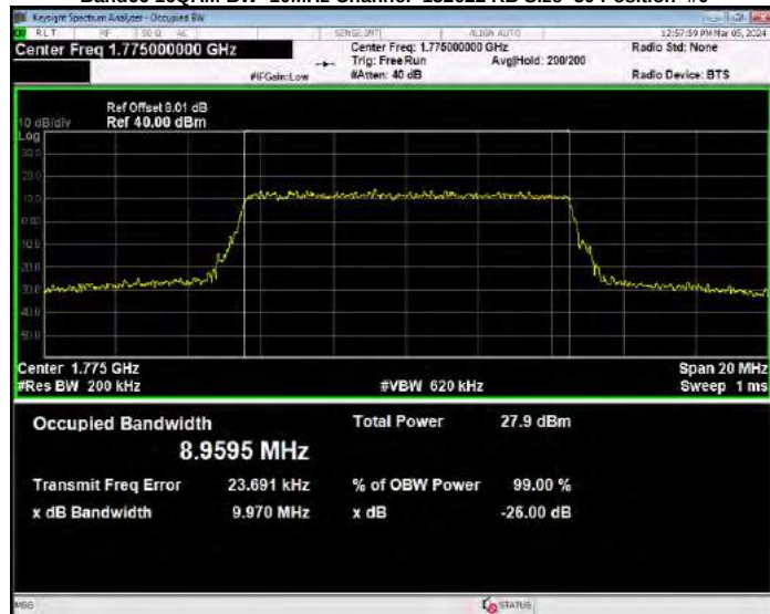
Band66 16QAM BW=15MHz Channel=132047 RB Size=75 Position=#0
