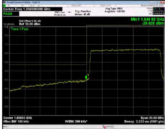
Band2 16QAM BW=10MHz Channel=19150 RB Size=1 Position=#0
