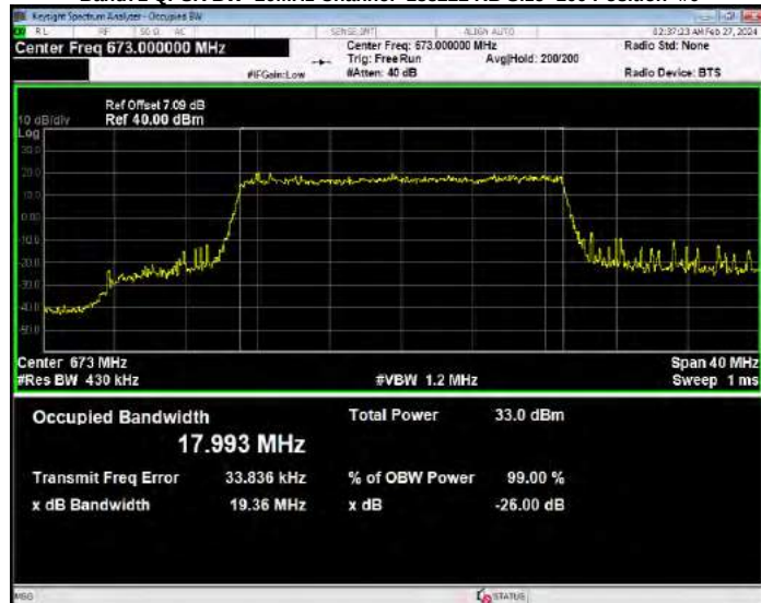
Band71 QPSK BW=20MHz Channel=133297 RB Size=100 Position=#0
