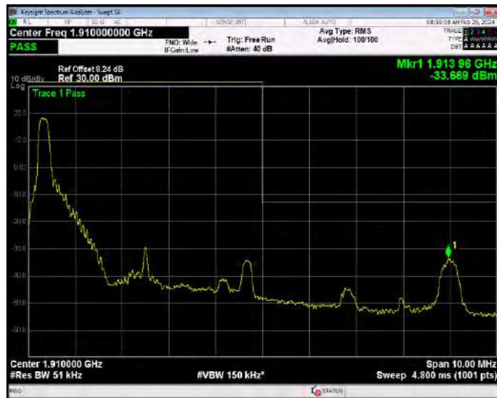
Band2 16QAM BW=5MHz Channel=19175 RB Size=25 Position=#0
