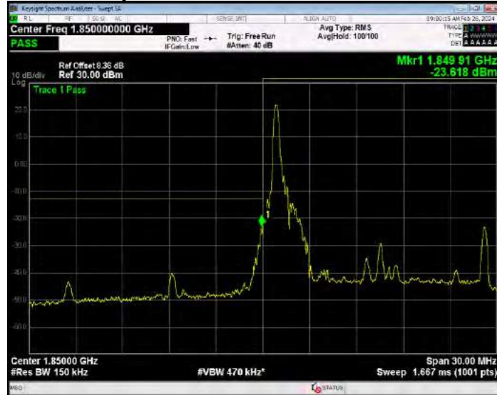
Band2 16QAM BW=15MHz Channel=18675 RB Size=75 Position=#0
