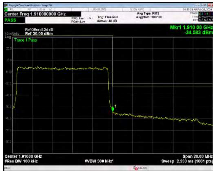
Band2 16QAM BW=15MHz Channel=18675 RB Size=1 Position=#0
