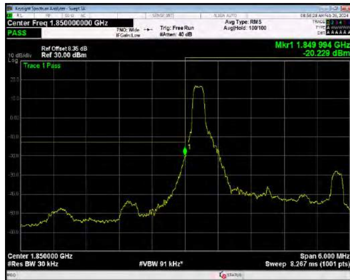
Band2 16QAM BW=3MHz Channel=18615 RB Size=15 Position=#0
