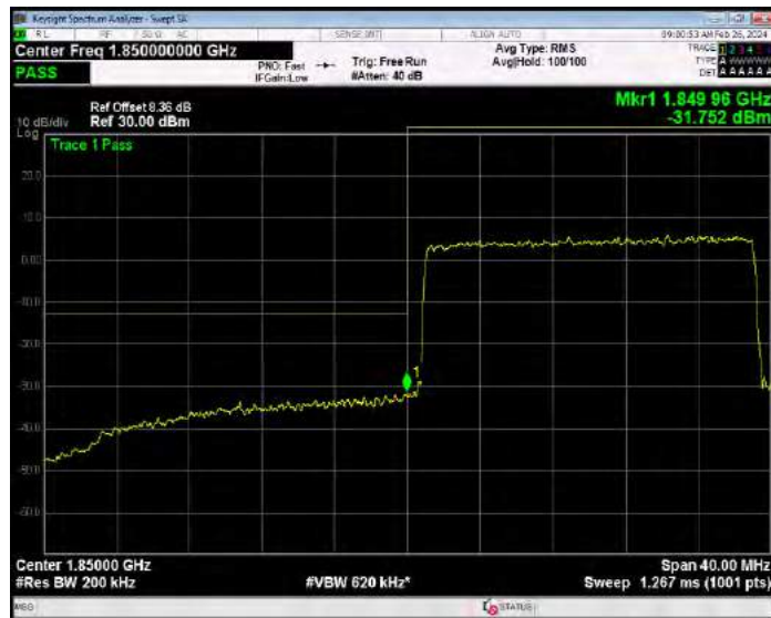
Band2 16QAM BW=20MHz Channel=19100 RB Size=1 Position=#0
