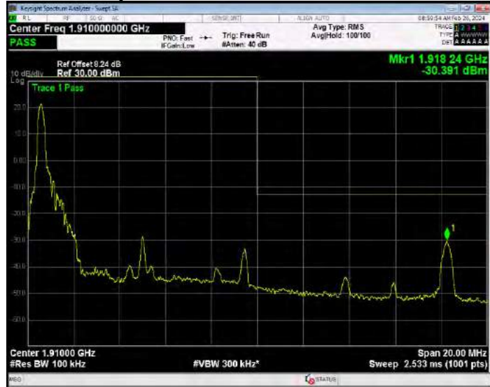
Band2 16QAM BW=10MHz Channel=19150 RB Size=50 Position=#0
