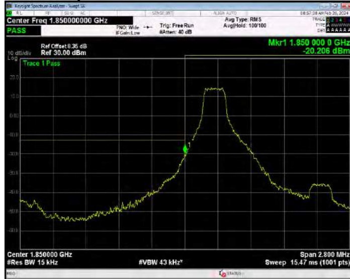
Band2 QPSK BW=1.4MHz Channel=18607 RB Size=6 Position=#0
