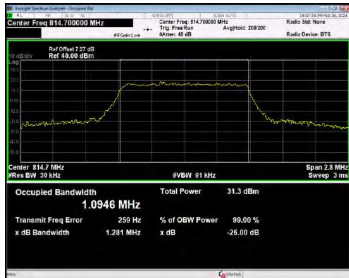
Band26(814-824) 16QAM BW=1.4MHz Channel=26740 RB Size=6 Position=#0
