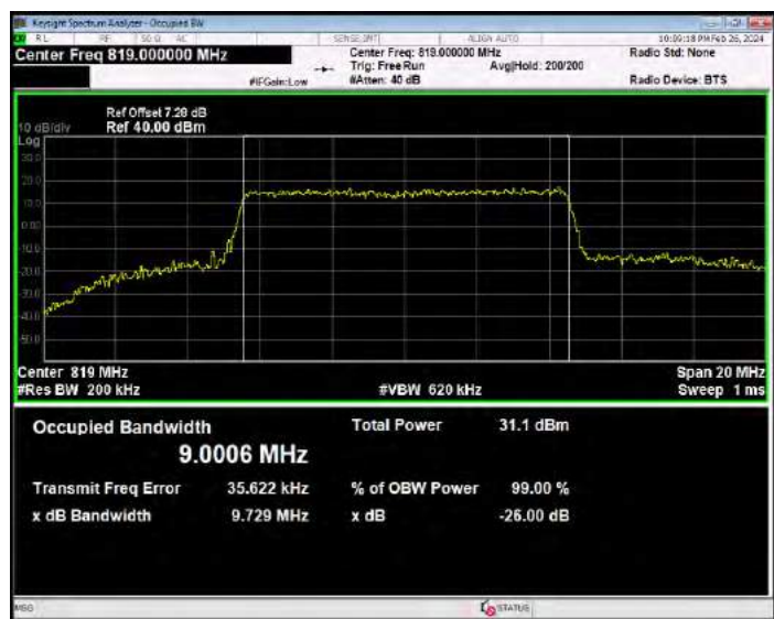
Band26(814-824) 16QAM BW=3MHz Channel=26705 RB Size=15 Position=#0
