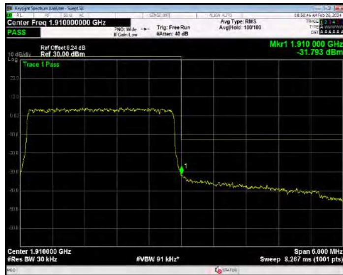
Band2 16QAM BW=5MHz Channel=18625 RB Size=1 Position=#0
