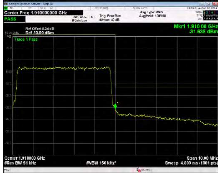
Band2 QPSK BW=1.4MHz Channel=18607 RB Size=1 Position=#0
