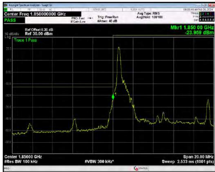
Band2 16QAM BW=10MHz Channel=18650 RB Size=50 Position=#0
