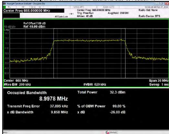
Band71 16QAM BW=10MHz Channel=133297 RB Size=50 Position=#0
