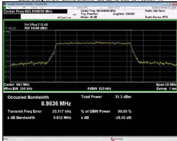
Band71 16QAM BW=15MHz Channel=133197 RB Size=75 Position=#0
