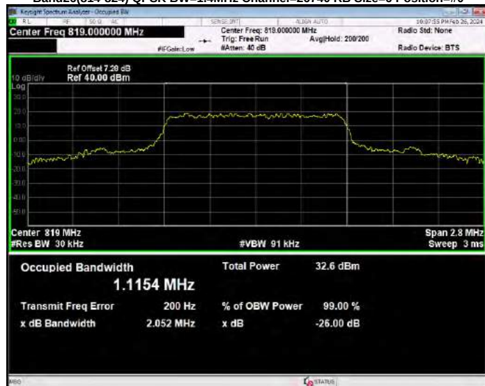
Band26(814-824) QPSK BW=1.4MHz Channel=26783 RB Size=6 Position=#0
