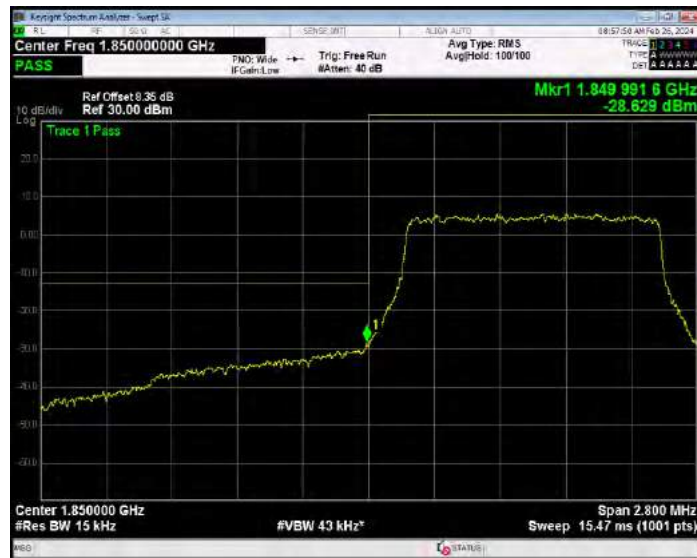
Band2 16QAM BW=1.4MHz Channel=19193 RB Size=1 Position=#0
