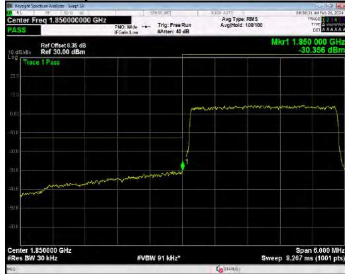
Band2 16QAM BW=3MHz Channel=19185 RB Size=1 Position=#0
