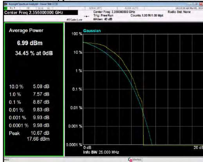
Band40(2350-2360) QPSK BW=5MHz Channel=39225 RB Size=1 Position=#0
