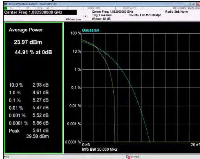
Band25 16QAM BW=3MHz Channel=26675 RB Size=1 Position=#0
