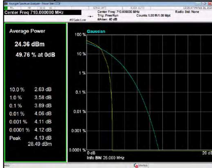
Band17 16QAM BW=10MHz Channel=23800 RB Size=1 Position=#0
