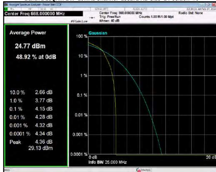
Band71 16QAM BW=10MHz Channel=133297 RB Size=1 Position=#0
