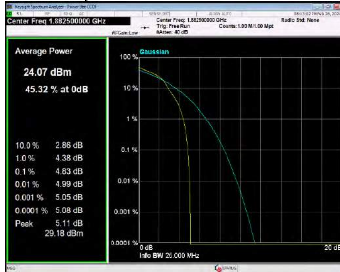
Band25 16QAM BW=1.4MHz Channel=26683 RB Size=1 Position=#0
