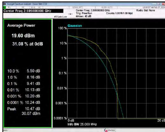
Band38 16QAM BW=20MHz Channel=38150 RB Size=1 Position=#0
