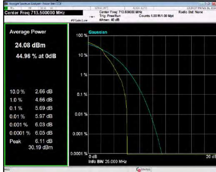
Band17 QPSK BW=10MHz Channel=23780 RB Size=1 Position=#0
