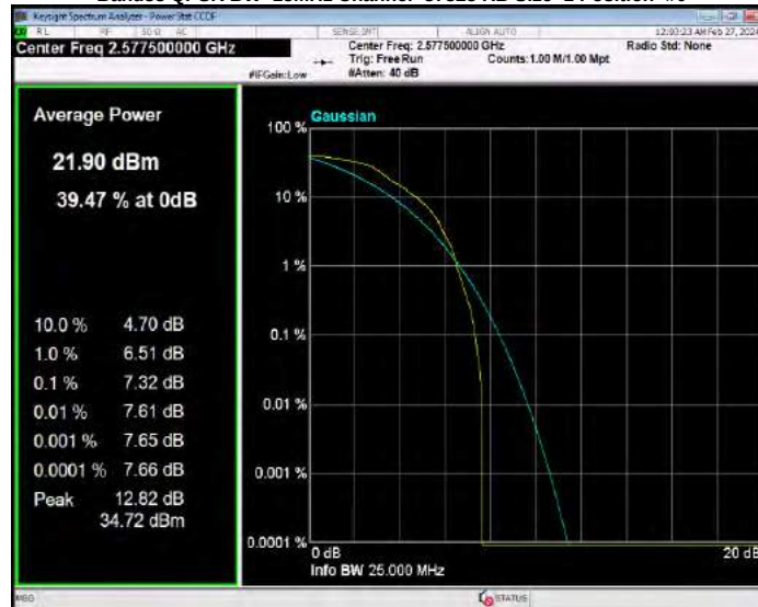
Band38 QPSK BW=15MHz Channel=38000 RB Size=1 Position=#0
