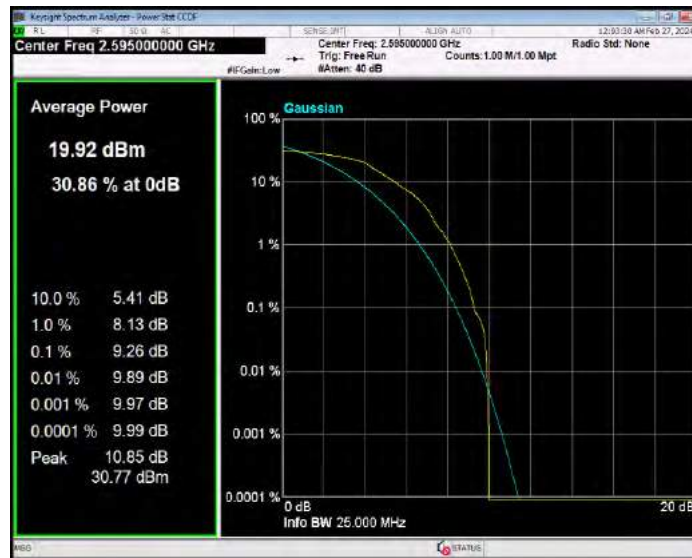
Band38 QPSK BW=15MHz Channel=38175 RB Size=1 Position=#0
