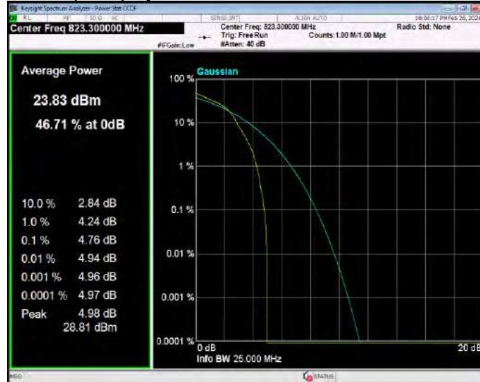
Band26(814-824) 16QAM BW=10MHz Channel=26740 RB Size=1 Position=#0
