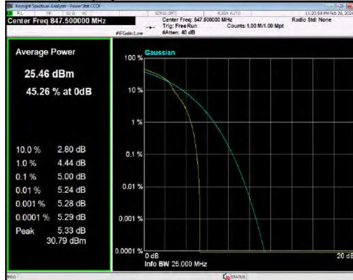
Band26(824-849) 16QAM BW=5MHz Channel=26815 RB Size=1 Position=#0
