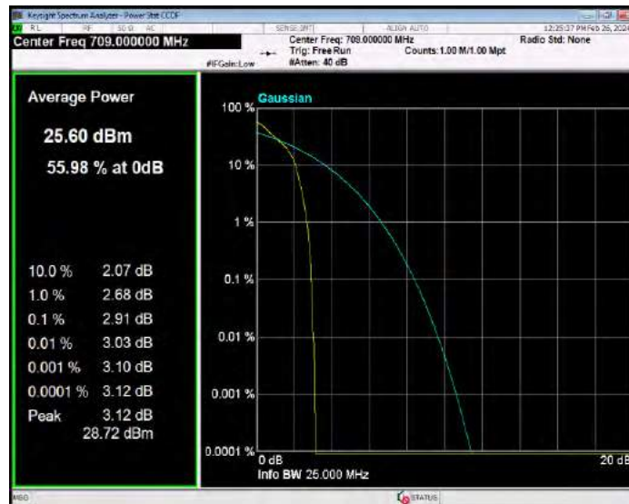
Band17 QPSK BW=10MHz Channel=23790 RB Size=1 Position=#0
