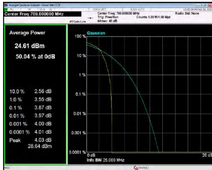
Band17 16QAM BW=10MHz Channel=23790 RB Size=1 Position=#0
