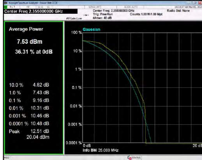
Band40(2350-2360) QPSK BW=5MHz Channel=39175 RB Size=1 Position=#0
