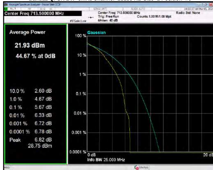
Band17 16QAM BW=10MHz Channel=23780 RB Size=1 Position=#0
