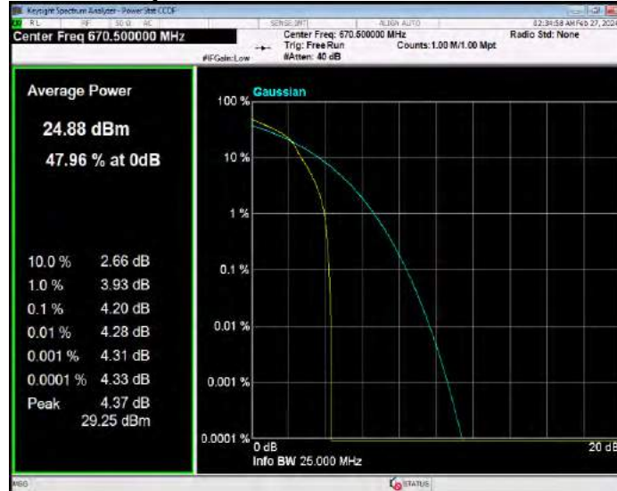
Band71 16QAM BW=15MHz Channel=133297 RB Size=1 Position=#0
