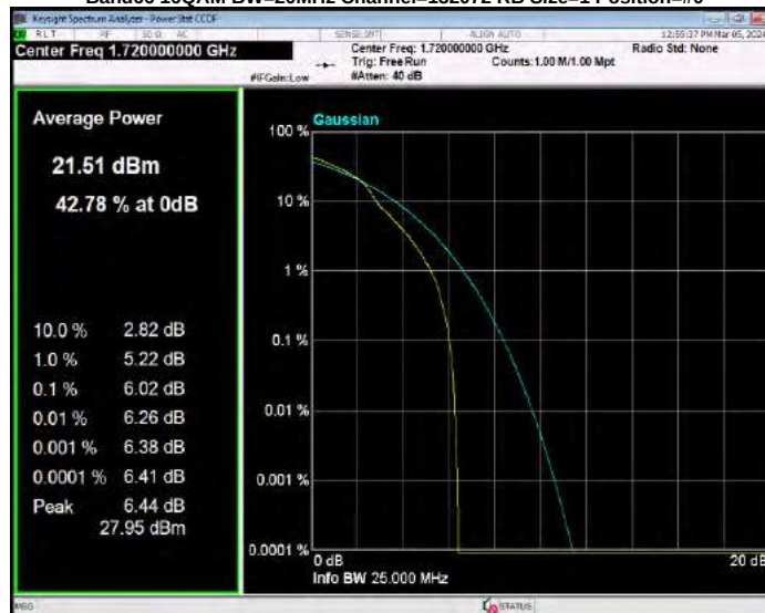
Band66 16QAM BW=20MHz Channel=132322 RB Size=1 Position=#0
