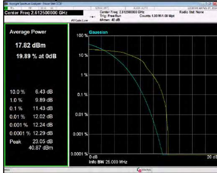
Band38 16QAM BW=20MHz Channel=37850 RB Size=1 Position=#0
