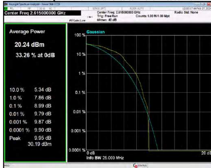
Band38 16QAM BW=15MHz Channel=37825 RB Size=1 Position=#0
