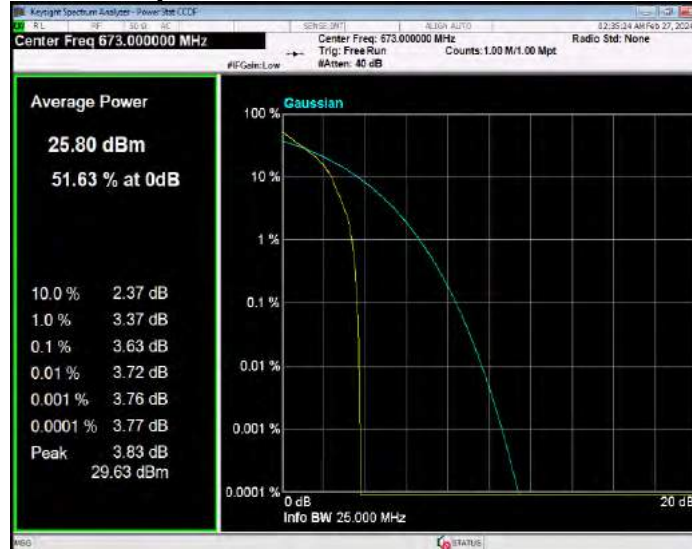
Band71 QPSK BW=20MHz Channel=133297 RB Size=1 Position=#0
