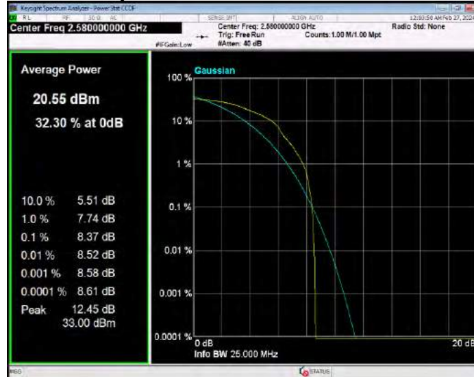
Band38 16QAM BW=20MHz Channel=38000 RB Size=1 Position=#0
