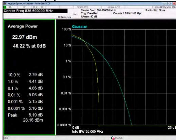
Band26(824-849) 16QAM BW=10MHz Channel=26990 RB Size=1 Position=#0
