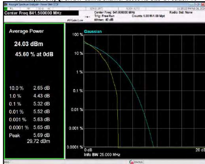
Band26(824-849) QPSK BW=3MHz Channel=26805 RB Size=1 Position=#0
