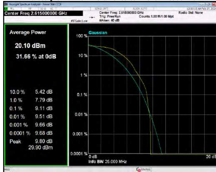
Band38 QPSK BW=15MHz Channel=37825 RB Size=1 Position=#0
