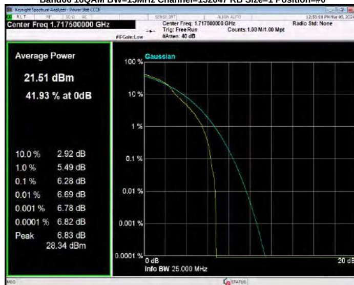
Band66 16QAM BW=15MHz Channel=132322 RB Size=1 Position=#0
