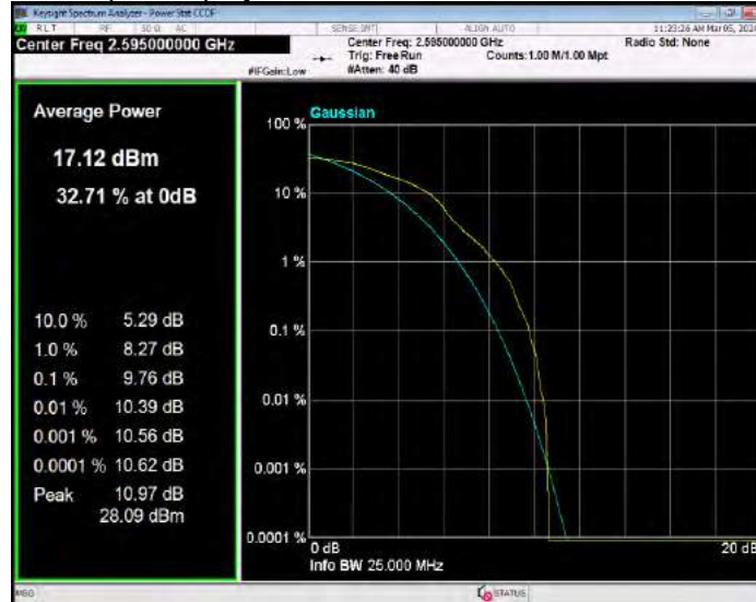
Band41(2535-2655) 16QAM BW=20MHz Channel=40640 RB Size=1 Position=#0
