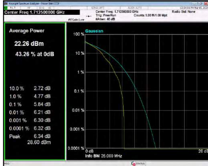
Band66 QPSK BW=5MHz Channel=132322 RB Size=1 Position=#0
