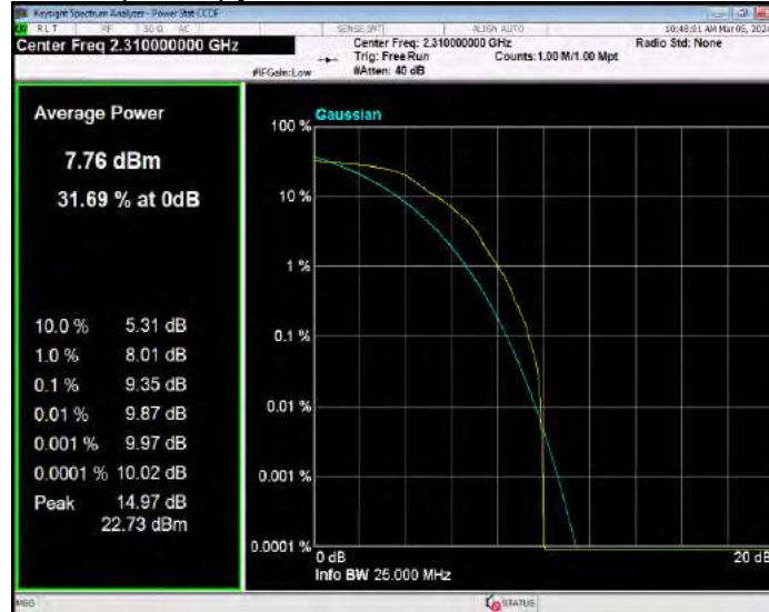
Band40(2305-2315) QPSK BW=5MHz Channel=38775 RB Size=1 Position=#0
