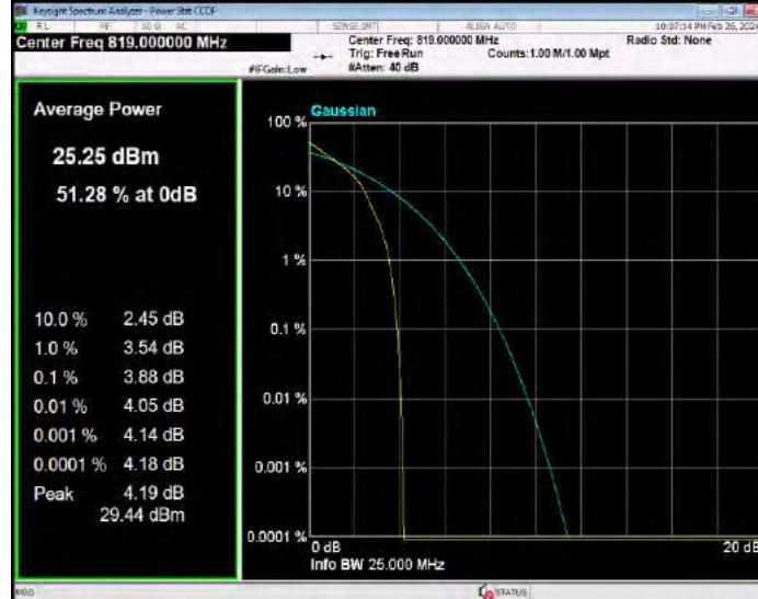
Band26(814-824) QPSK BW=3MHz Channel=26705 RB Size=1 Position=#0
