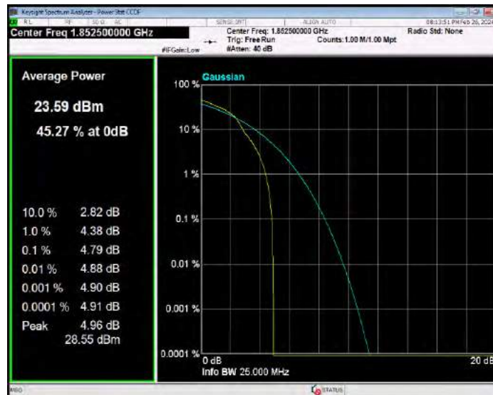
Band25 16QAM BW=5MHz Channel=26365 RB Size=1 Position=#0
