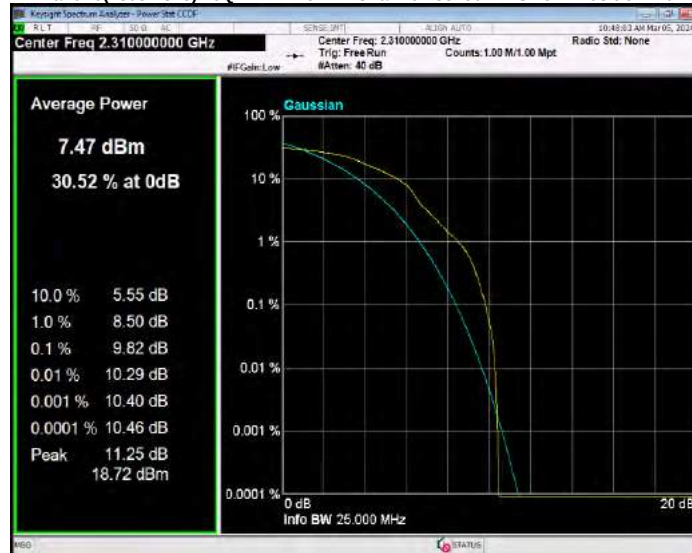
Band40(2305-2315) 16QAM BW=5MHz Channel=38775 RB Size=1 Position=#0
