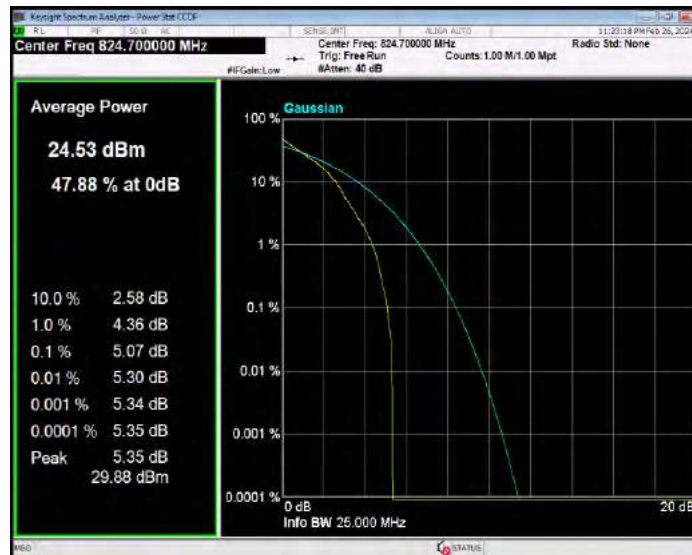
Band26(824-849) QPSK BW=1.4MHz Channel=26915 RB Size=1 Position=#0
