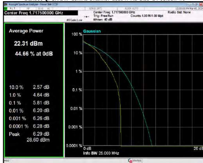
Band66 QPSK BW=15MHz Channel=132322 RB Size=1 Position=#0
