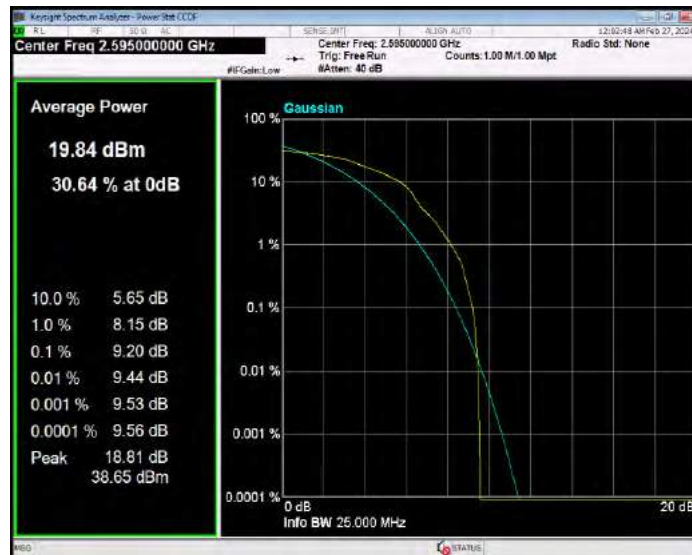
Band38 16QAM BW=5MHz Channel=38225 RB Size=1 Position=#0
