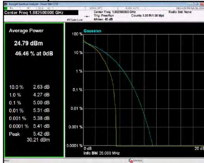
Band25 QPSK BW=10MHz Channel=26640 RB Size=1 Position=#0
