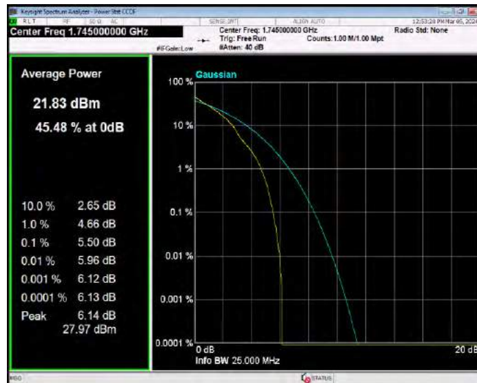
Band66 QPSK BW=1.4MHz Channel=132665 RB Size=1 Position=#0
