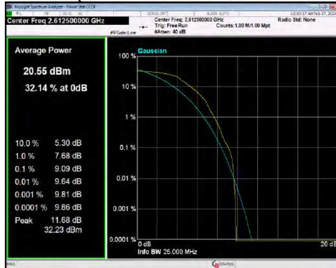
Band38 QPSK BW=20MHz Channel=37850 RB Size=1 Position=#0
