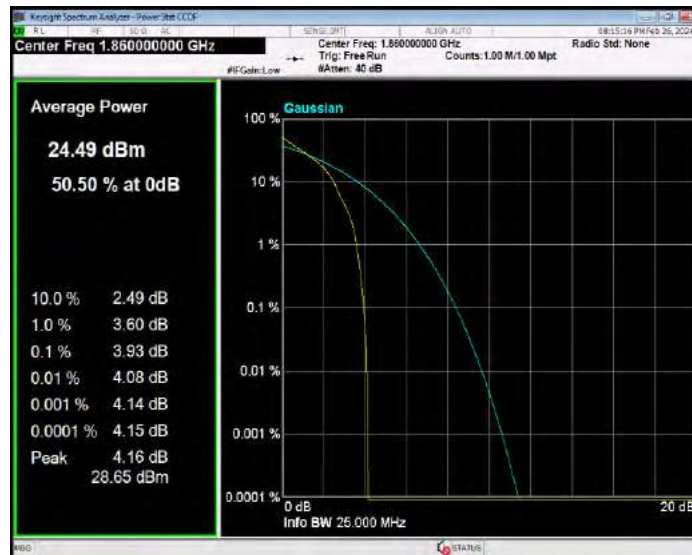
Band25 QPSK BW=20MHz Channel=26365 RB Size=1 Position=#0
