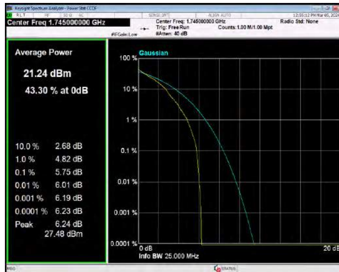
Band66 QPSK BW=15MHz Channel=132597 RB Size=1 Position=#0
