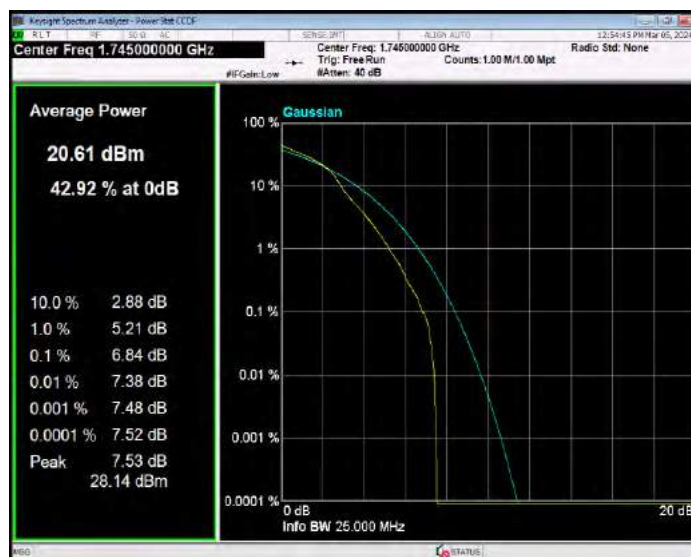
Band66 16QAM BW=10MHz Channel=132622 RB Size=1 Position=#0
