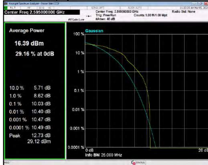
Band41(2535-2655) 16QAM BW=5MHz Channel=40640 RB Size=1 Position=#0
