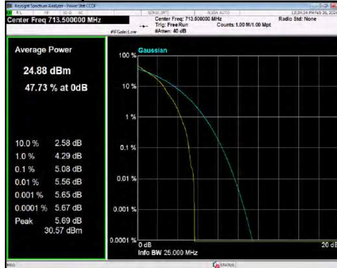
Band25 16QAM BW=1.4MHz Channel=26047 RB Size=1 Position=#0
