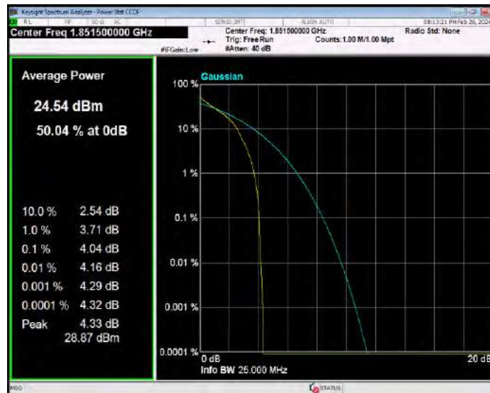
Band25 QPSK BW=3MHz Channel=26365 RB Size=1 Position=#0
