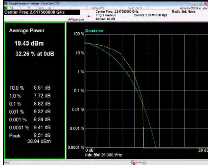
Band38 QPSK BW=10MHz Channel=37800 RB Size=1 Position=#0
