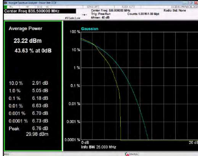
Band26(824-849) 16QAM BW=3MHz Channel=27025 RB Size=1 Position=#0
