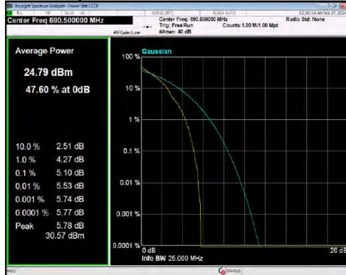
Band71 QPSK BW=20MHz Channel=133222 RB Size=1 Position=#0
