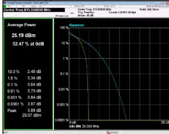
Band26(814-824) QPSK BW=3MHz Channel=26740 RB Size=1 Position=#0
