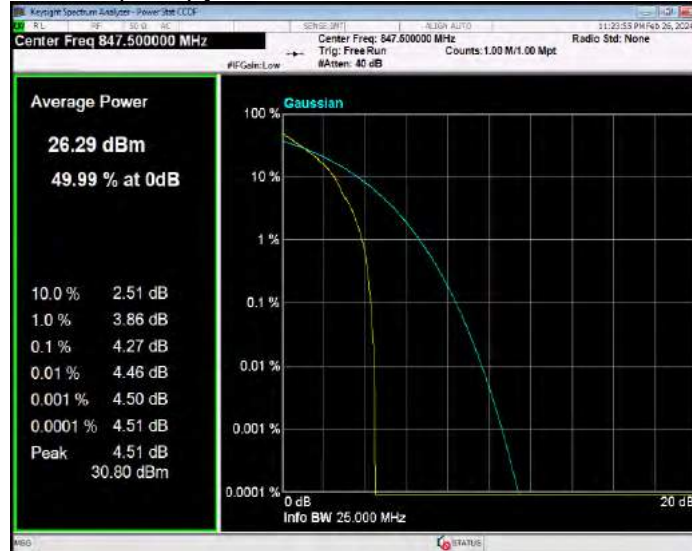
Band26(824-849) QPSK BW=5MHz Channel=26815 RB Size=1 Position=#0
