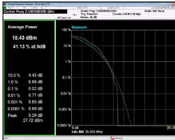
Band41(2535-2655) QPSK BW=5MHz Channel=40640 RB Size=1 Position=#0
