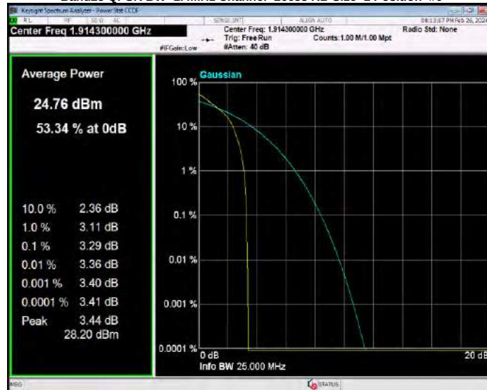
Band25 QPSK BW=10MHz Channel=26090 RB Size=1 Position=#0
