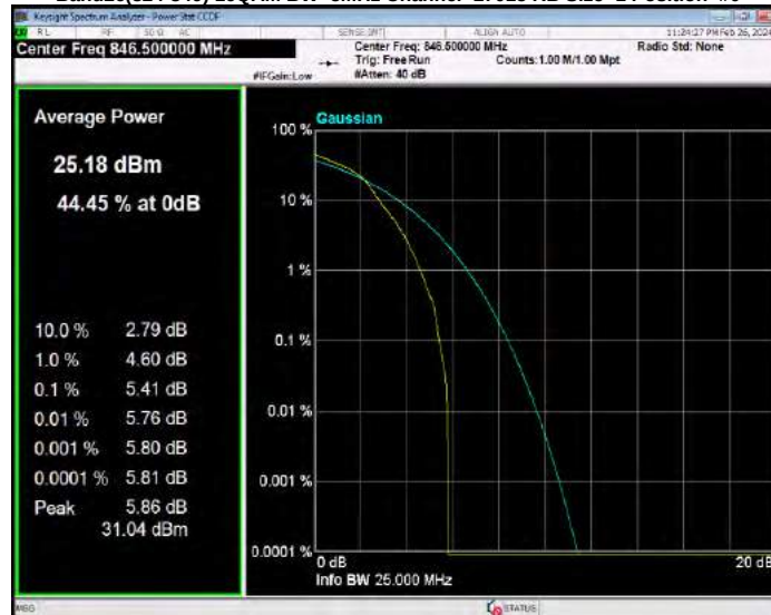
Band26(824-849) QPSK BW=1.4MHz Channel=26797 RB Size=1 Position=#0
