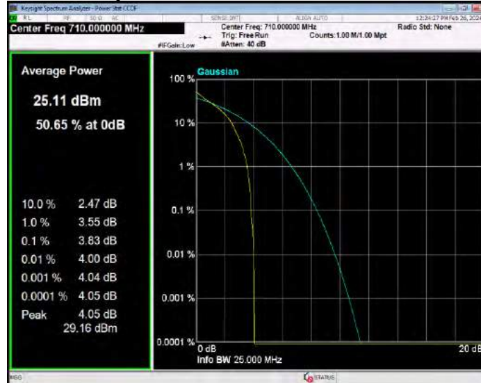
Band17 QPSK BW=5MHz Channel=23825 RB Size=1 Position=#0
