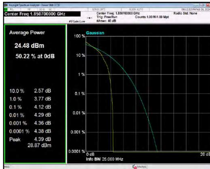
Band25 QPSK BW=1.4MHz Channel=26365 RB Size=1 Position=#0
