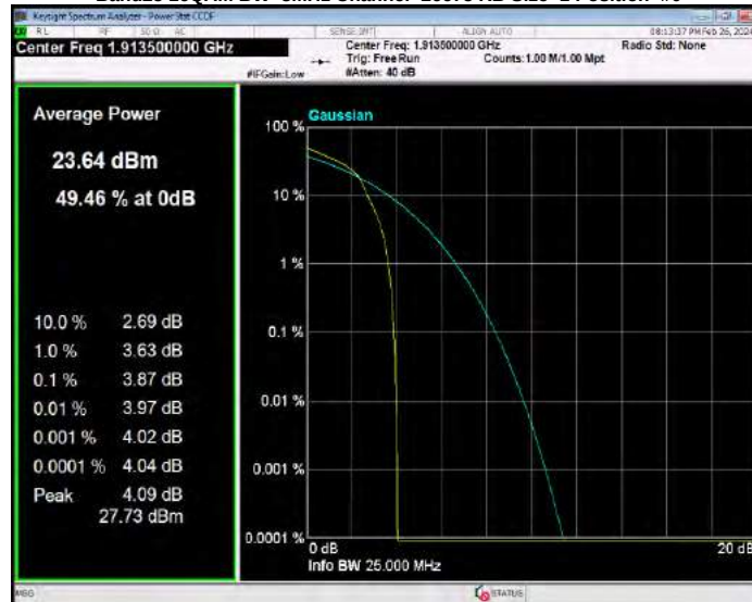
Band25 16QAM BW=5MHz Channel=26065 RB Size=1 Position=#0
