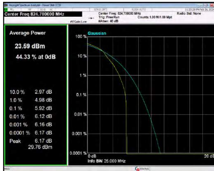
Band26(824-849) 16QAM BW=1.4MHz Channel=26915 RB Size=1 Position=#0
