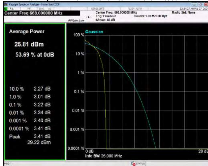
Band71 QPSK BW=10MHz Channel=133297 RB Size=1 Position=#0
