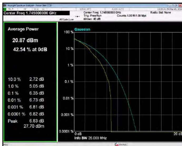
Band66 QPSK BW=20MHz Channel=132572 RB Size=1 Position=#0
