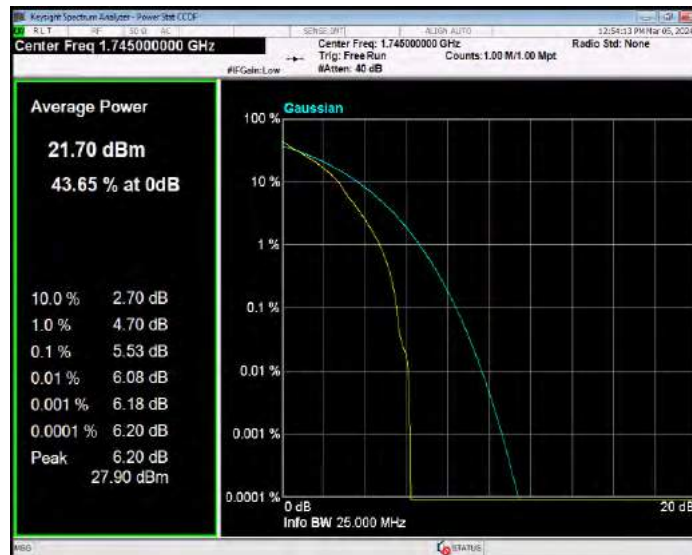
Band66 QPSK BW=5MHz Channel=132647 RB Size=1 Position=#0
