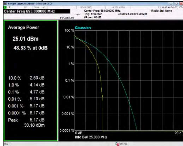
Band71 QPSK BW=15MHz Channel=133197 RB Size=1 Position=#0
