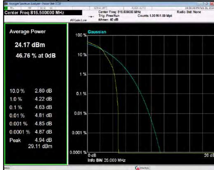
Band26(814-824) 16QAM BW=5MHz Channel=26740 RB Size=1 Position=#0
