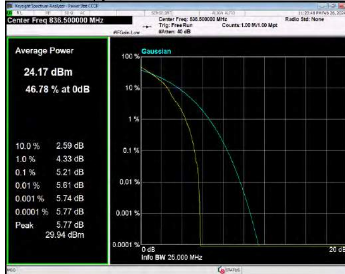
Band26(824-849) QPSK BW=3MHz Channel=27025 RB Size=1 Position=#0
