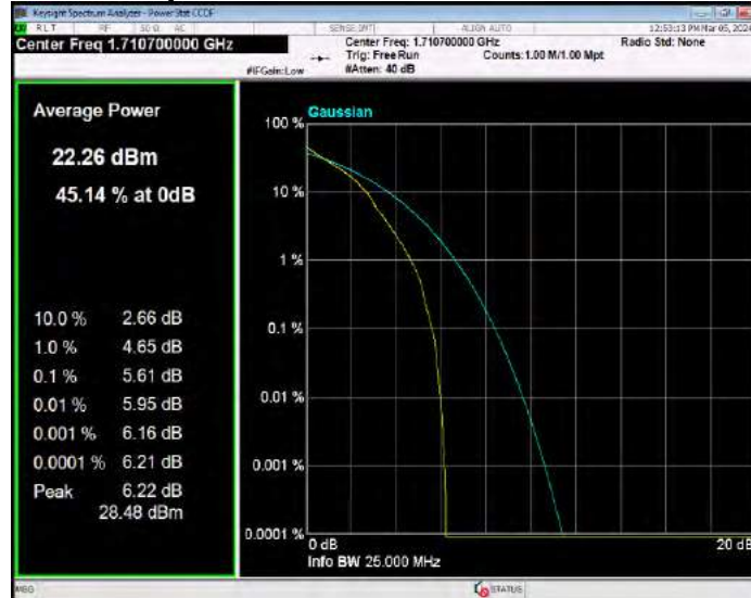
Band66 QPSK BW=1.4MHz Channel=132322 RB Size=1 Position=#0
