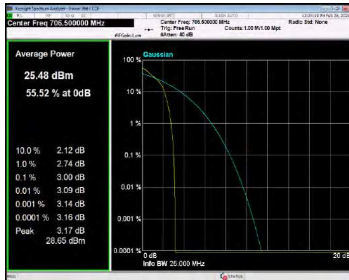
Band17 QPSK BW=5MHz Channel=23790 RB Size=1 Position=#0
