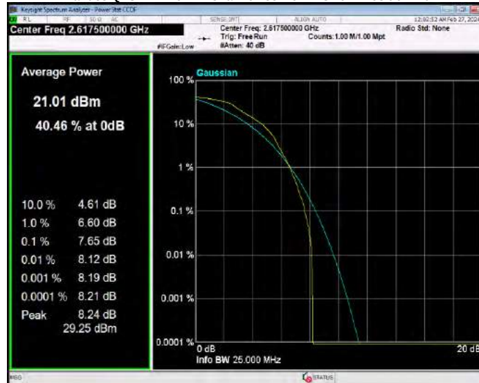
Band40(2305-2315) 16QAM BW=10MHz Channel=38750 RB Size=1 Position=#0
