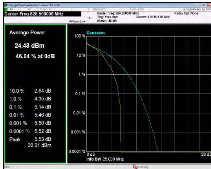
Band26(824-849) QPSK BW=5MHz Channel=26915 RB Size=1 Position=#0
