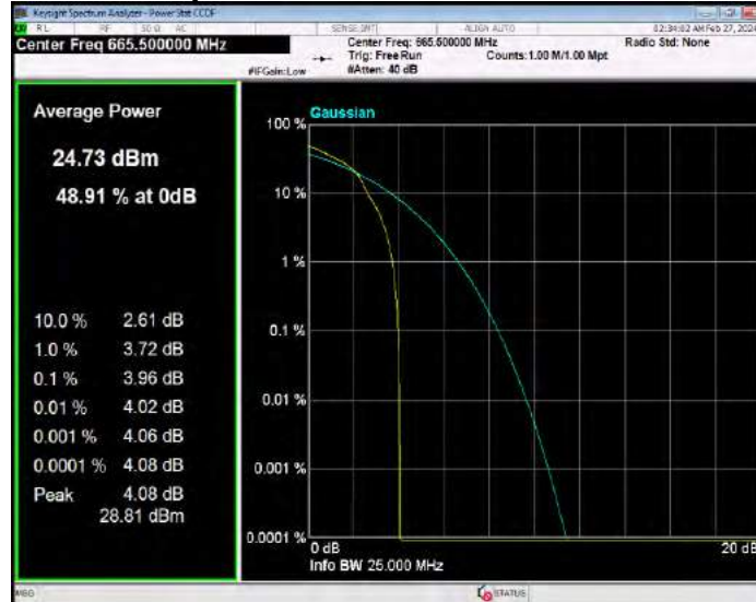
Band71 16QAM BW=5MHz Channel=133297 RB Size=1 Position=#0
