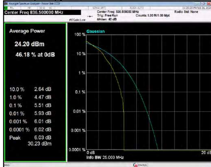
Band26(824-849) QPSK BW=1.4MHz Channel=27033 RB Size=1 Position=#0
