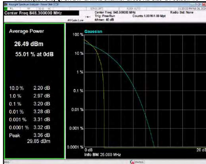
Band26(824-849) QPSK BW=10MHz Channel=26840 RB Size=1 Position=#0
