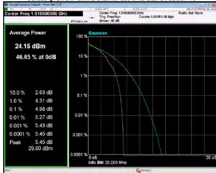
Band25 QPSK BW=15MHz Channel=26115 RB Size=1 Position=#0
