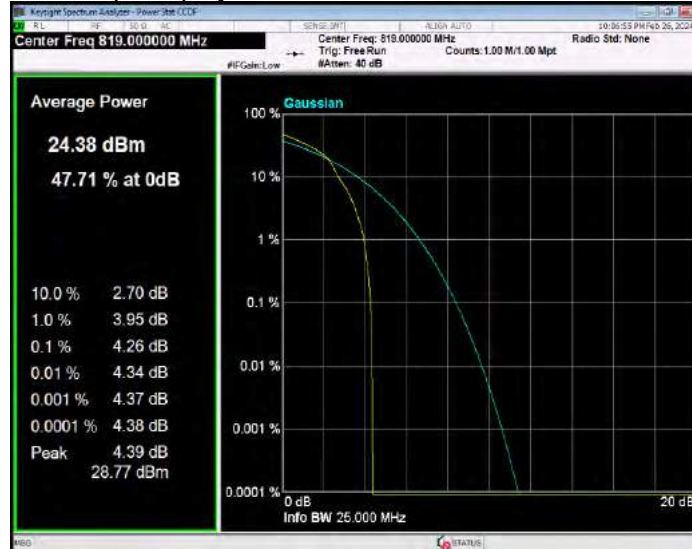
Band26(814-824) 16QAM BW=5MHz Channel=26765 RB Size=1 Position=#0
