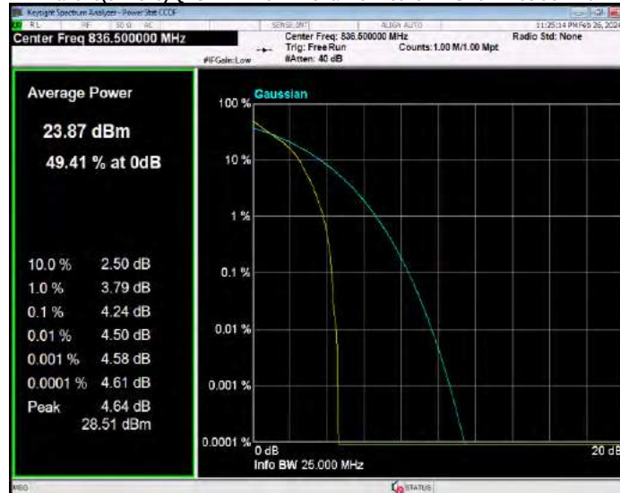
Band26(824-849) QPSK BW=15MHz Channel=26965 RB Size=1 Position=#0
