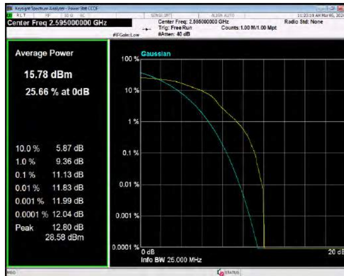
Band41(2535-2655) 16QAM BW=15MHz Channel=40640 RB Size=1 Position=#0
