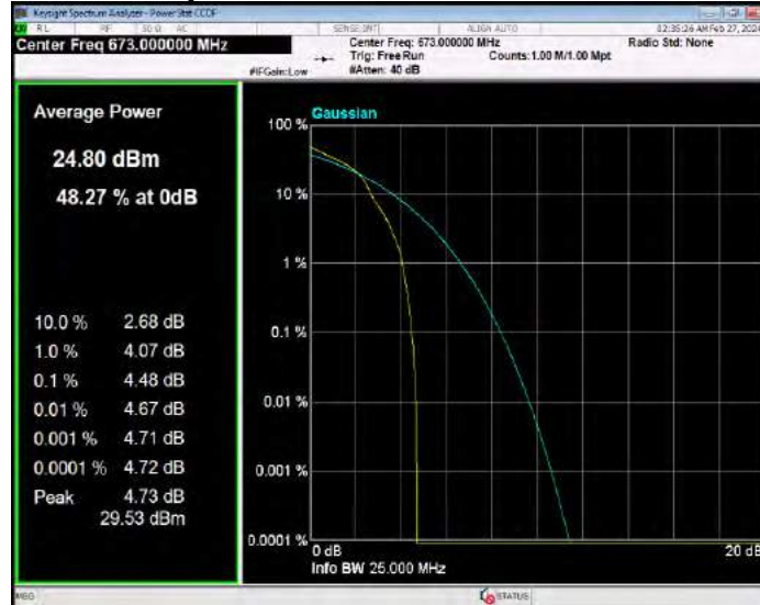
Band71 16QAM BW=20MHz Channel=133297 RB Size=1 Position=#0
