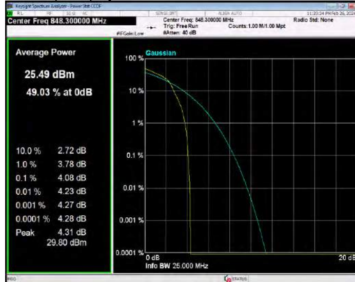
Band26(824-849) 16QAM BW=10MHz Channel=26840 RB Size=1 Position=#0
