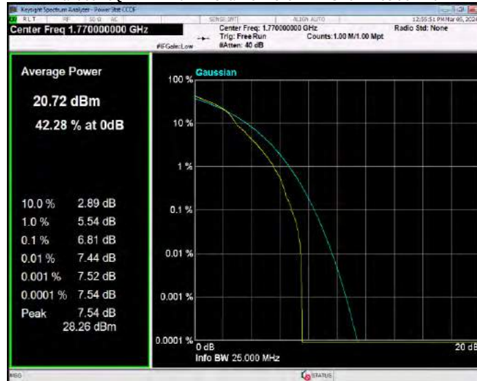
Band66 16QAM BW=3MHz Channel=131987 RB Size=1 Position=#0
