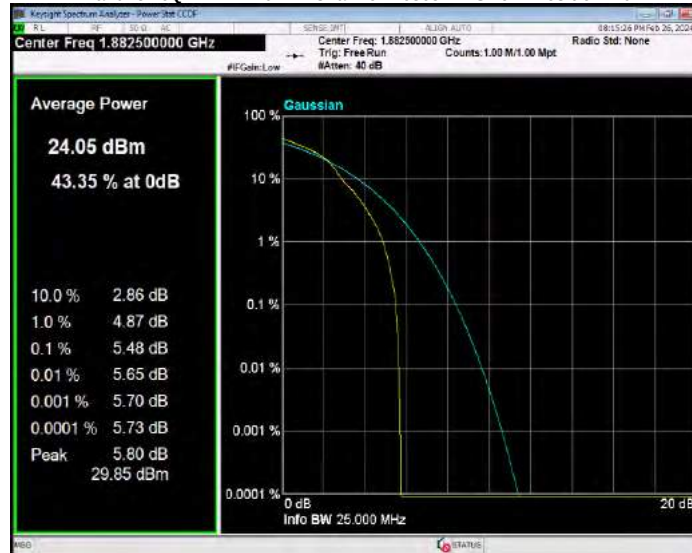
Band25 16QAM BW=20MHz Channel=26390 RB Size=1 Position=#0
