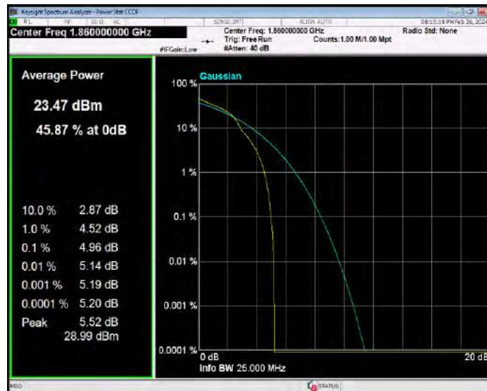
Band25 16QAM BW=20MHz Channel=26365 RB Size=1 Position=#0
