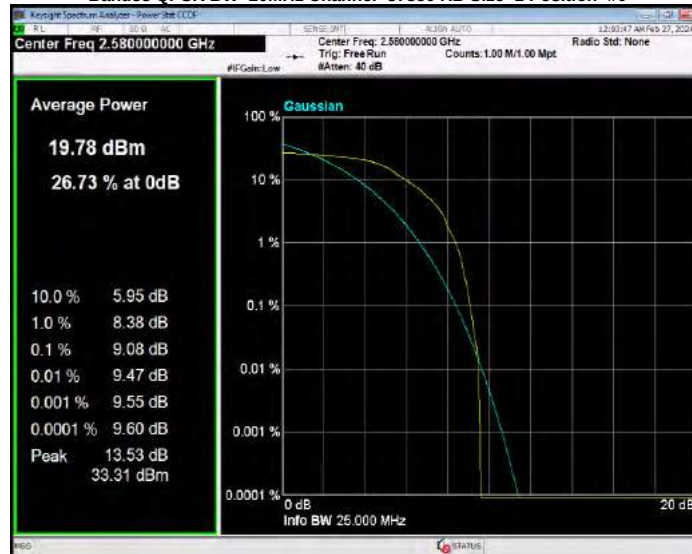
Band38 QPSK BW=20MHz Channel=38000 RB Size=1 Position=#0
