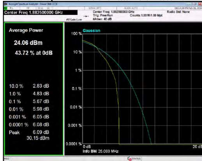
Band25 16QAM BW=10MHz Channel=26640 RB Size=1 Position=#0
