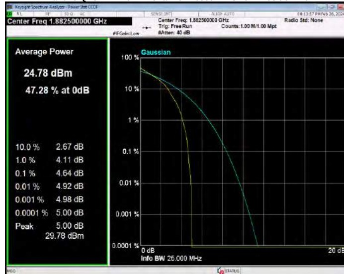
Band25 QPSK BW=5MHz Channel=26665 RB Size=1 Position=#0
