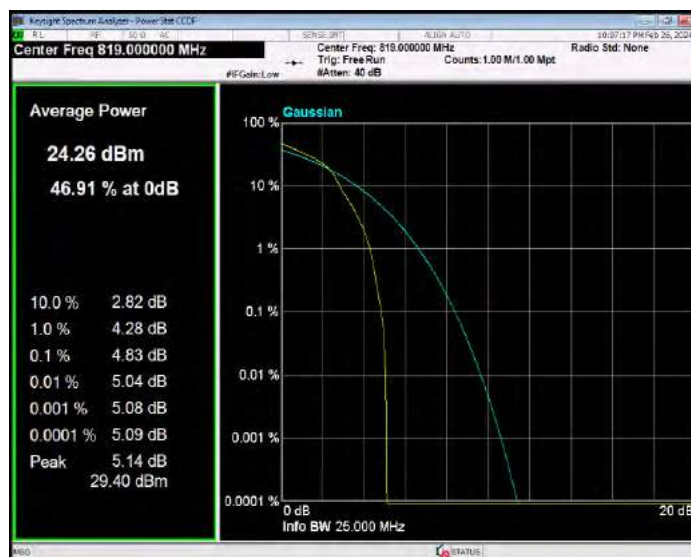
Band26(814-824) 16QAM BW=3MHz Channel=26705 RB Size=1 Position=#0
