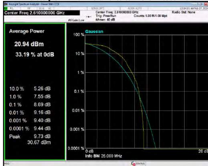
Band38 QPSK BW=5MHz Channel=37775 RB Size=1 Position=#0
