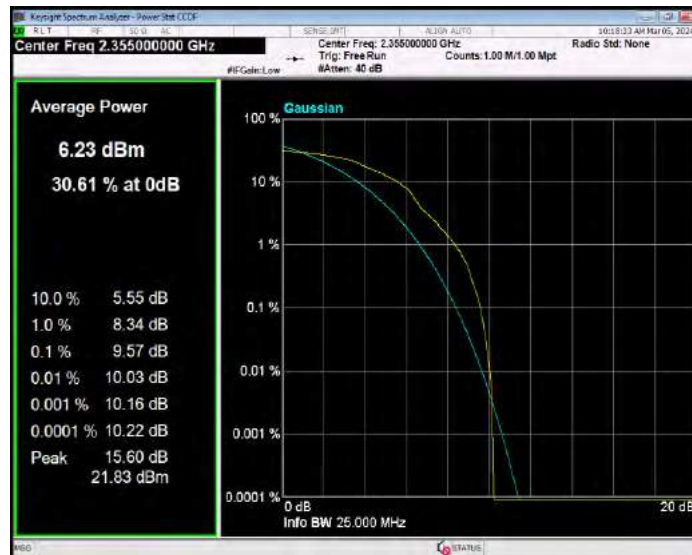
Band40(2350-2360) 16QAM BW=5MHz Channel=39225 RB Size=1 Position=#0
