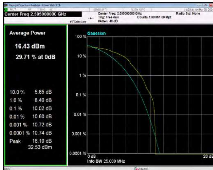
Band41(2535-2655) QPSK BW=10MHz Channel=40640 RB Size=1 Position=#0
