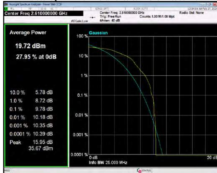
Band38 16QAM BW=5MHz Channel=37775 RB Size=1 Position=#0
