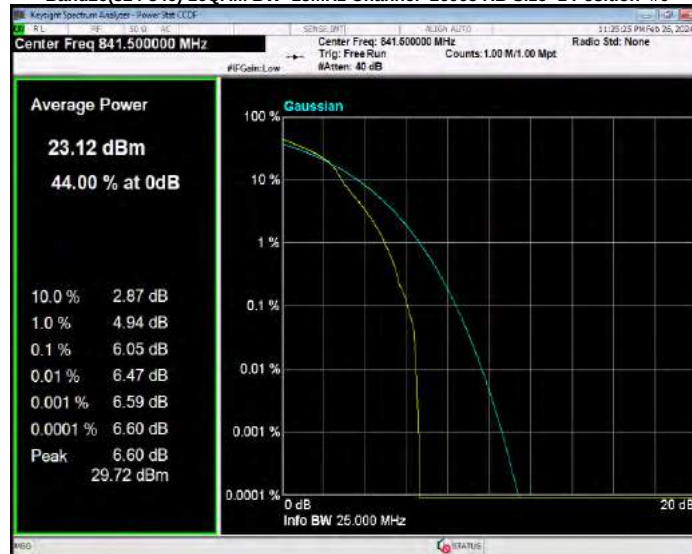
Band26(824-849) 16QAM BW=3MHz Channel=26805 RB Size=1 Position=#0
