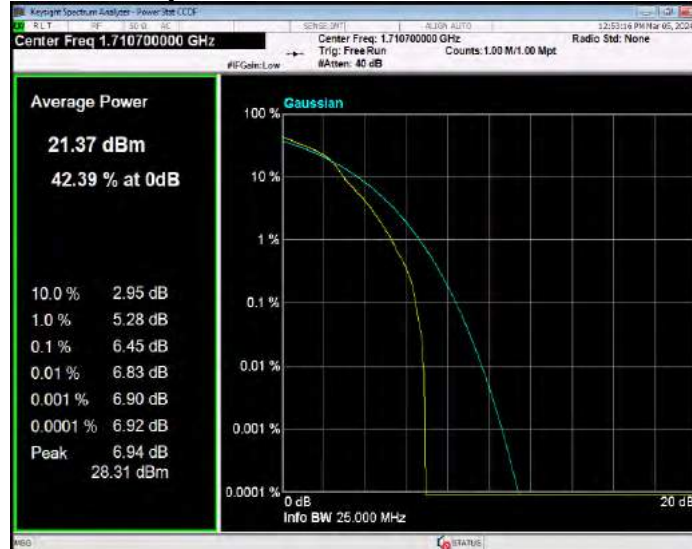
Band66 16QAM BW=1.4MHz Channel=132322 RB Size=1 Position=#0
