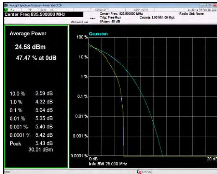
Band26(824-849) QPSK BW=3MHz Channel=26915 RB Size=1 Position=#0
