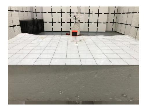
Set-up for Radiated Spurious Emission, Above 1GHz
