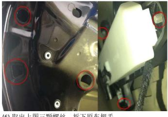
(6).取出上图三颗螺丝,拆下原车把手 Take out the three screws in the picture above and remove the original handlebar
