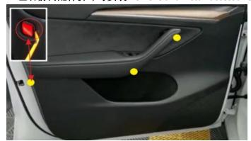
(1).卸下上图三处螺丝 Remove the three screws in the picture above
