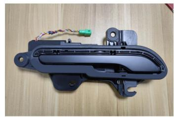
(10).将第二代把手安装到车上,用原车螺丝固定 Install the second generation handle on the car and secure it with the original car screws
