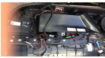
(4).把与盖板相连的插线拔下 拿下盖板 Remove and remove the plug wire connected to the cover plate
