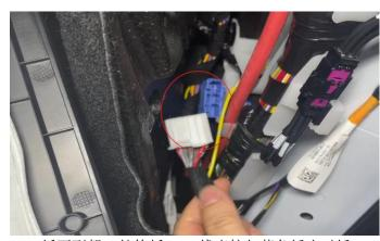
(2) 拆下副驾 A 柱饰板 CAN 线直接与蓝色插座对插 Remove co-pilot's A-pillar trim panel and plug the CAN cable directly into the blue socket
