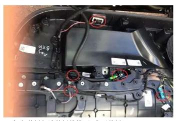
(4).把与盖板相连的插线拔下 拿下盖板 Remove the plug wire connected to the cover plate and remove the cover plate
