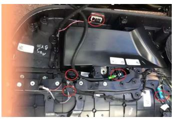
(4).把与盖板相连的插线拔下 拿下盖板 Remove the plug wire connected to the cover plate and remove the cover plate
