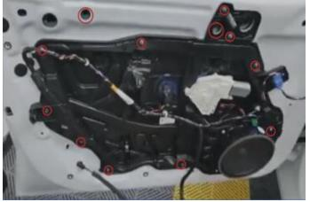
(5).拔掉所有插头取下标记的所有螺丝拿下饰板 Unplug all plugs, remove all marked screws and remove the trim plate
