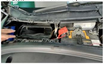
(1) 在前盖电池取电,左边找孔穿线至副驾驶 Connect the cable to the battery in the front cover, find a hole on the left side and thread the cable to the co-pilot
