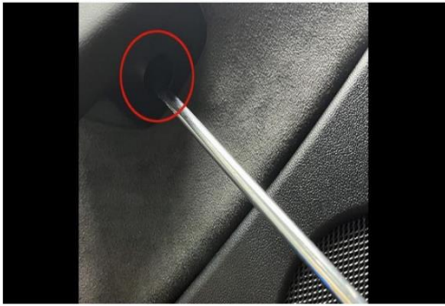
7. Remove the setscrew of rear door panel
