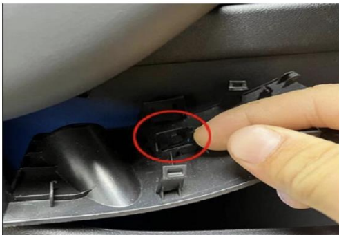
9. Install the door storage box light on the original reserved position
