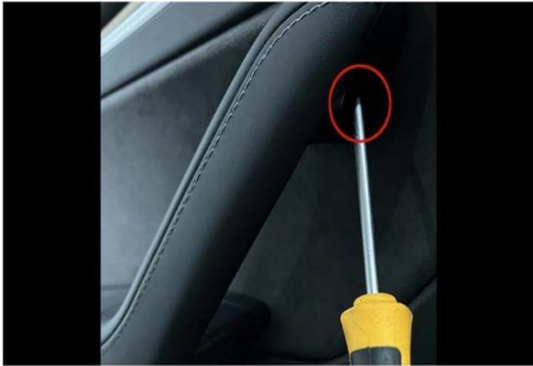
1. Remove the door panel setscrews
