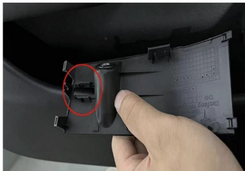
5. Install the door storage box light on the original reserved position
