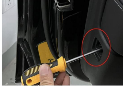
1. Remove the door panel setscrews
