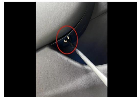
6. Remove the setscrew of rear door panel
