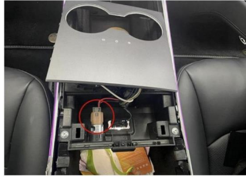
4. Main module power cable connect with cigarette lighter
