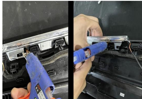
4. Use holt melt glue to fix the light strips
