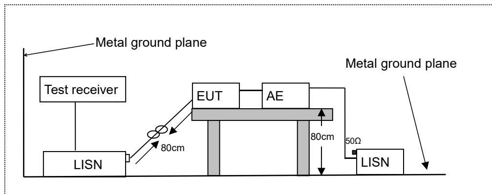
LISN: Line Impedance Stabilization Network
