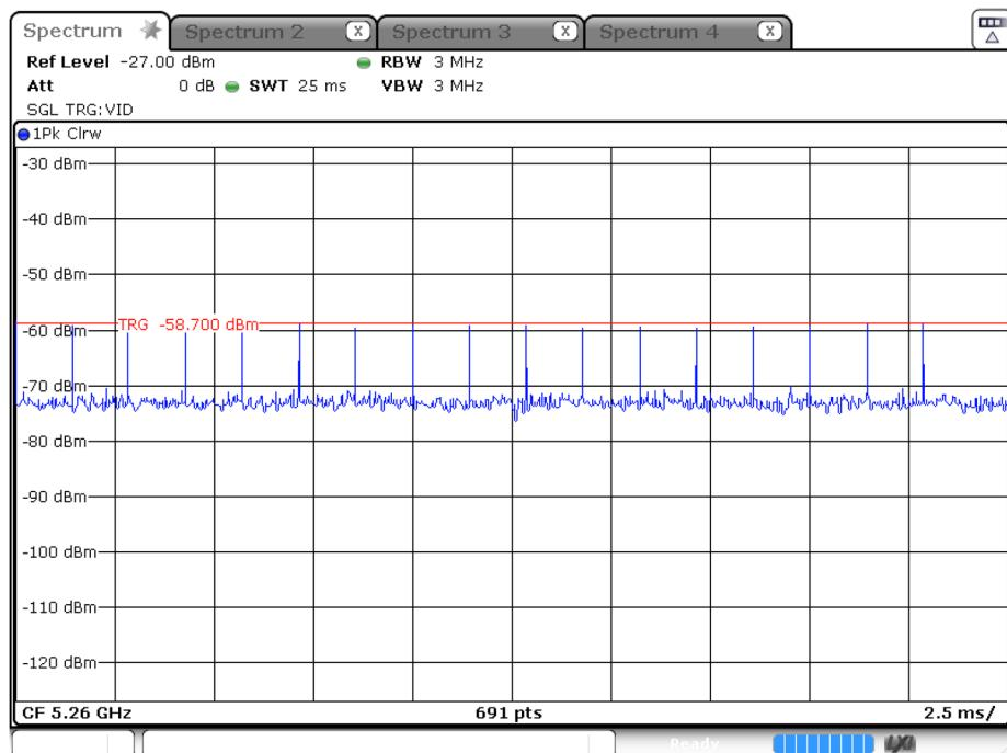
**Radar Type 1 test A Calibration Plot (5260MHz)**
