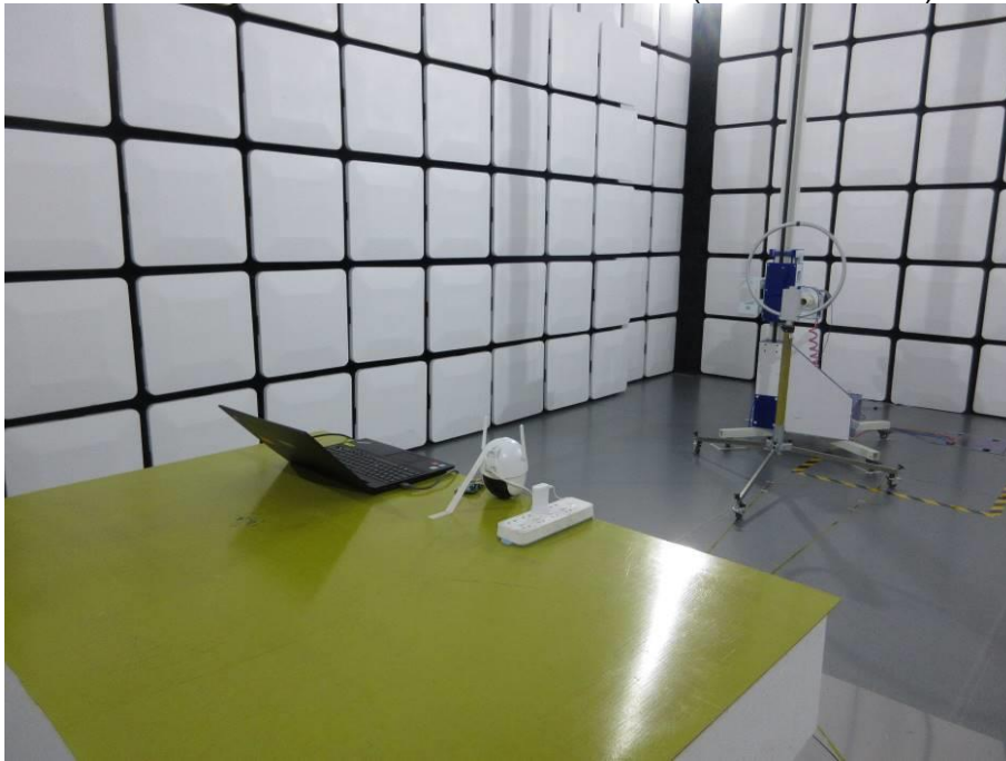
RADIATED RF MEASUREMENT SETUP (9kHz ~ 30 MHz)
