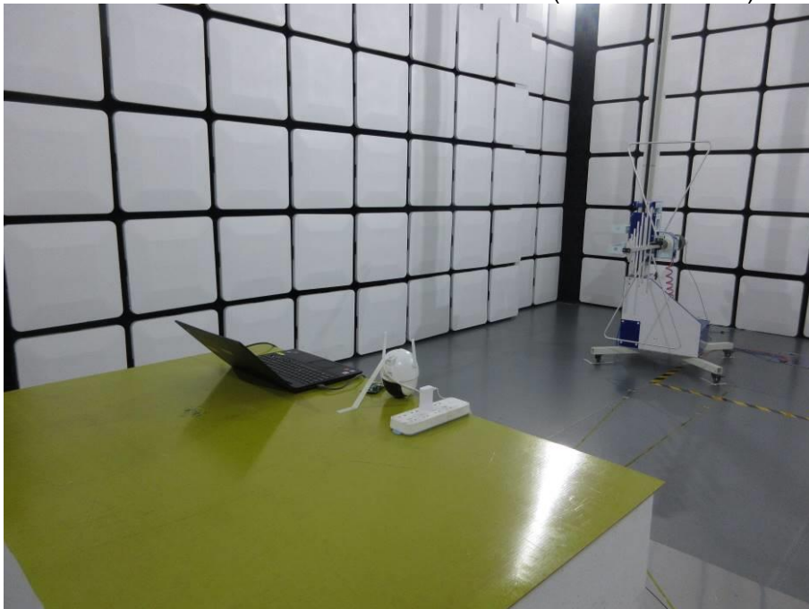
RADIATED RF MEASUREMENT SETUP (30MHz ~ 1 GHz)
