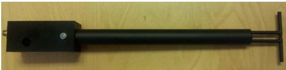
Figure 1 – MVG COMOSAR Validation Dipole
