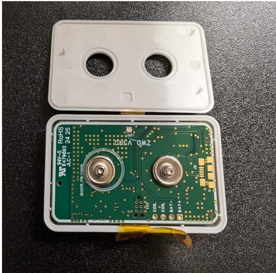
Photograph 4 – View of the PCB Mounting in the Enclosure
