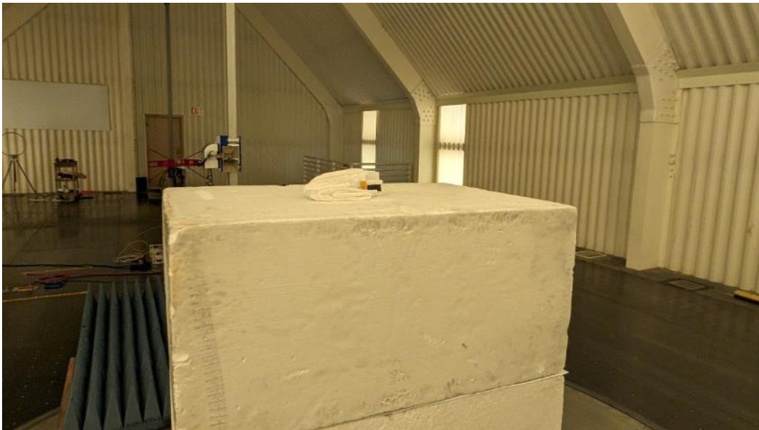
Photograph 2: Back View Radiated Emissions Worst-Case Configuration “Standing on Short Edge”
