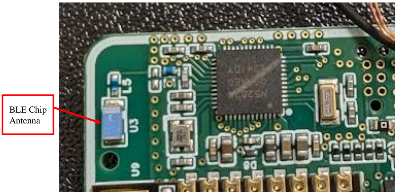
Photograph 19: Close-up View of the RF Circuitry
