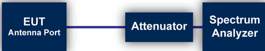
Figure 2: Direct Connection at the Antenna Port Test
