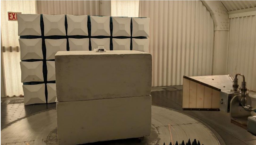
Photograph 1: Front View Radiated Emissions Worst-Case Configuration “Standing on Short Edge”
