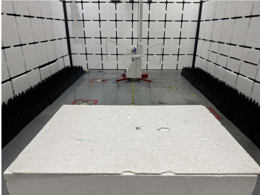
Radiated spurious emission Test Setup-1(Below 1GHz)
